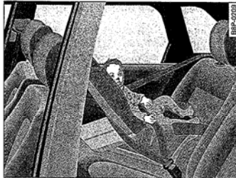
Fig. 174 Rearward-facing infant seat, properly installed on the rear seat
