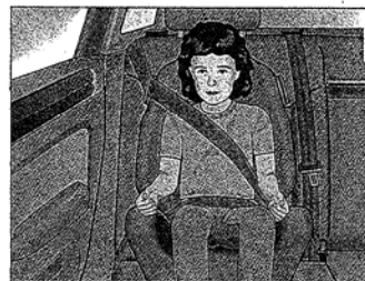
Fig. 176 Rear seat: child properly restrained in a booster seat
