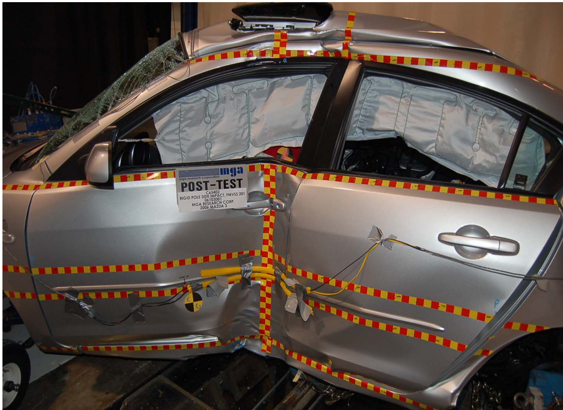
Post-Test Impact Zone Close-up View
