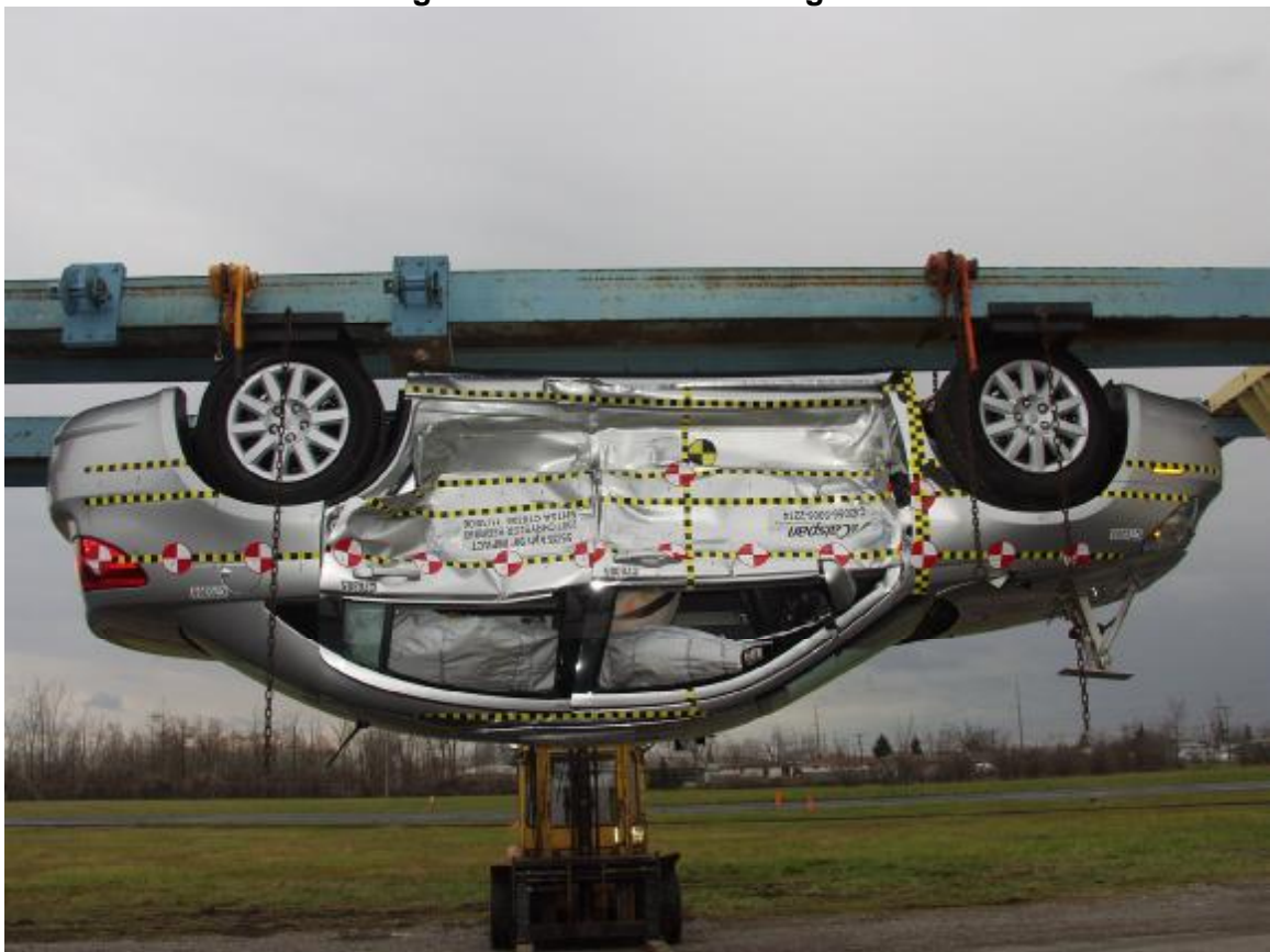
Figure A-52: Rollover 180 Degrees
