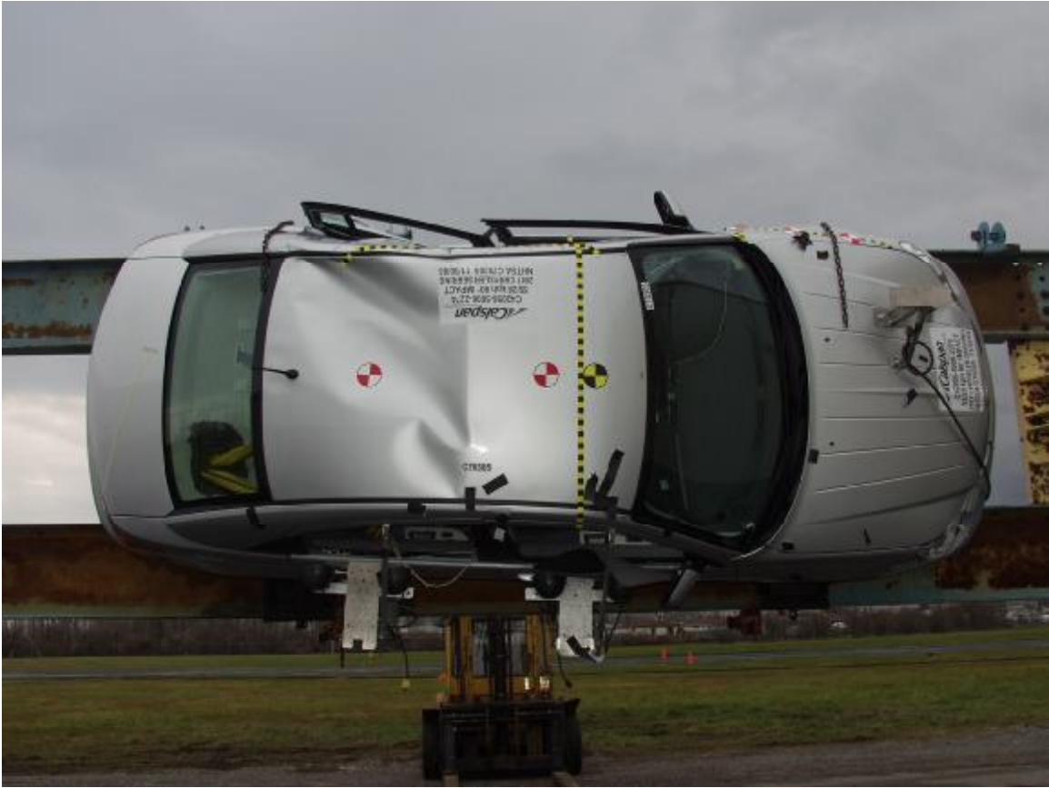
Figure A-53: Rollover 270 Degrees
