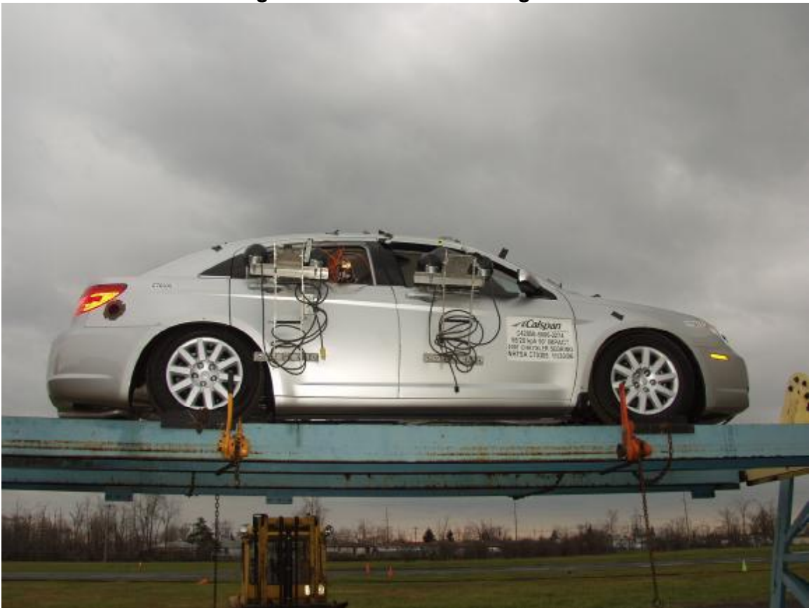
Figure A-54: Rollover 360 Degrees
