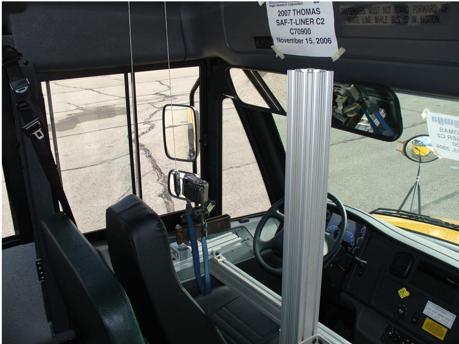
Field of View Instrument Setup
