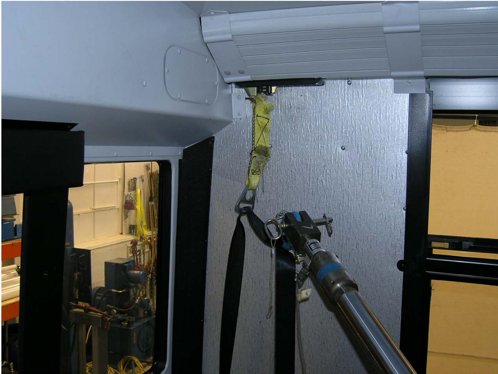
Post-Test of Wheelchair Anchorage W8.5 Upper Torso Type D Load Test
