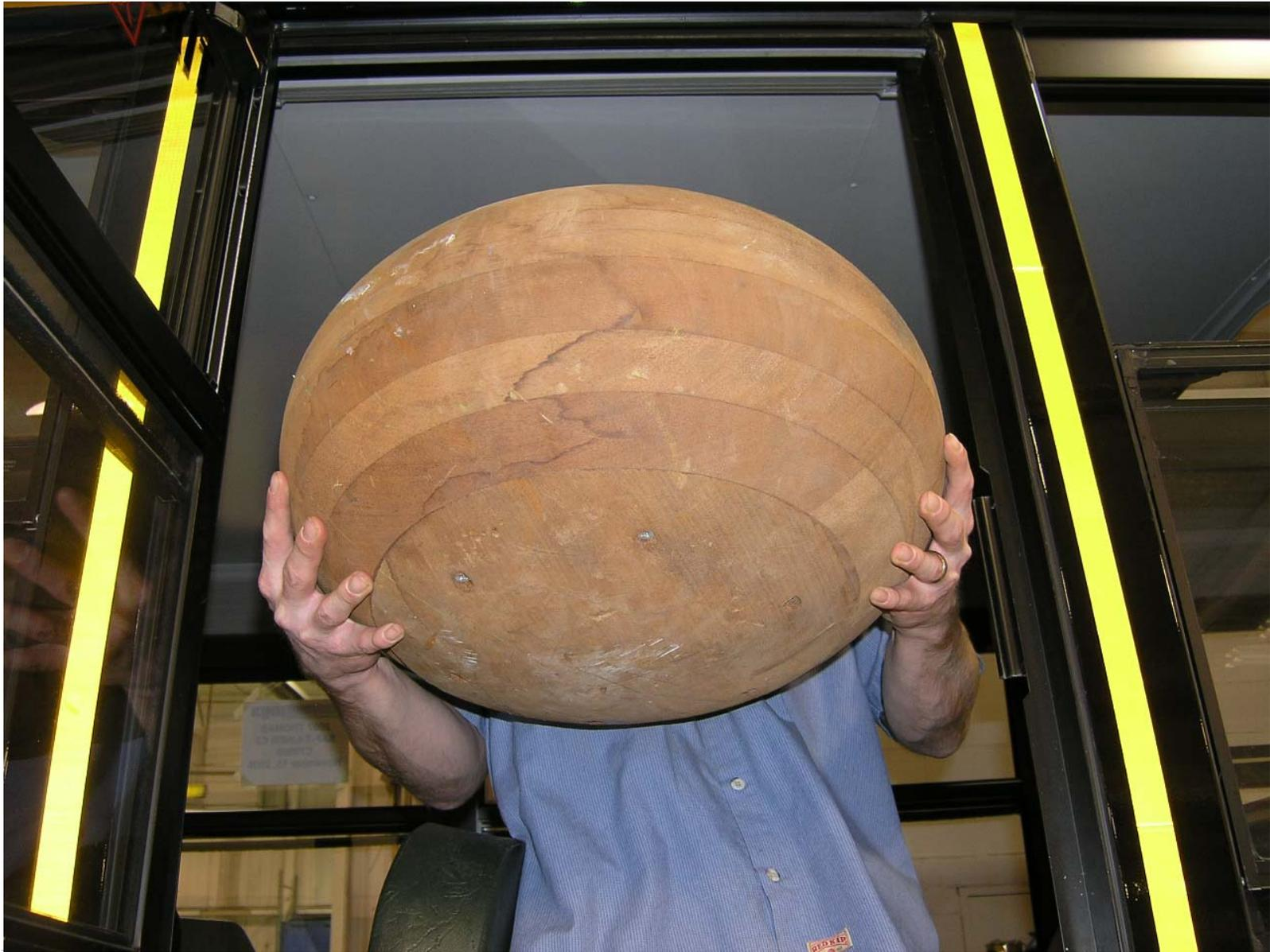
Left Side Emergency Exit Ellipsoid Clearance
