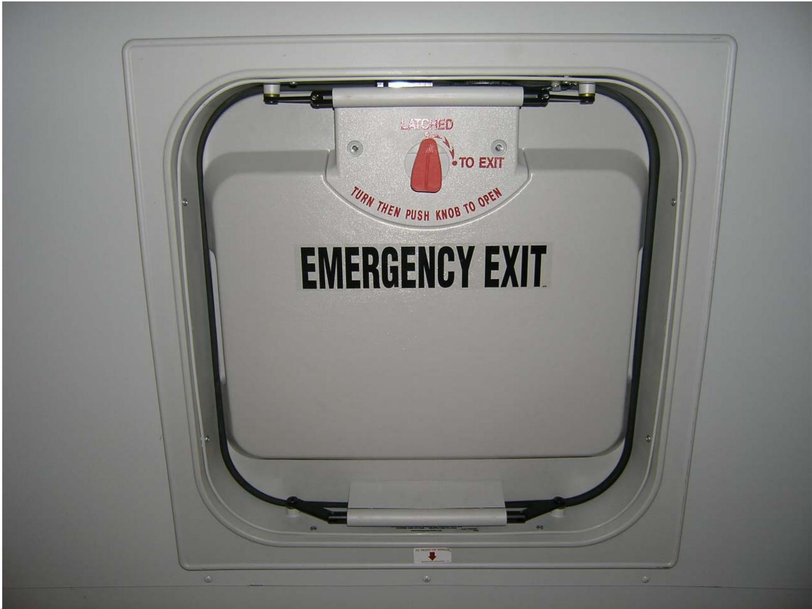
Roof Hatch Emergency Exit (Inside View)
