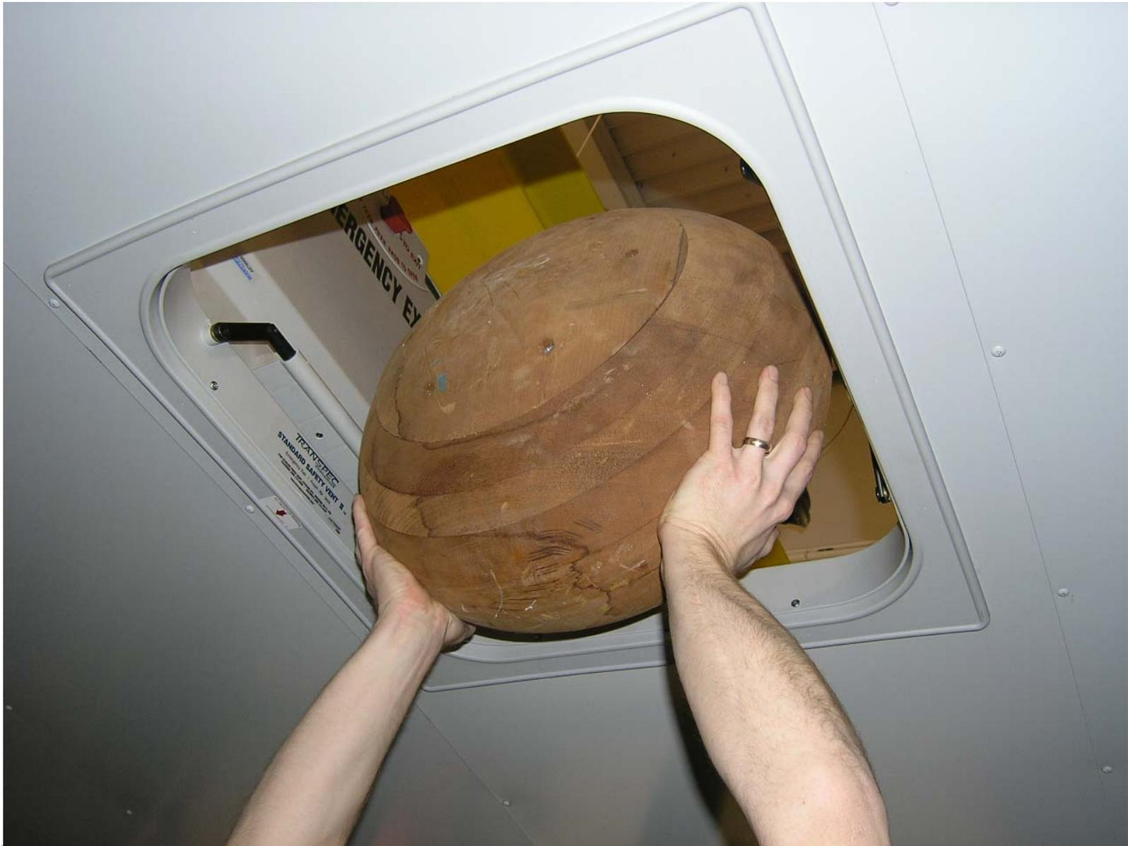
Roof Hatch Emergency Exit Ellipsoid Clearance
