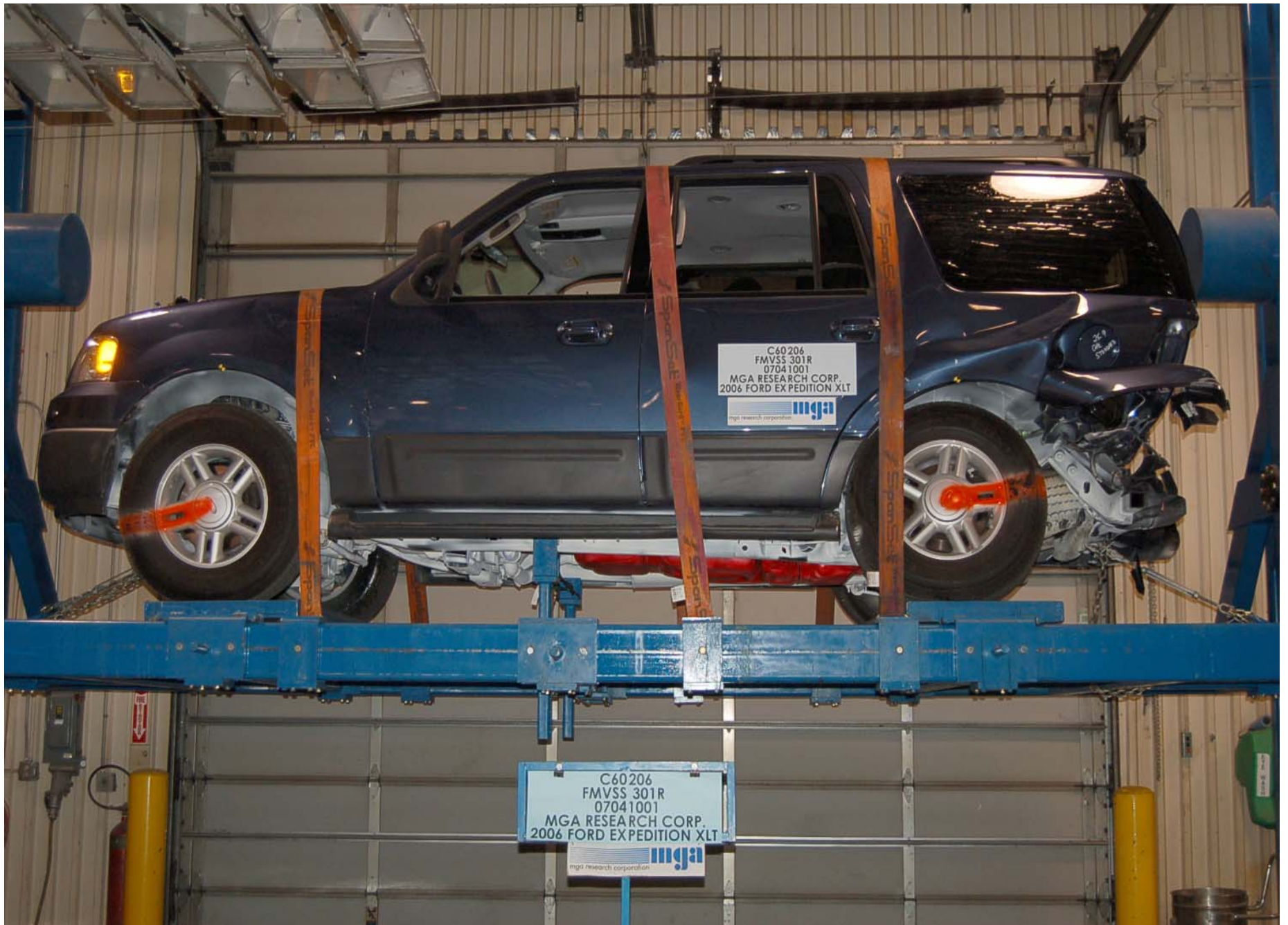
Static Rollover at 360 Degrees
