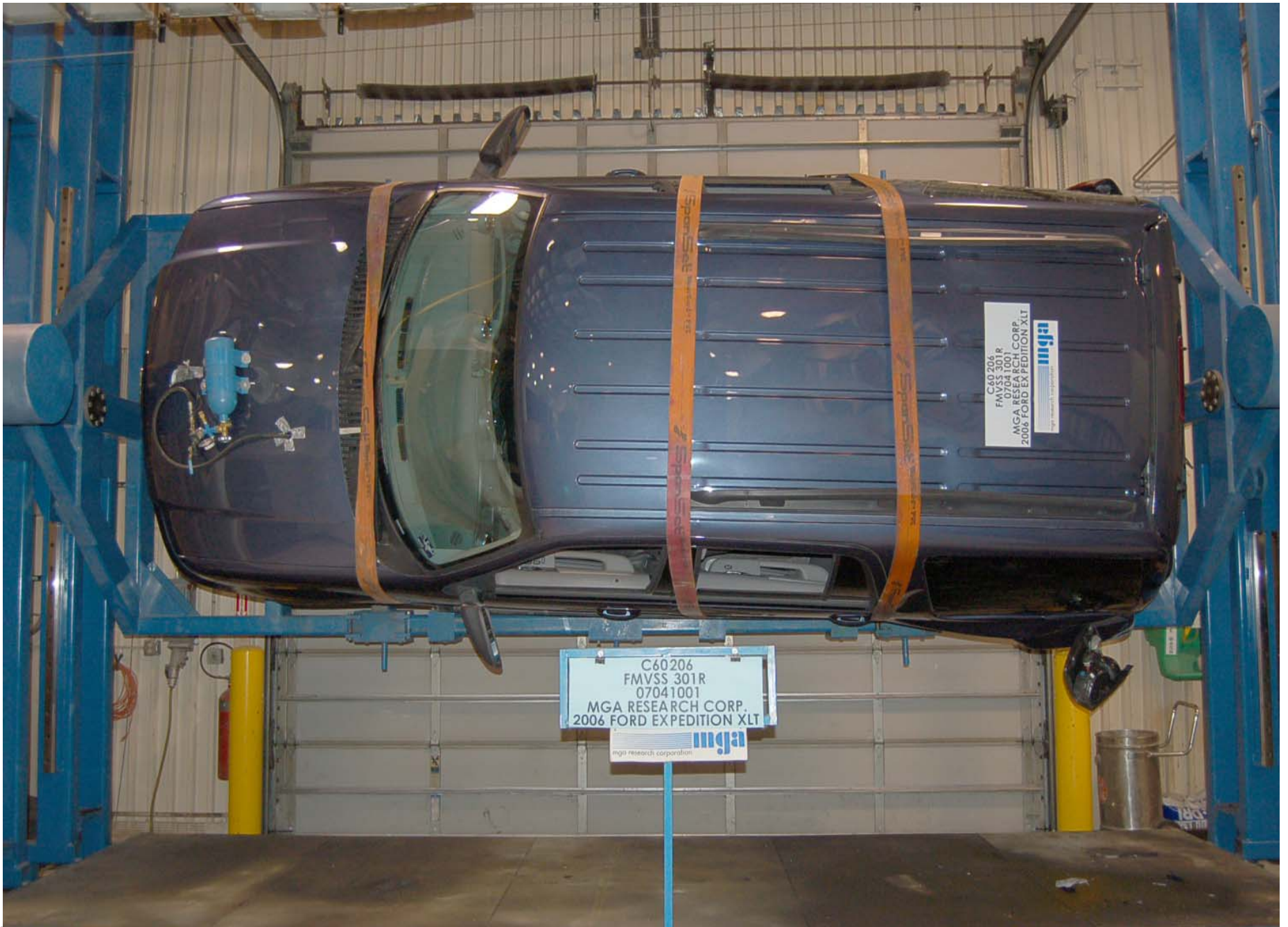
Static Rollover at 90 Degrees
