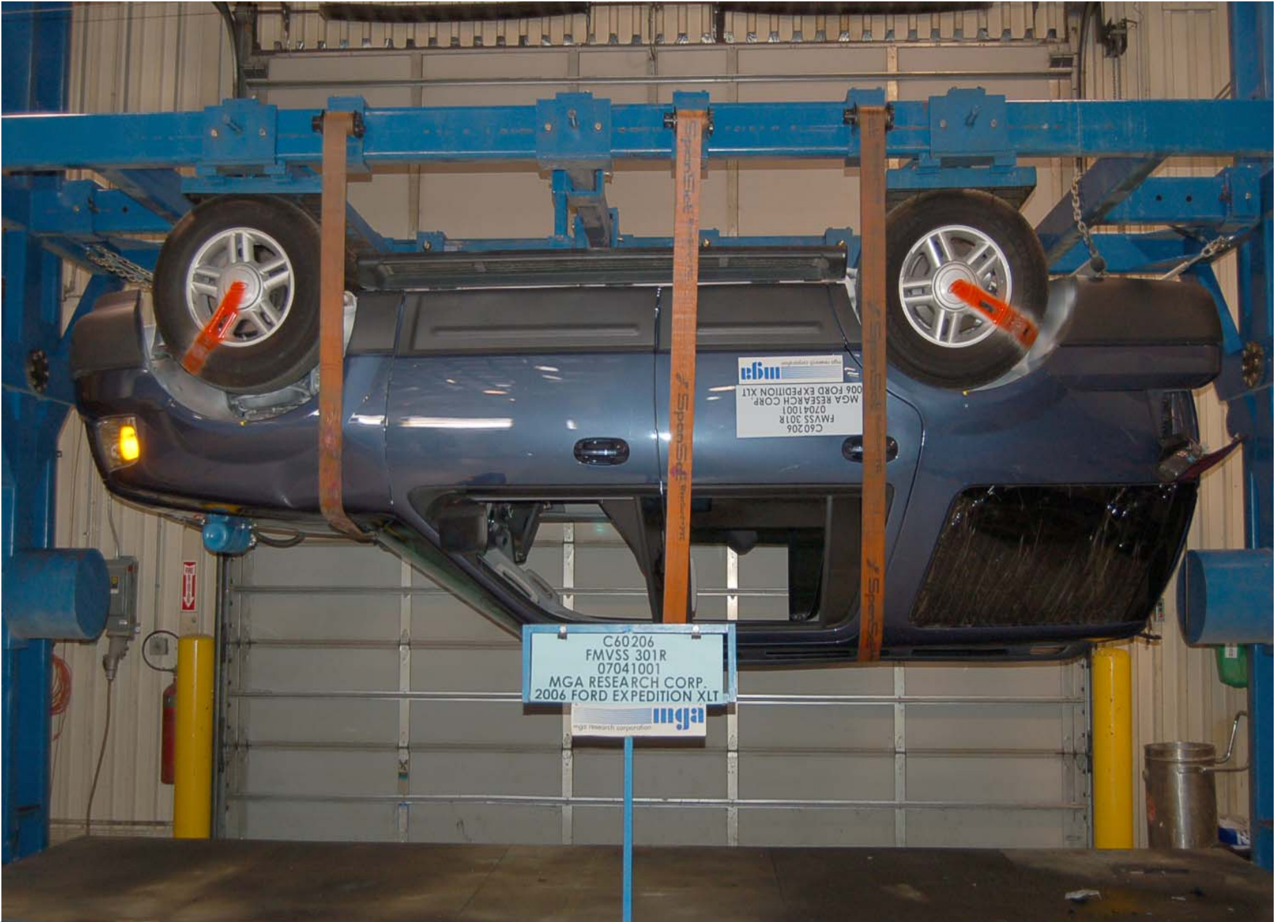
Static Rollover at 180 Degrees
