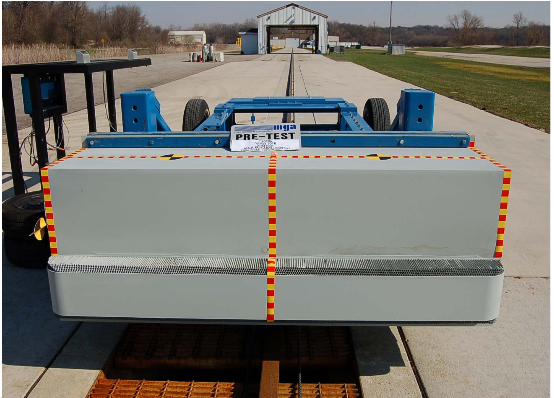
Pre-Test Front View of MDB
