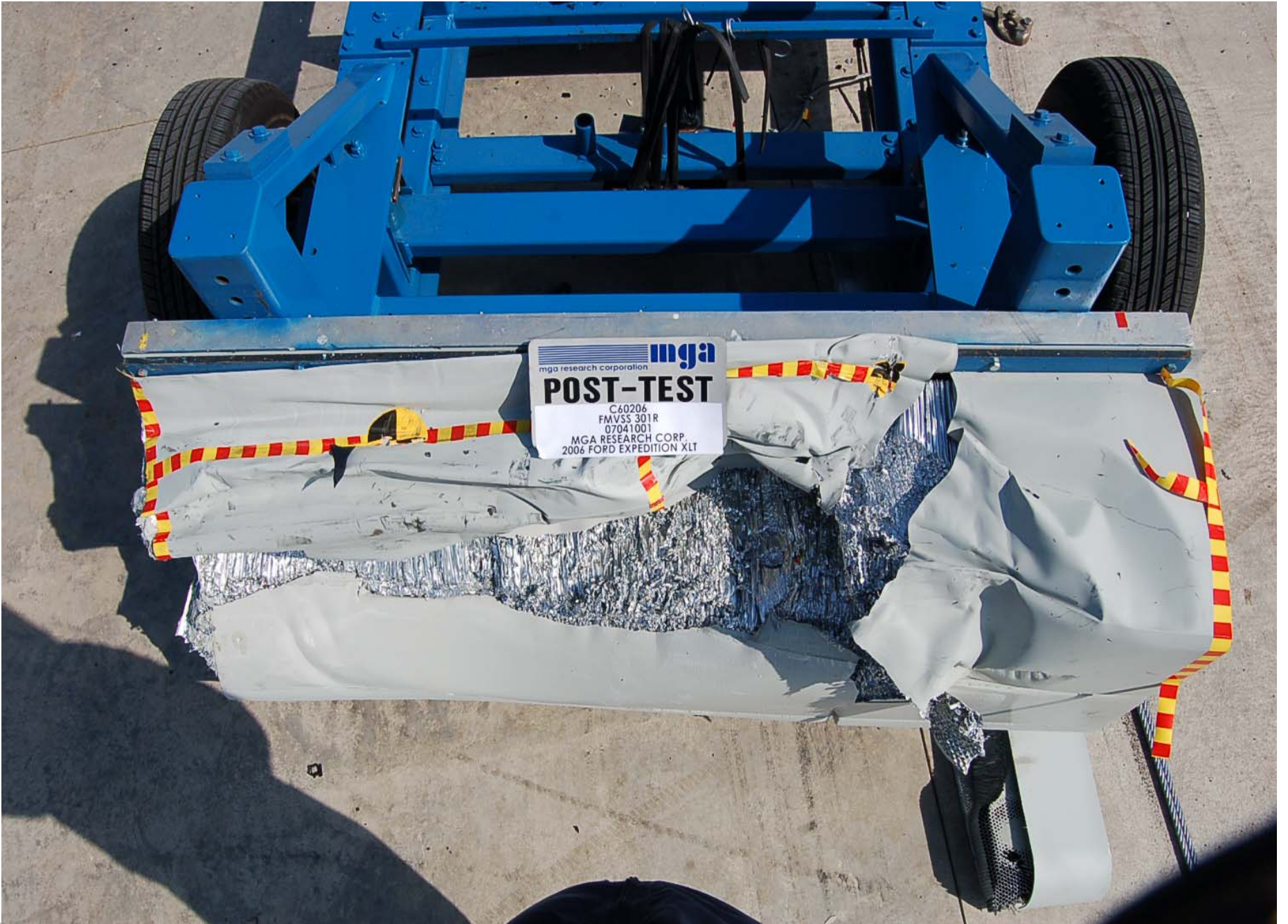
Post-Test Top View of MDB
