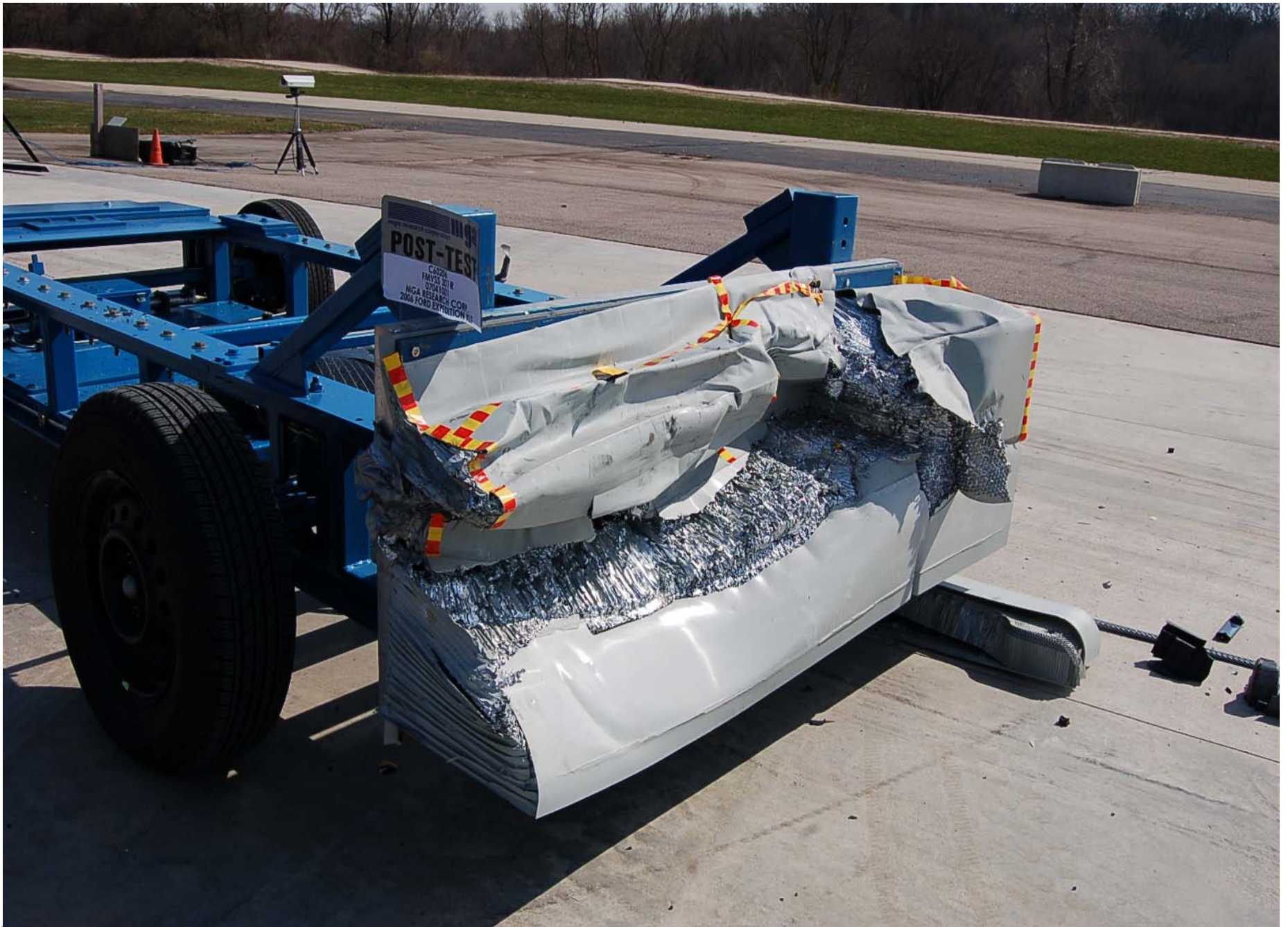
Post-Test ¾ Right Side View of MDB
