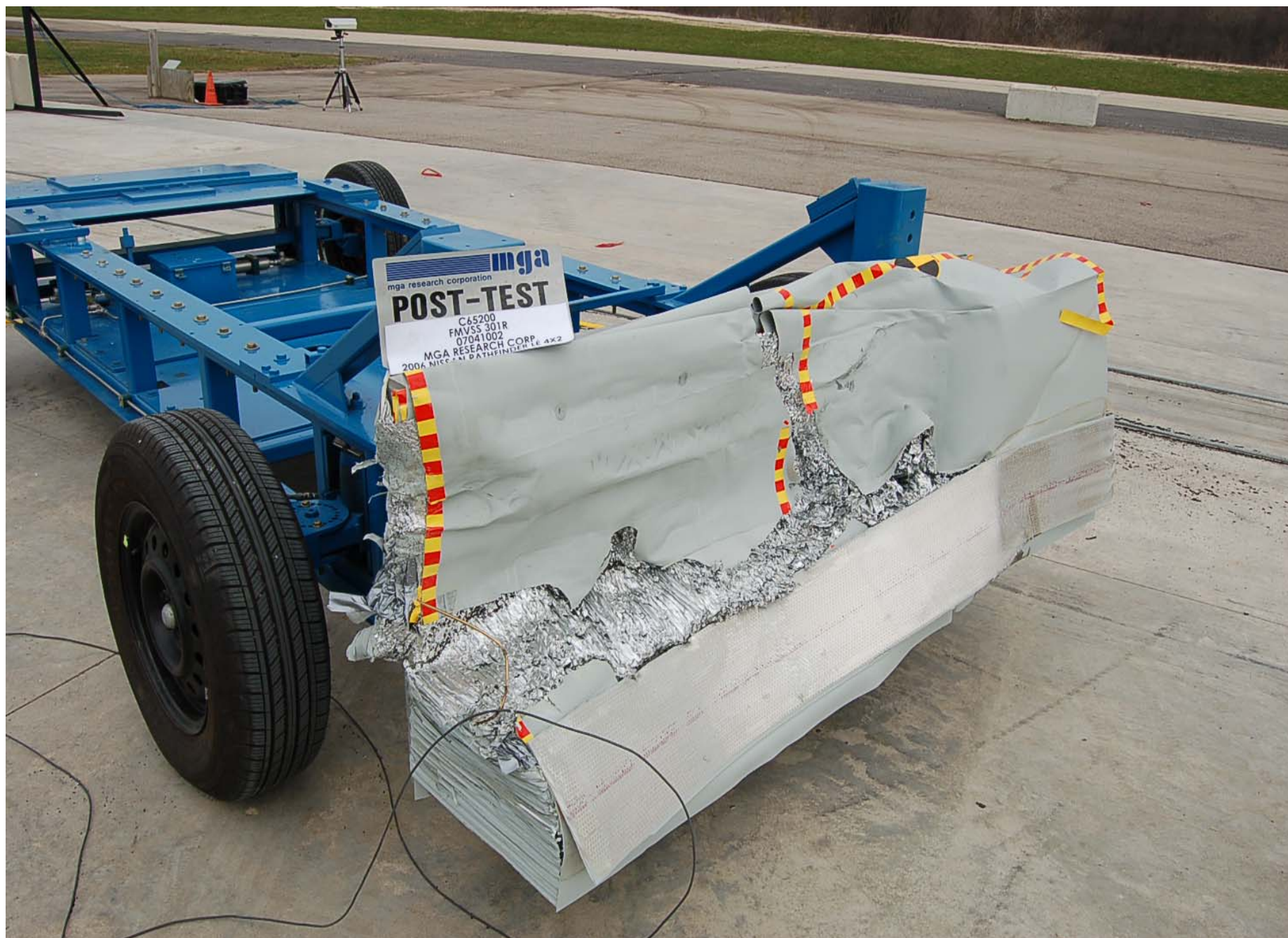
Post-Test ¾ Right Side View of MDB
