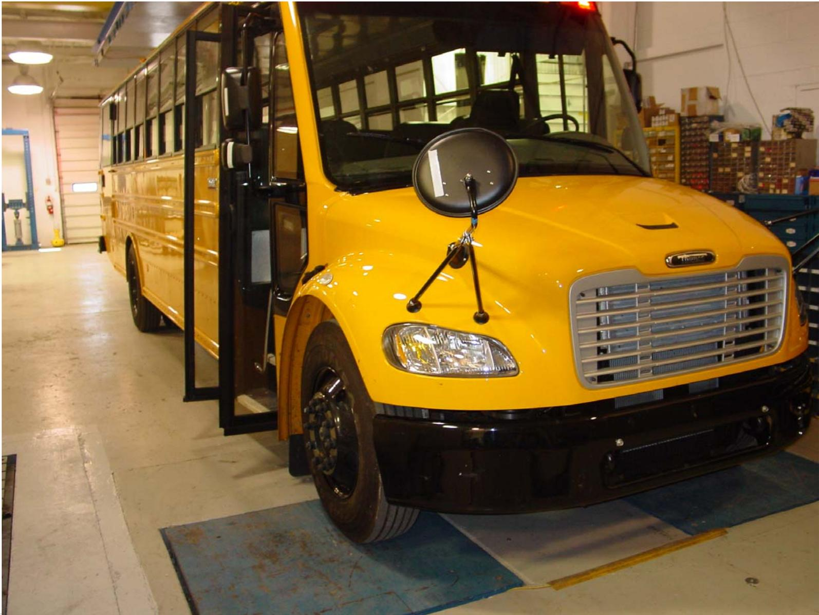
Vehicle on Scales Doing Measurement of Front Axle Loads
