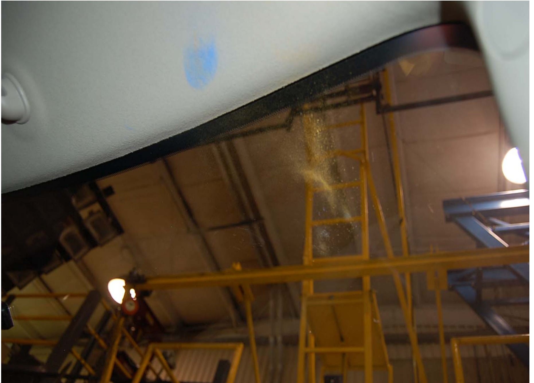
Post-Test Passenger Dummy Head Contact (windshield/header)
