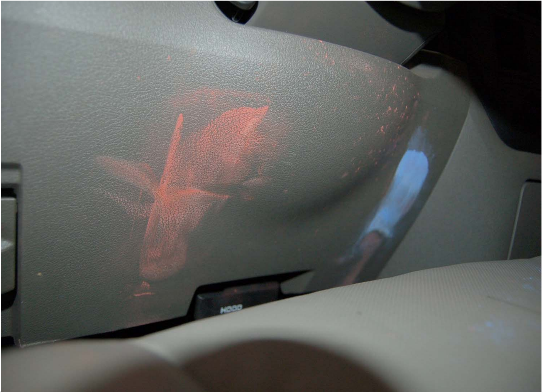
Post-Test Driver Dummy Knee Contact
