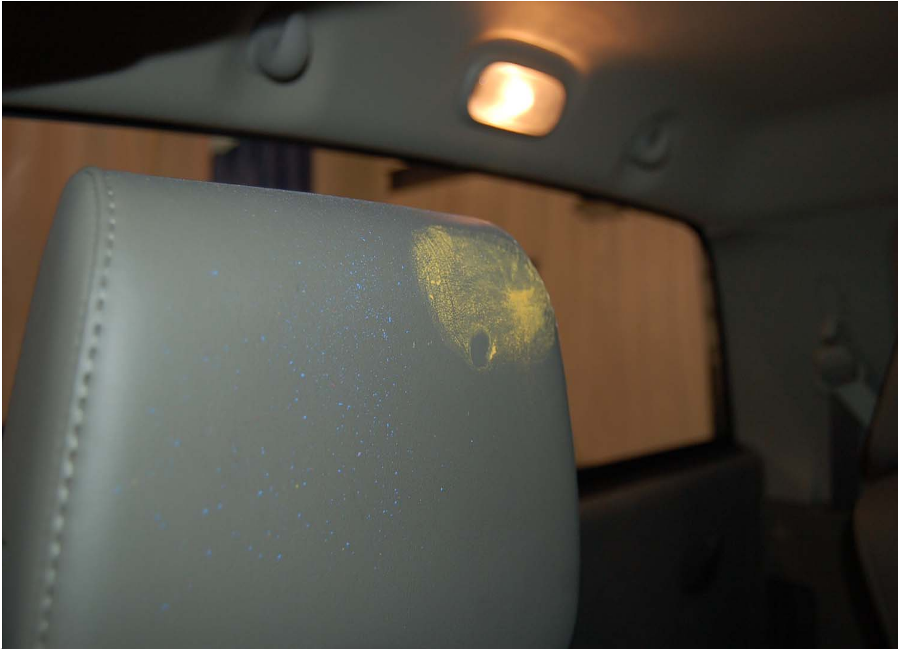
Post-Test Passenger Dummy Head Contact (head rest)
