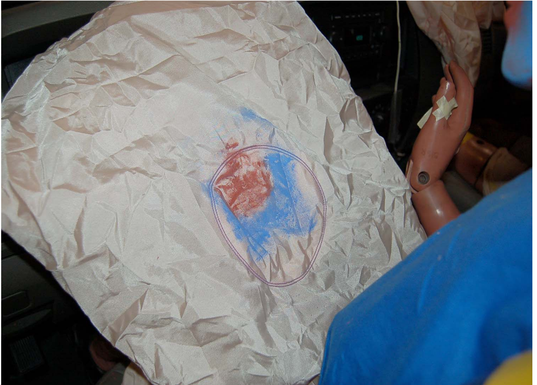
Post-Test Driver Dummy Airbag Contact
