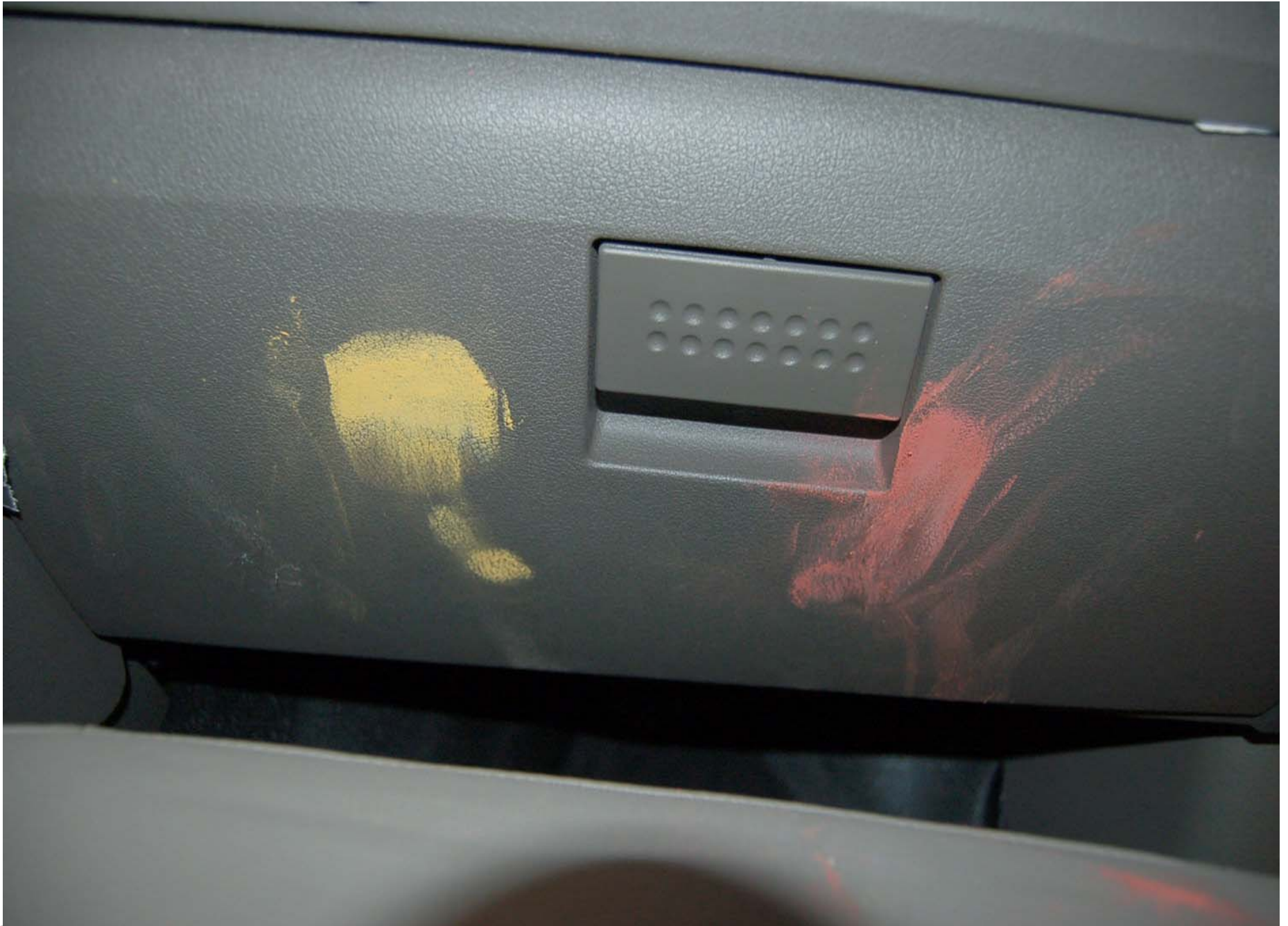
Post-Test Passenger Dummy Knee Contact
