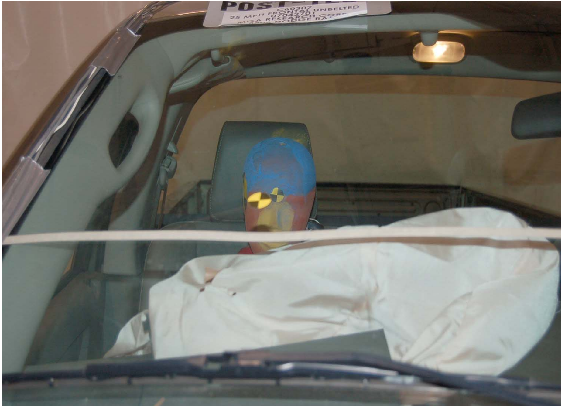
Post-Test Passenger Dummy Front View (head position)
