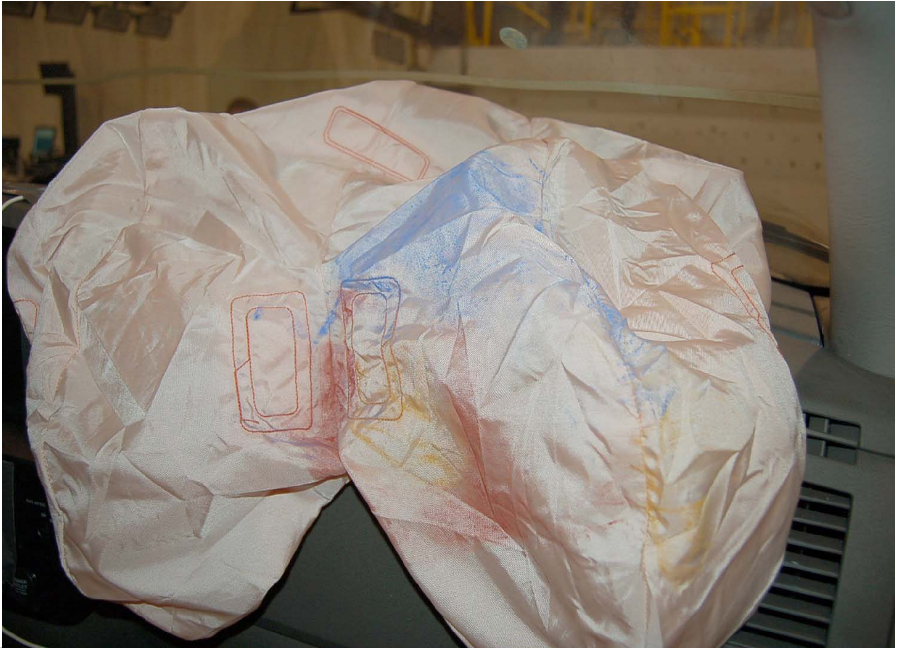
Post-Test Passenger Dummy Airbag Contact
