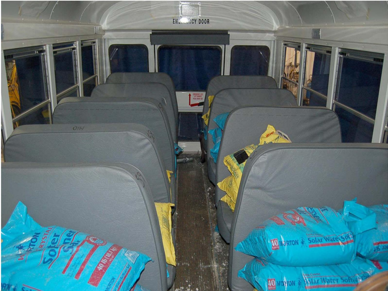
Pre-Test View of Ballast Weight View 1
