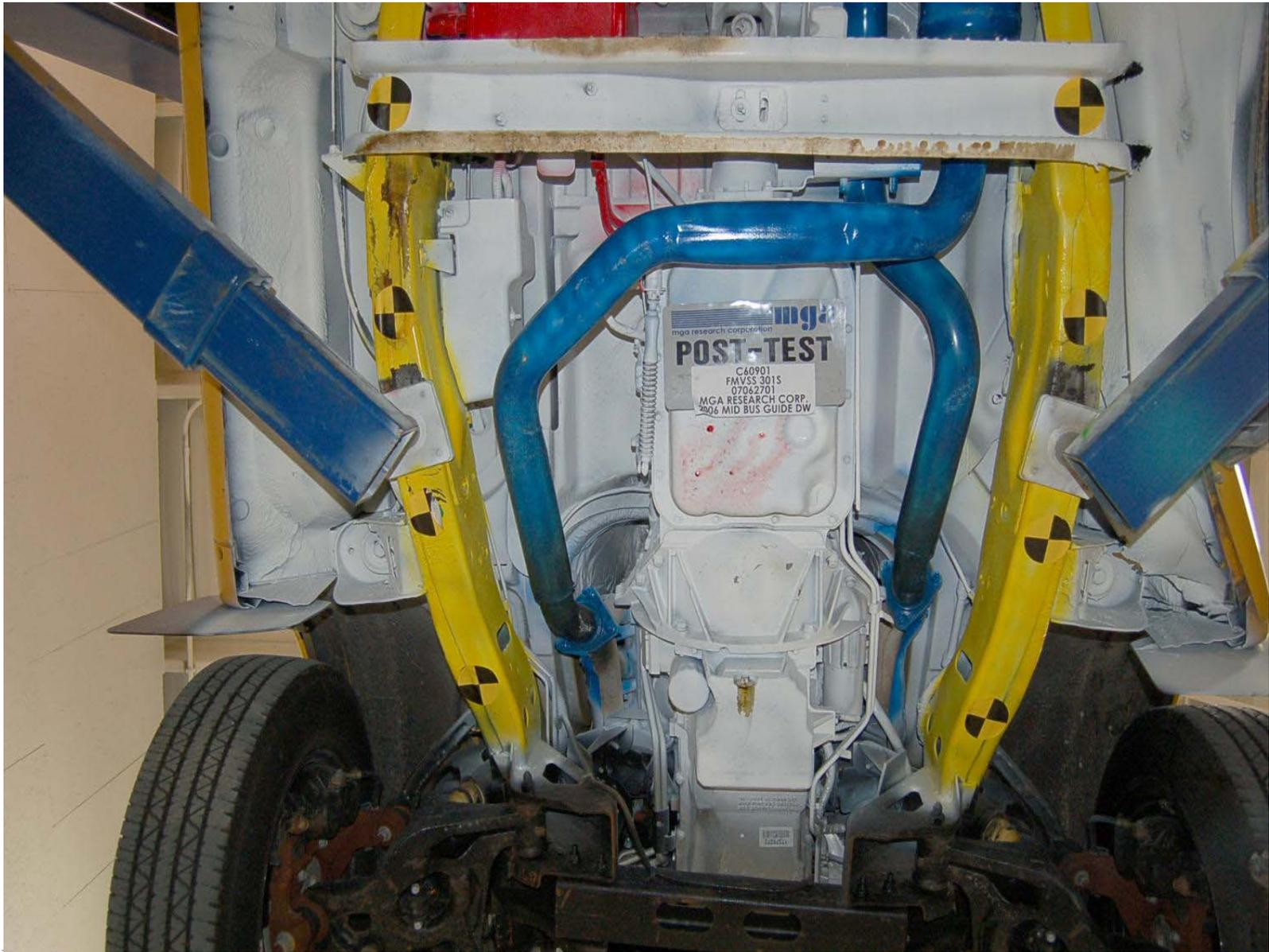
Post-Test Damage Underbody View 2
