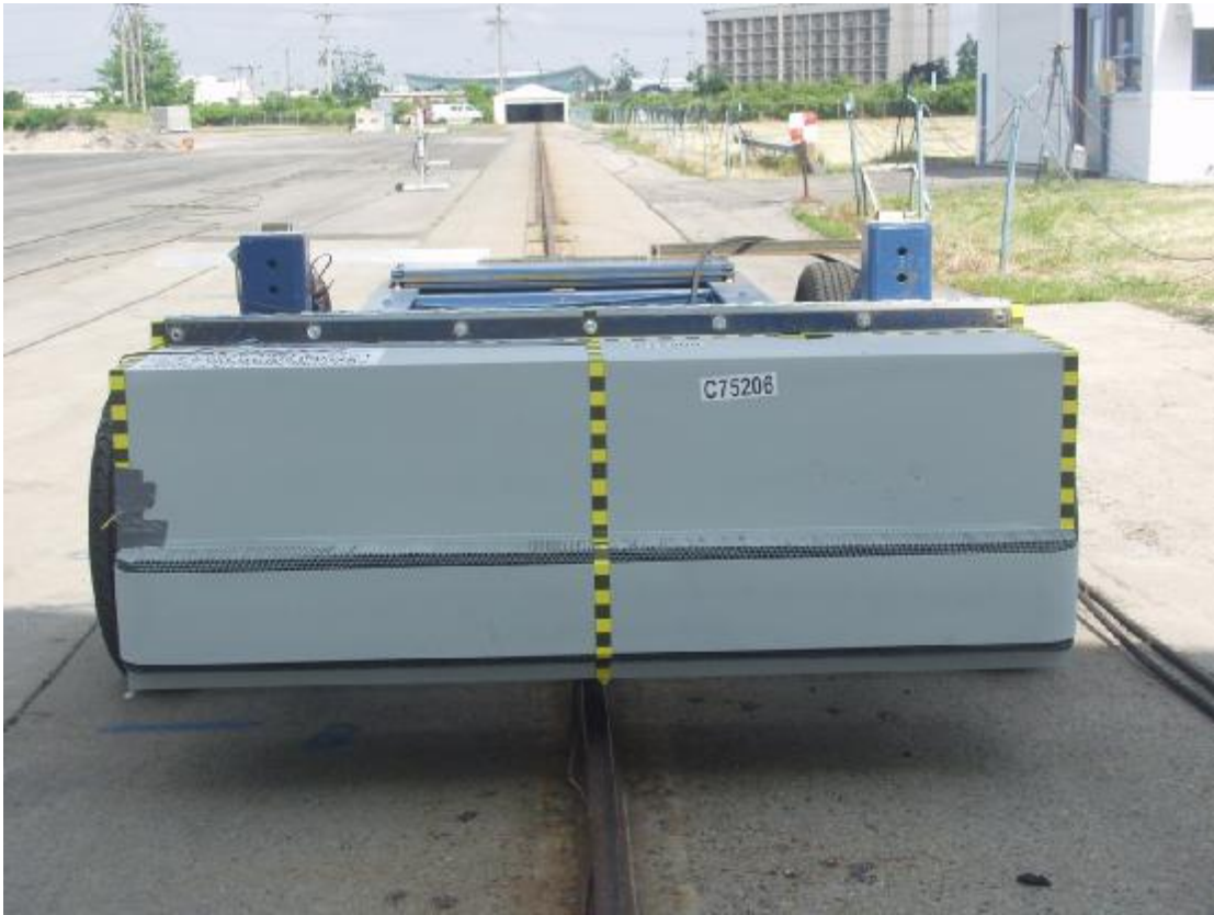
Figure A-19: Pre-Test MDB Front View
