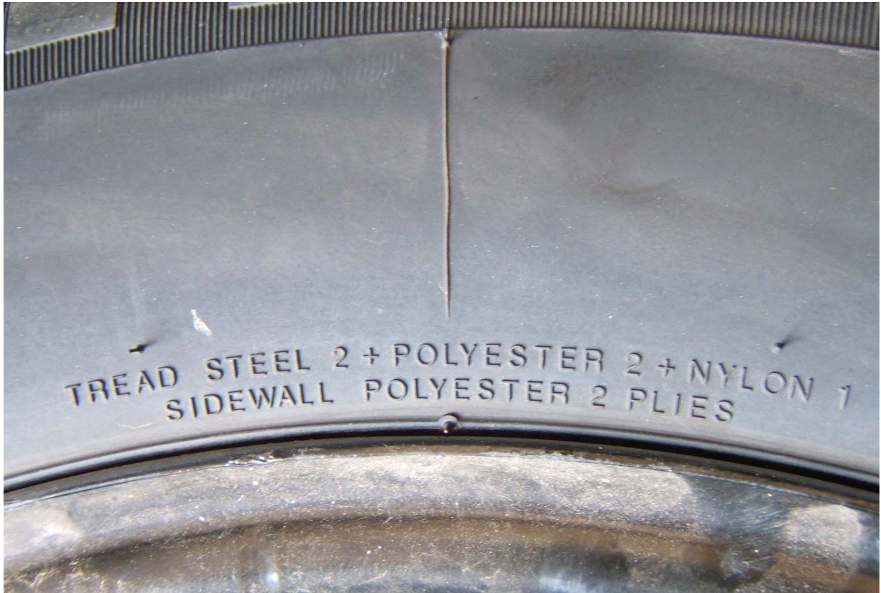
FIGURE 5.9 TIRE SHOWING CONSTRUCTION
