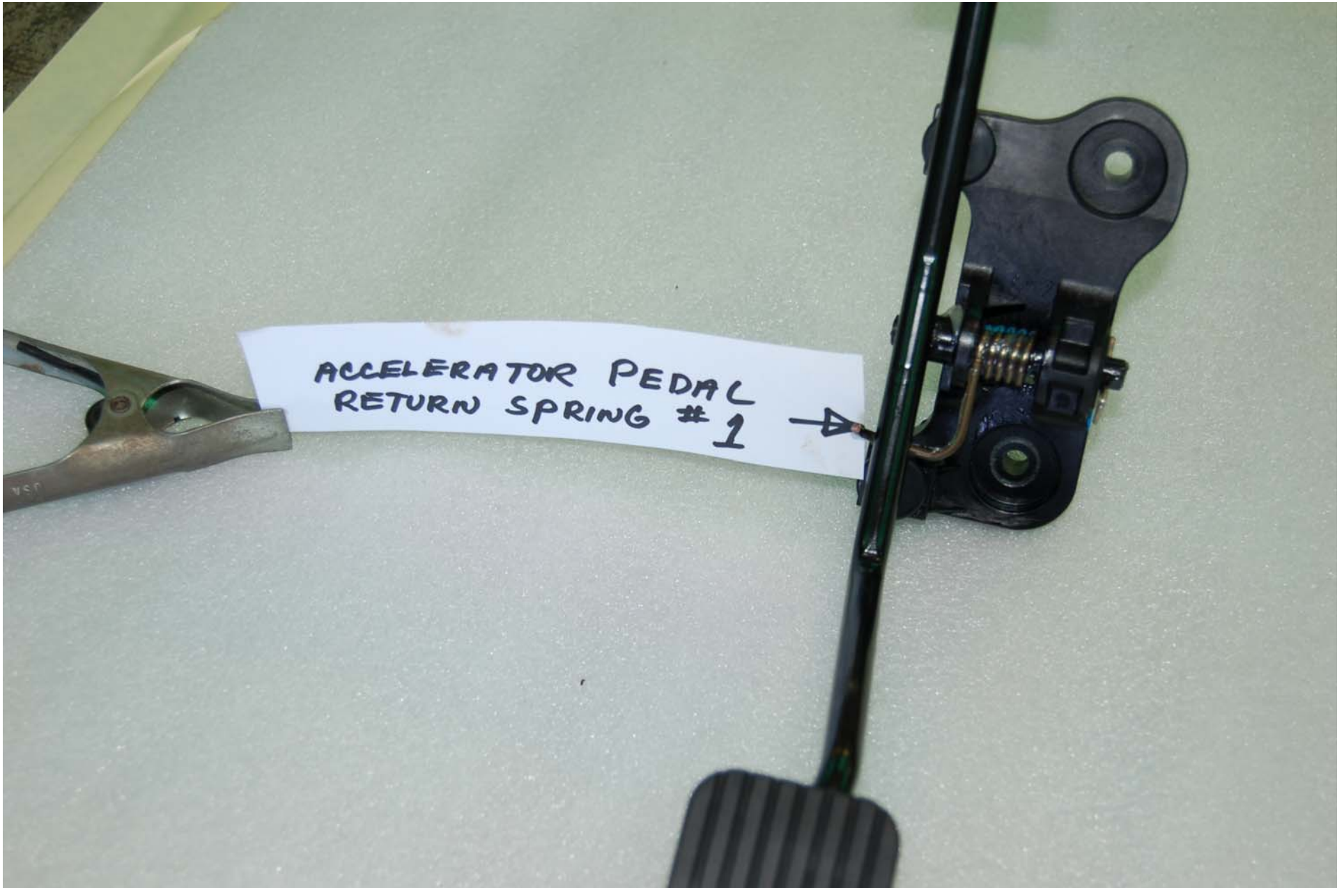
FIGURE 5.7 ACCELERATOR PEDAL ASSEMBLY SHOWING SPRING #1
