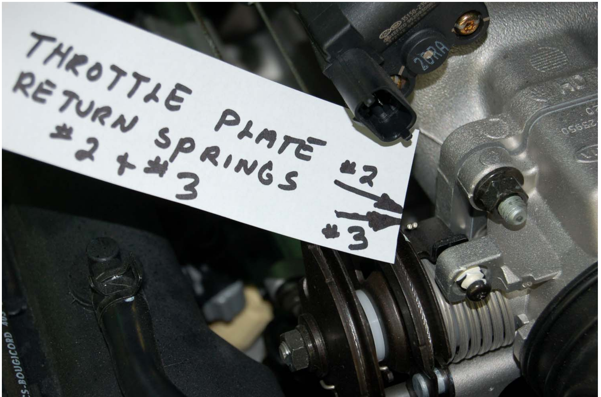
FIGURE 5.10 THROTTLE PLATE RETURN SPRINGS #2 AND #3 (VIEW #2)
