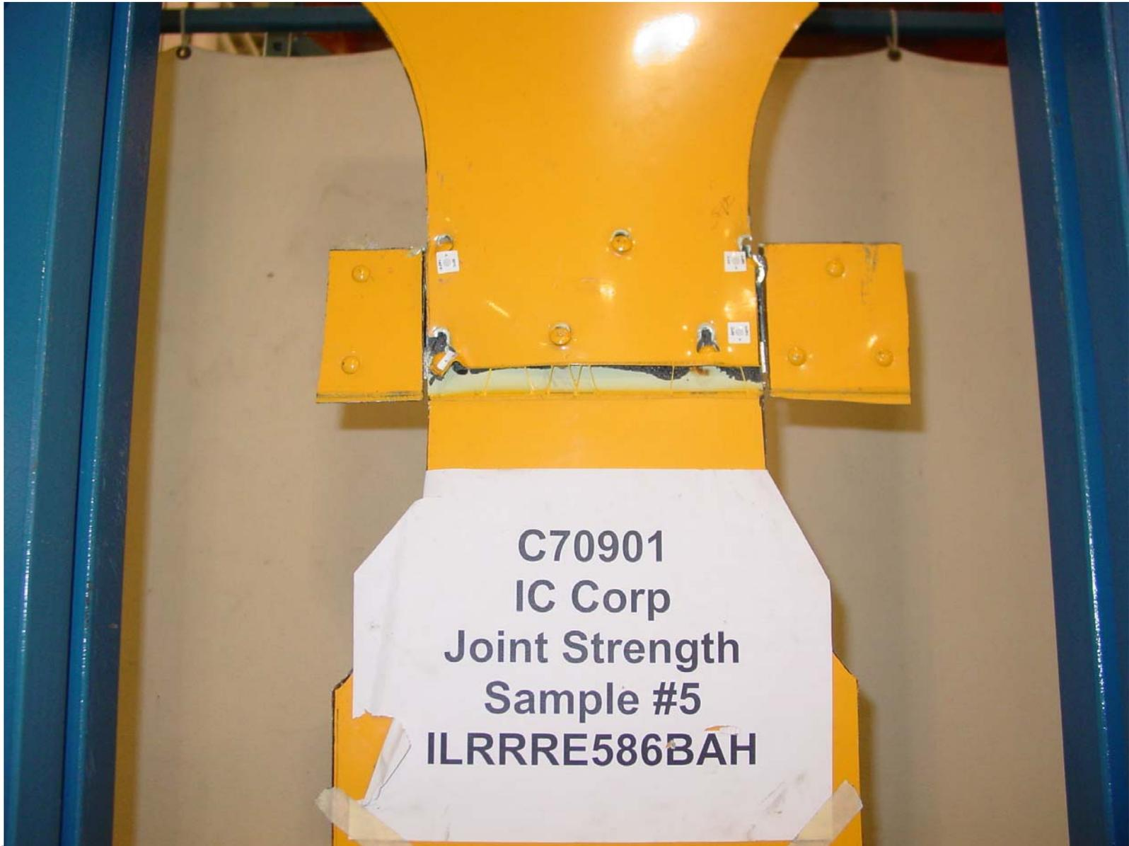
Post-Test of Joint #5 view 2
