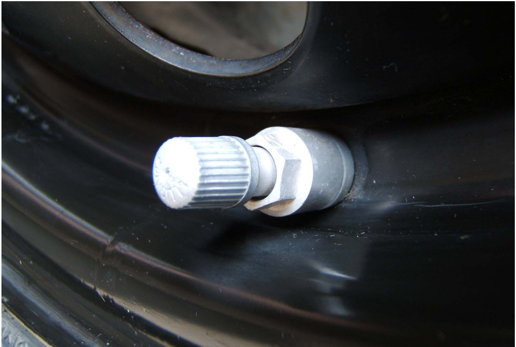
FIGURE 5.10 RIM SHOWING VALVE STEM
