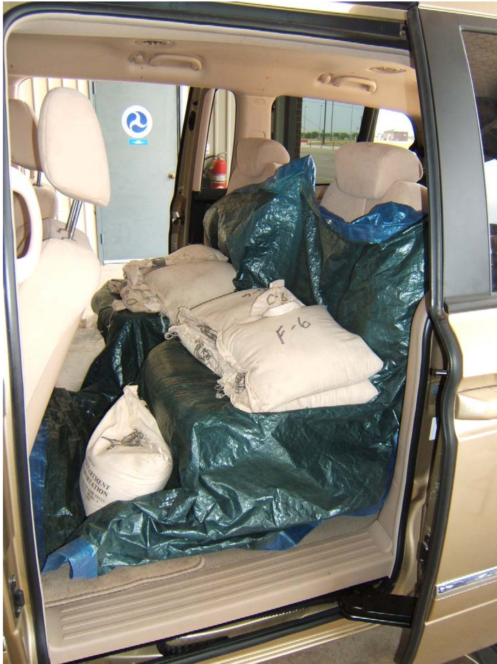
FIGURE 5.14 VEHICLE CENTER SEAT BALLAST FOR VCW LOAD
