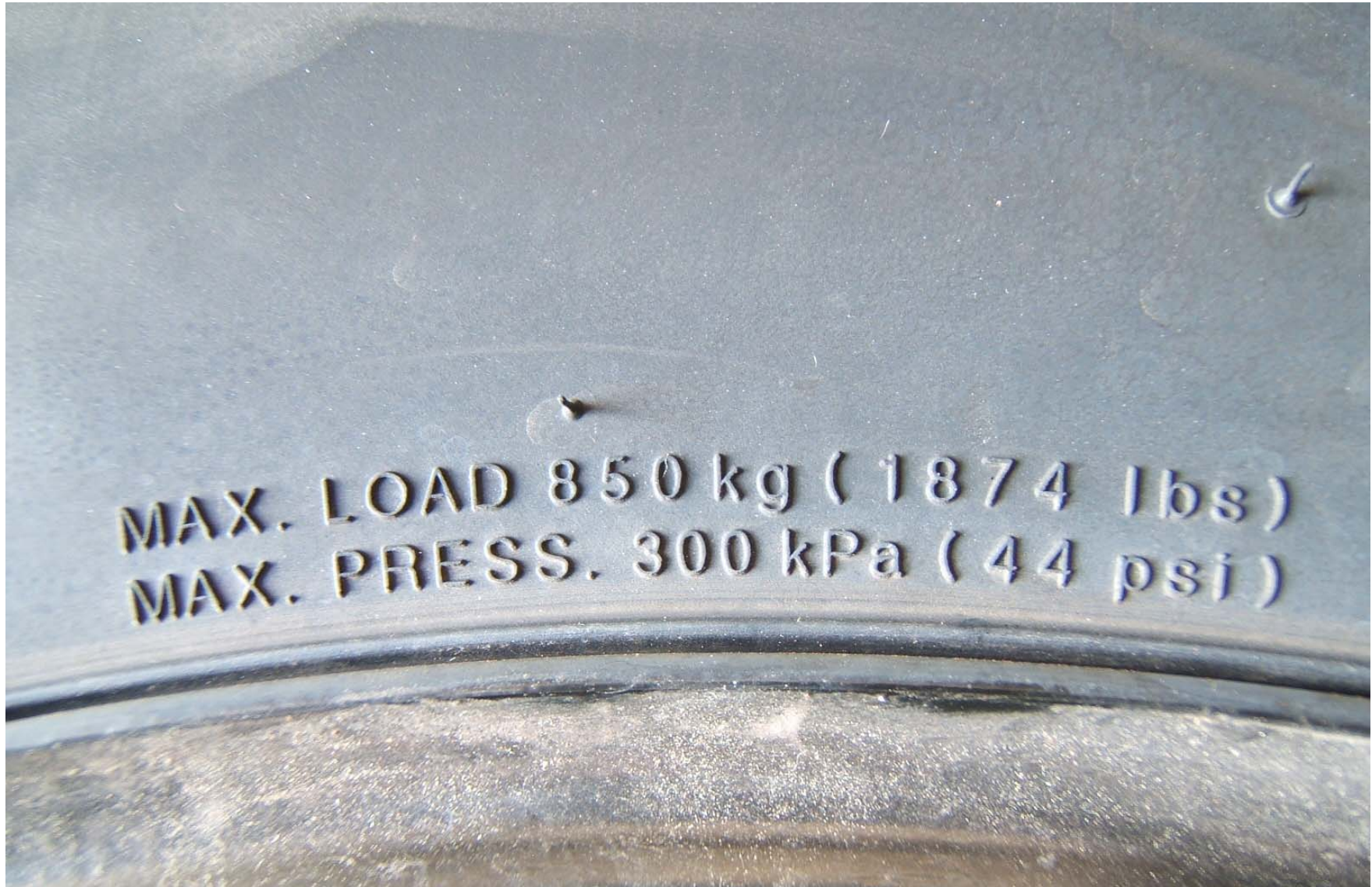
FIGURE 5.8 TIRE SHOWING MAX LOAD RATING AND MAX COLD INFLATION PRESSURE
