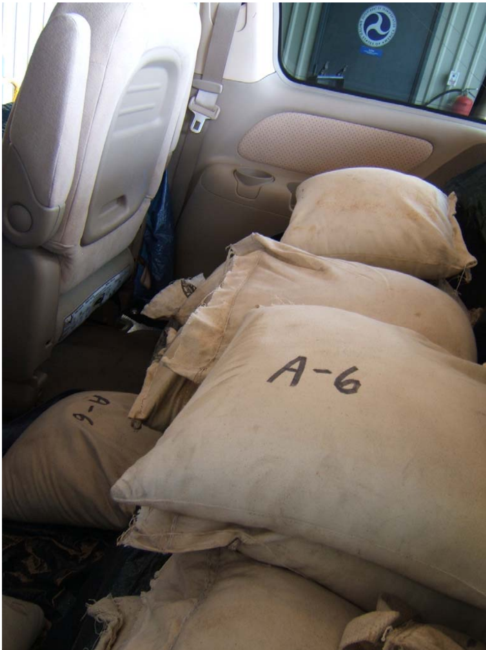
FIGURE 5.15 VEHICLE REAR SEAT BALLAST FOR VCW LOAD
