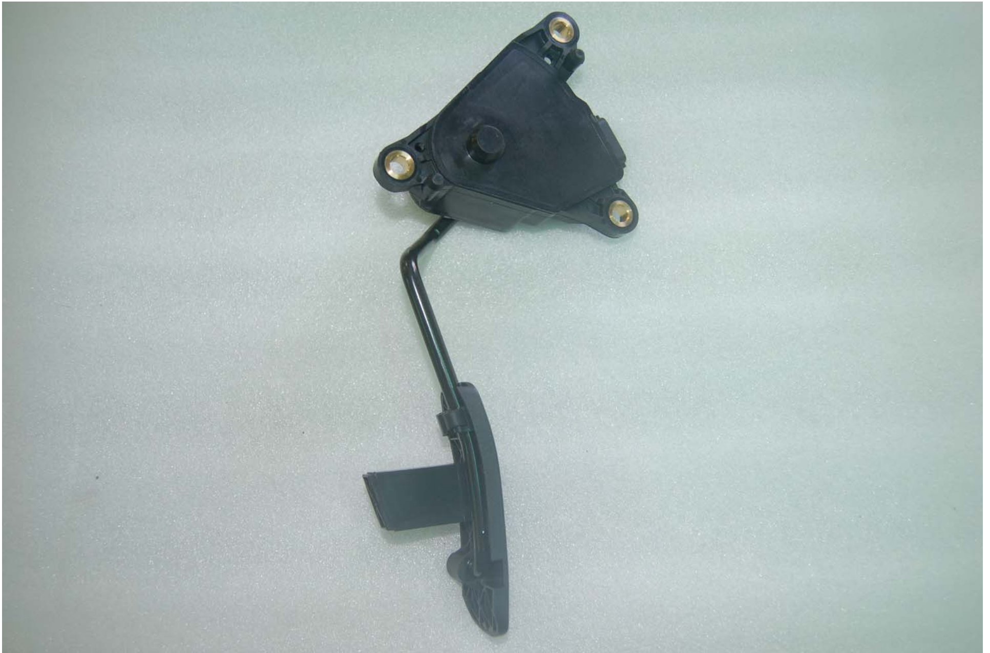
FIGURE 5.8 ACCELERATOR PEDAL ASSEMBLY (APS)
