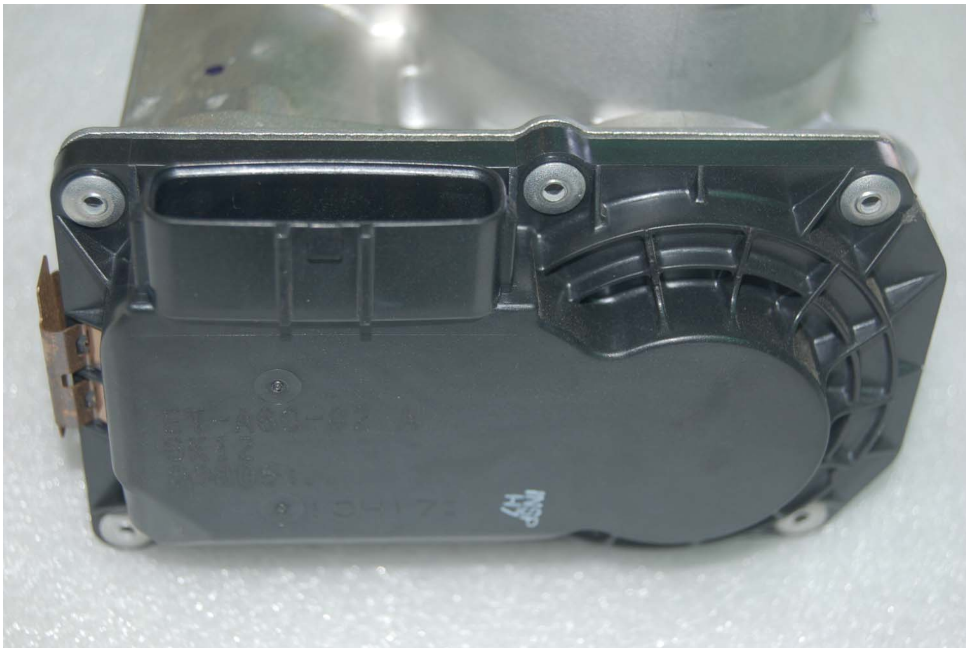
FIGURE 5.13 CLOSE-UP VIEW OF THROTTLE POSITION SENSOR ASSEMBLY
