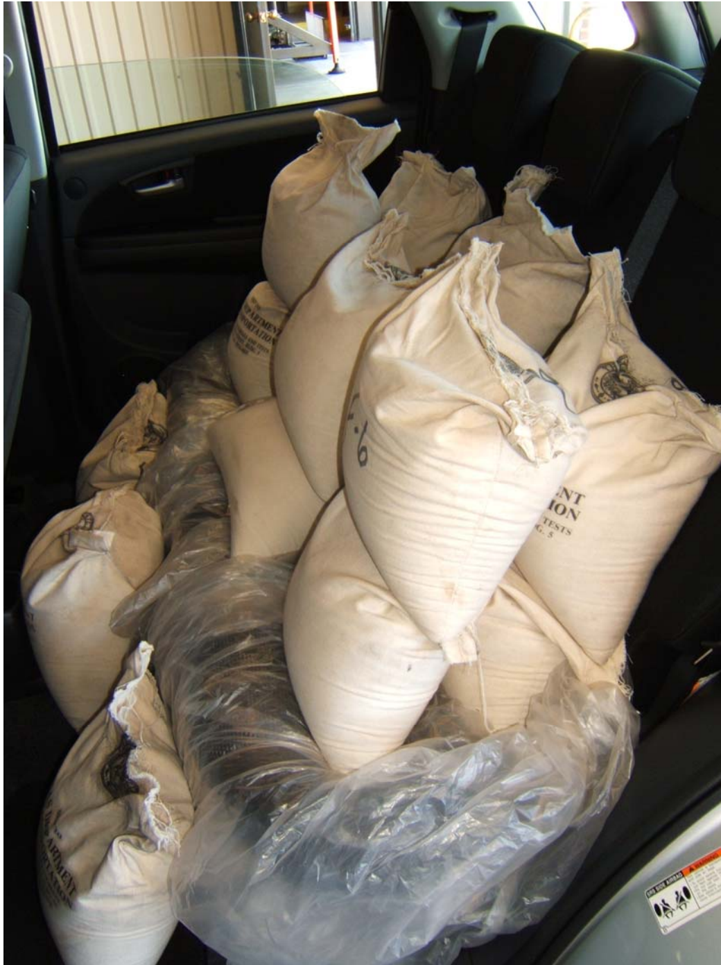
FIGURE 5.18 VEHICLE REAR SEAT BALLASTED FOR MAXIMUM LOAD
