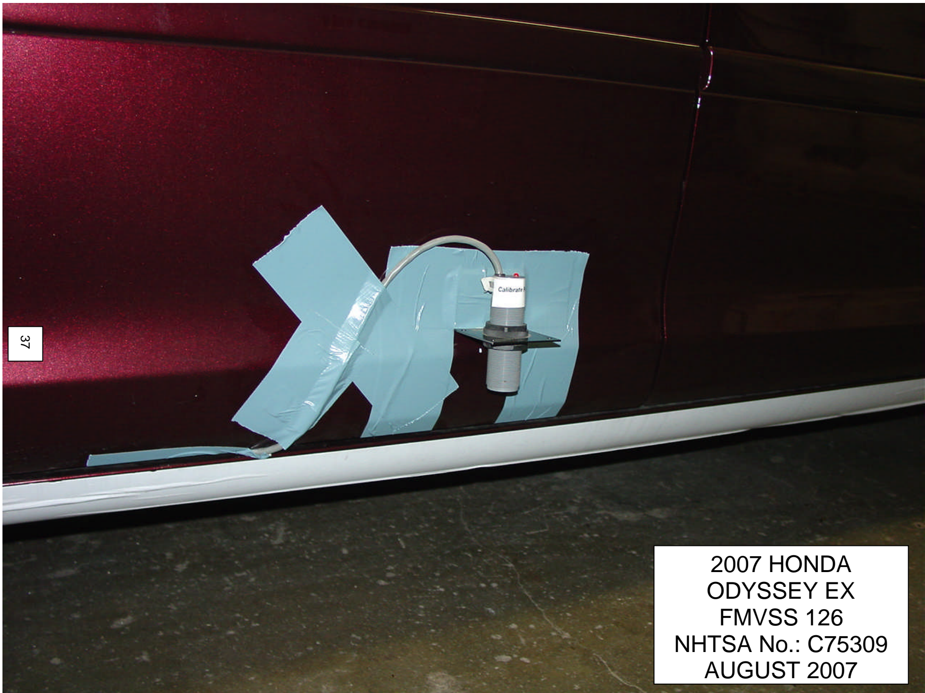
5.11 TEST INSTRUMENTATION – BODY ROLL SENSOR
