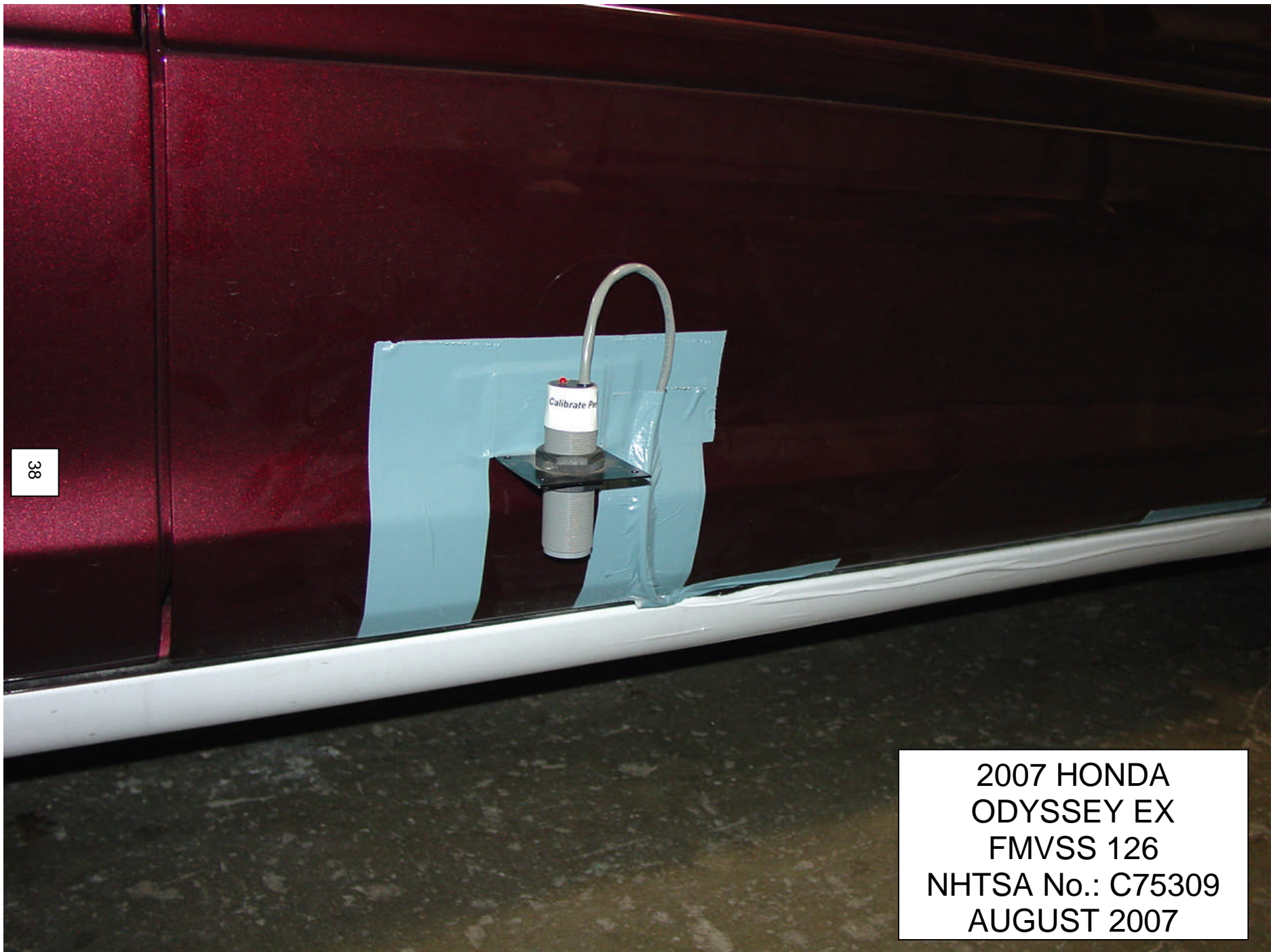
5.12 TEST INSTRUMENTATION – BODY ROLL SENSOR
