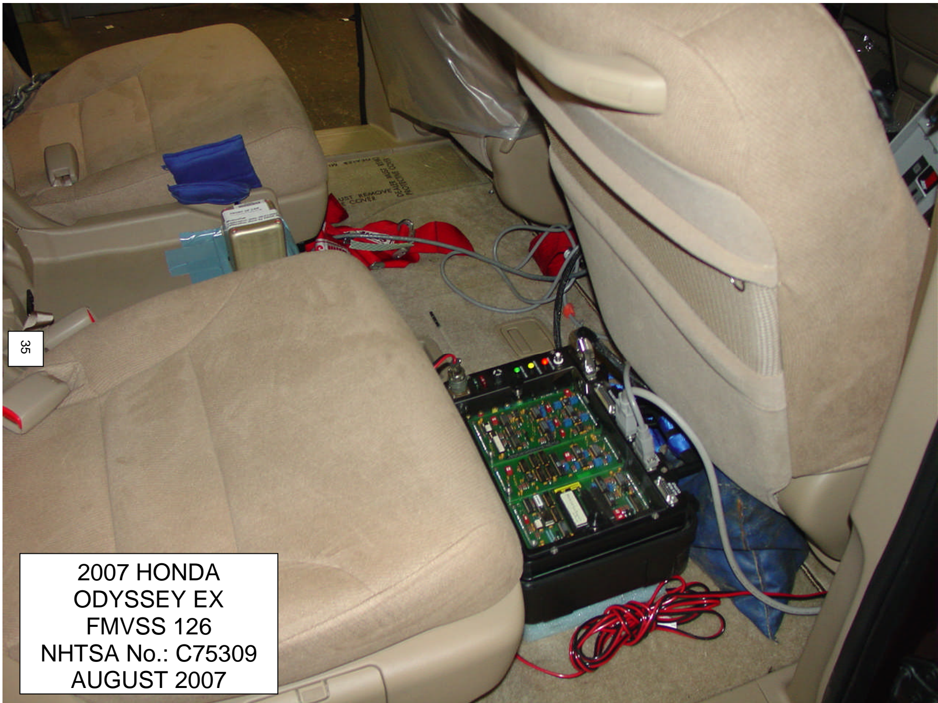
5.9 TEST INSTRUMENTATION – STEERING CONTROLLER BATTERY BOX AND BALLAST
