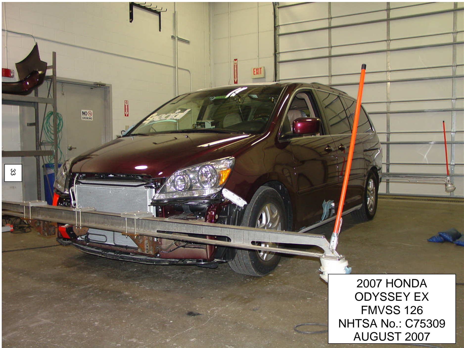
5.7 TEST VEHICLE WITH OUTRIGGERS
