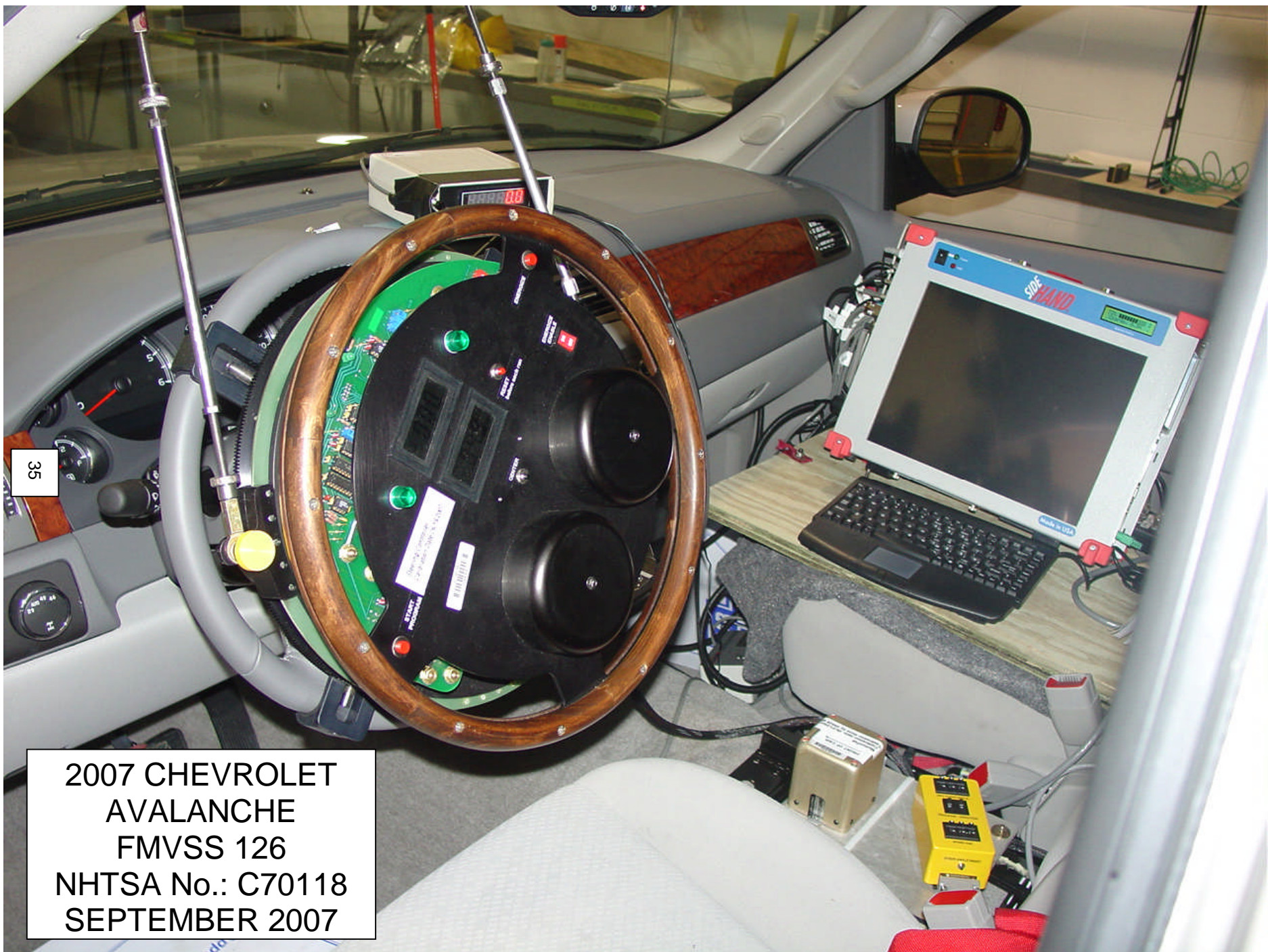
5.9 TEST INSTRUMENTATION – STEERING WHEEL CONTROLLER AND DATA ACQUISITION SYSTEM
