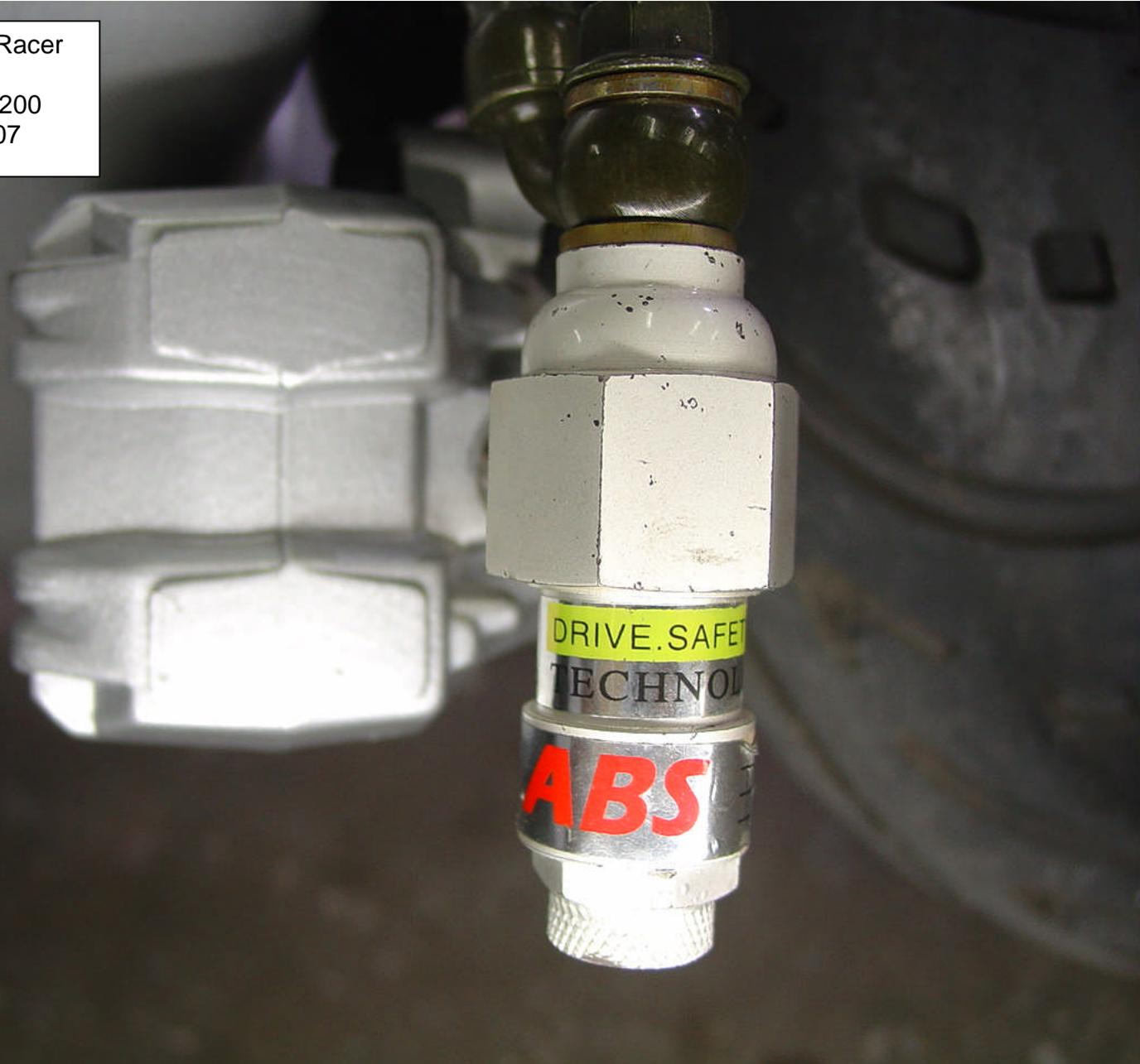
Front Brake Component Labeled as ABS
