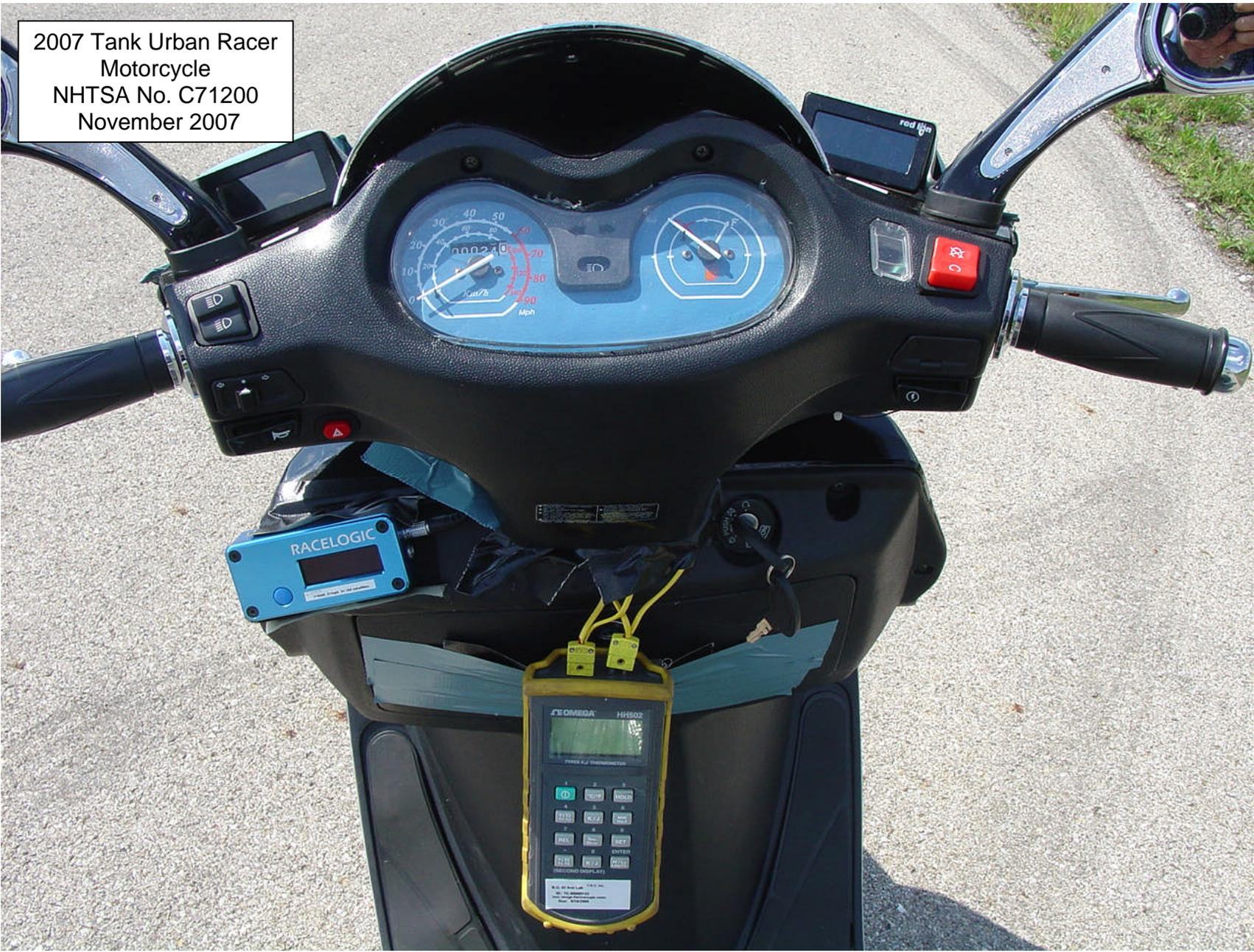
Instrumentation Installed on Vehicle
