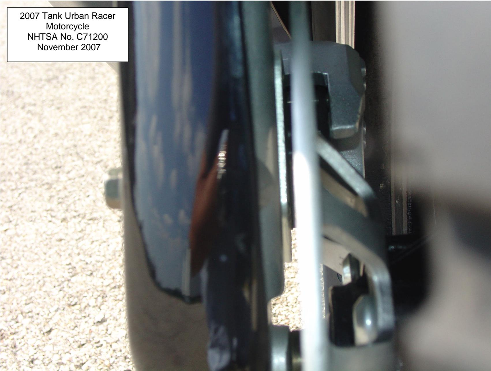
Visual Inspection of Front Brake Lining Thickness Provision
