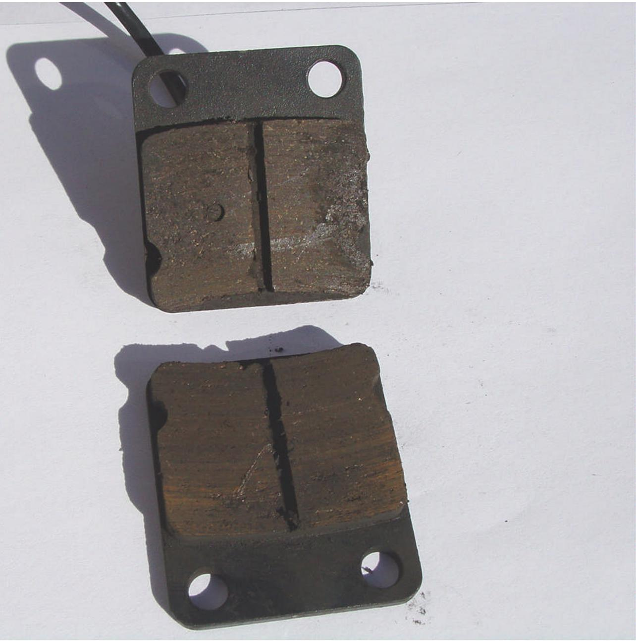
Condition, Front Brake Linings – Post Test
