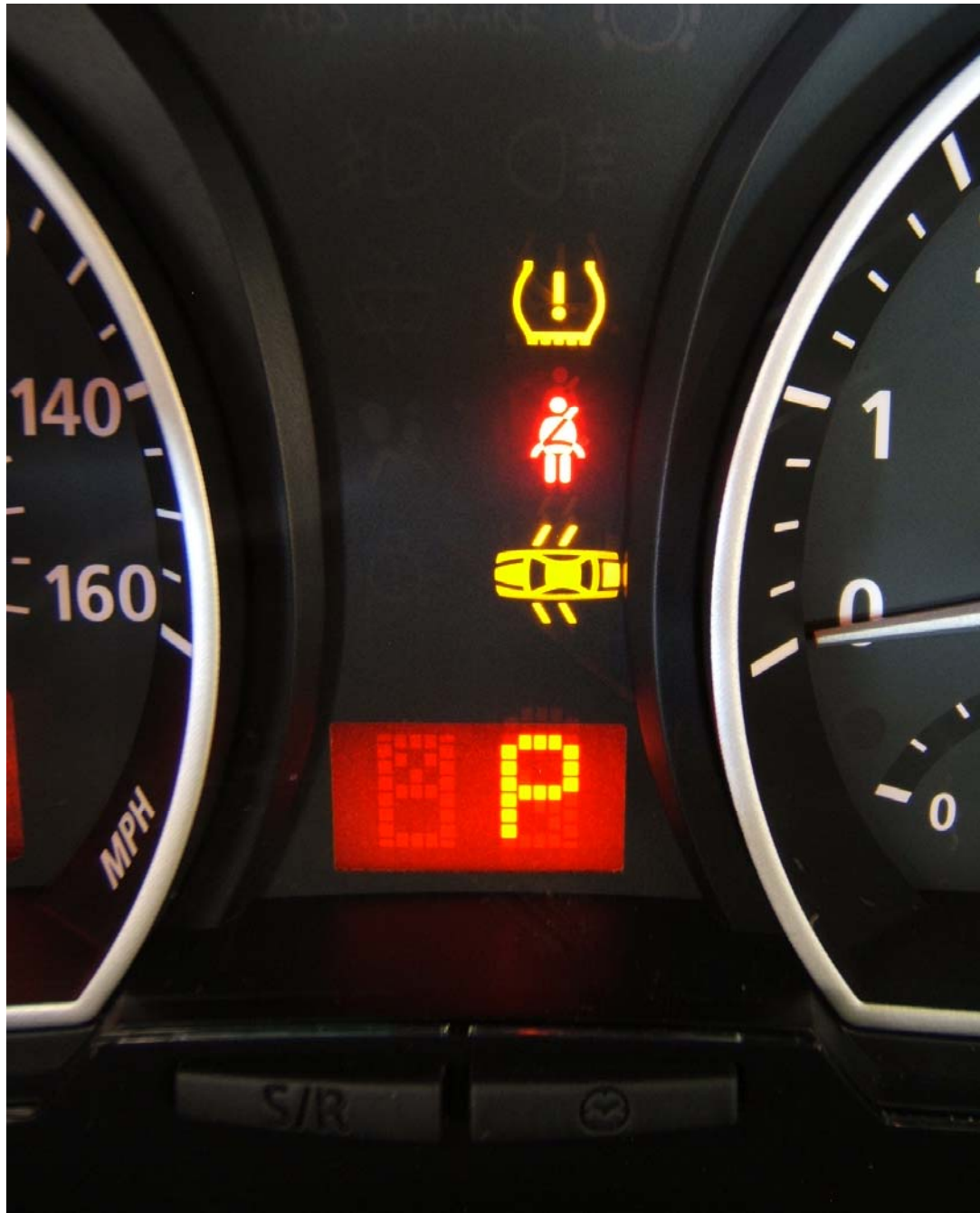
FIGURE 5.11 INSTRUMENT PANEL SHOWING COMBINATION LOW TIRE PRESSURE TELLTALE / MALFUNCTION TELLTALE
