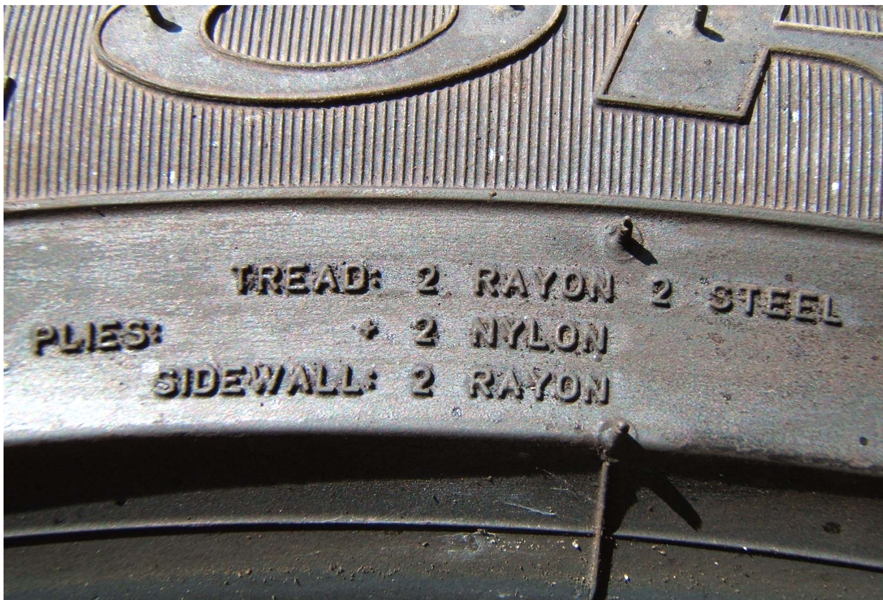
FIGURE 5.9 TIRE SHOWING SIDEWALL/TREAD CONSTRUCTION
