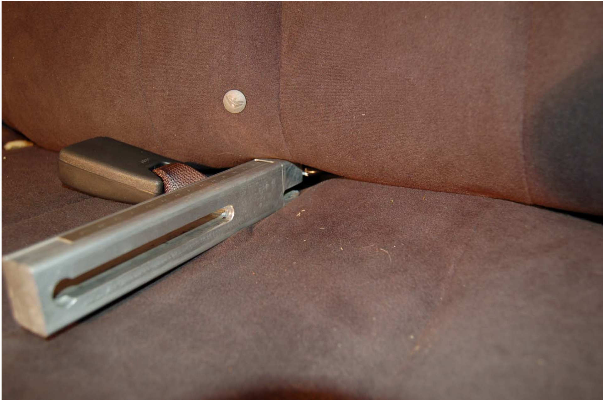
FIGURE 5.27 INTERFERENCE OF SEAT BACK WITH CRF LEG
