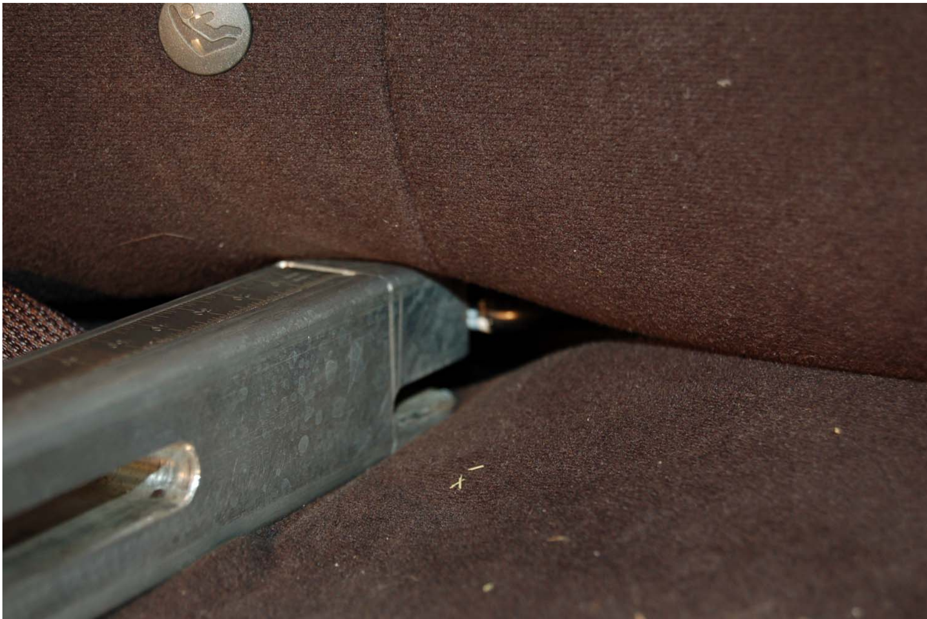
FIGURE 5.28 INTERFERENCE OF SEAT BACK WITH CRF LEG
