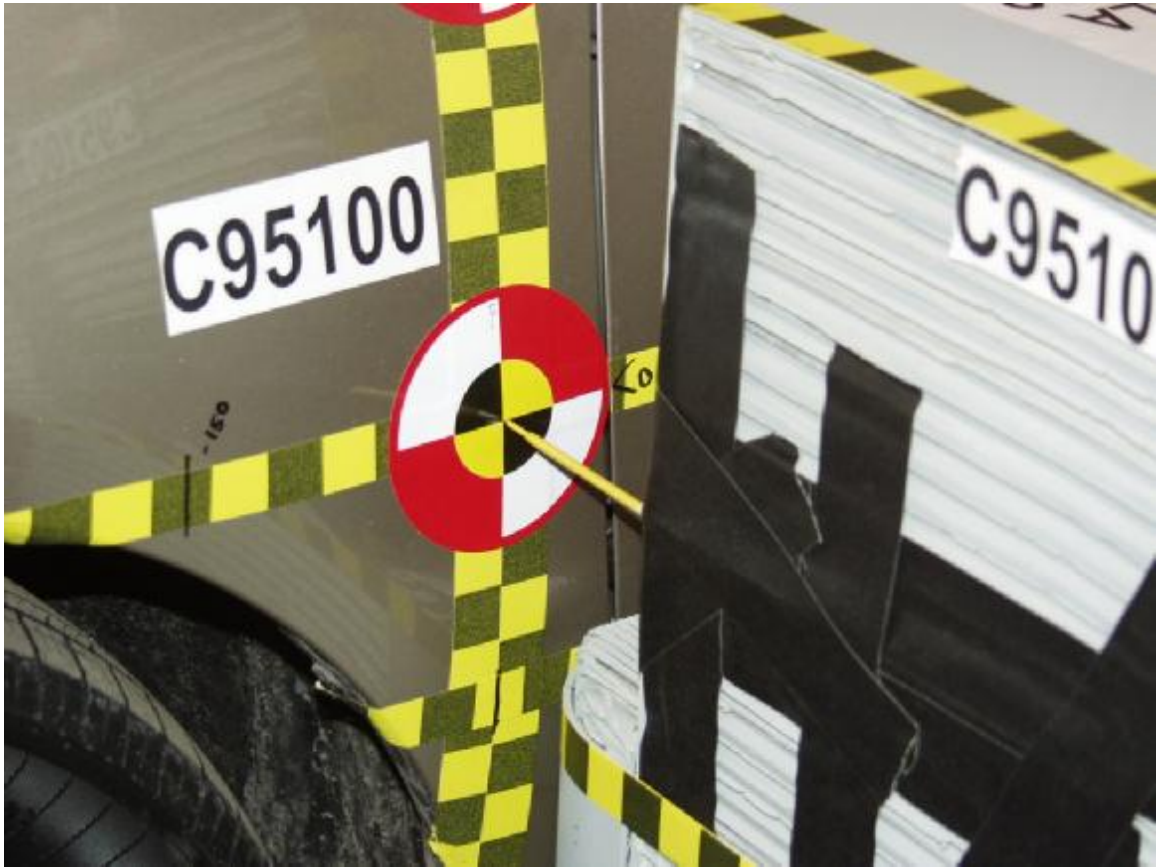
Figure A-33: Pre-Test Close-Up View of Impact Point Target
