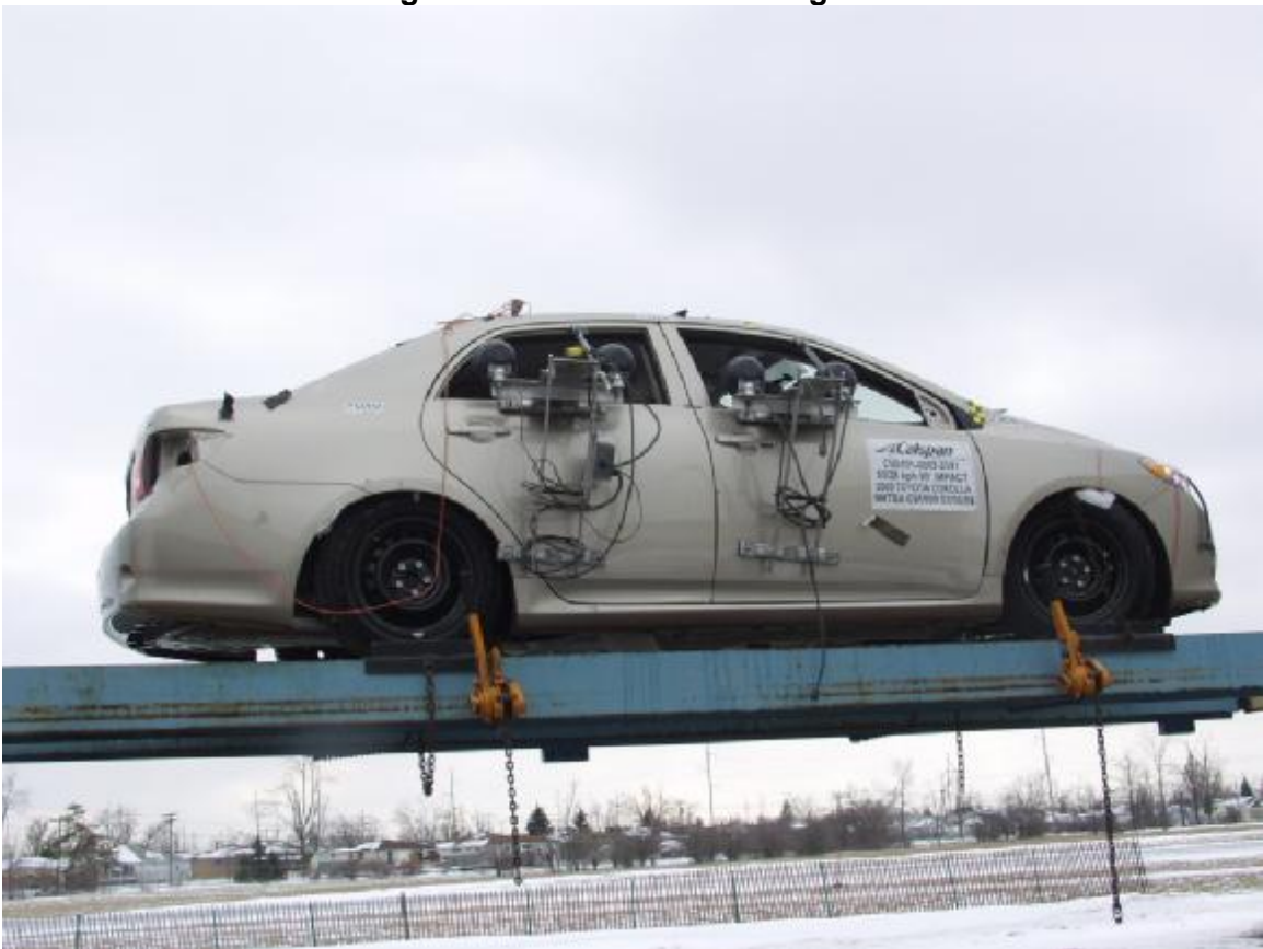
Figure A-54: Rollover 360 Degrees
