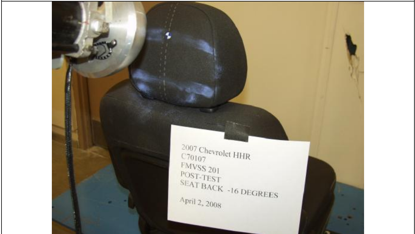
Figure A-22: HEAD RESTRAINT IMPACT AREA POST-TEST
