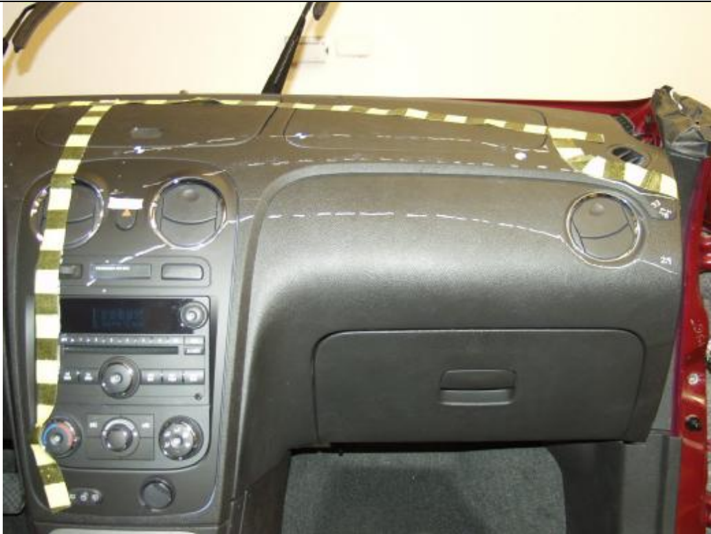
Figure A-14: DELINEATED INSTRUMENT PANEL IMPACT ZONE PRE-TEST
