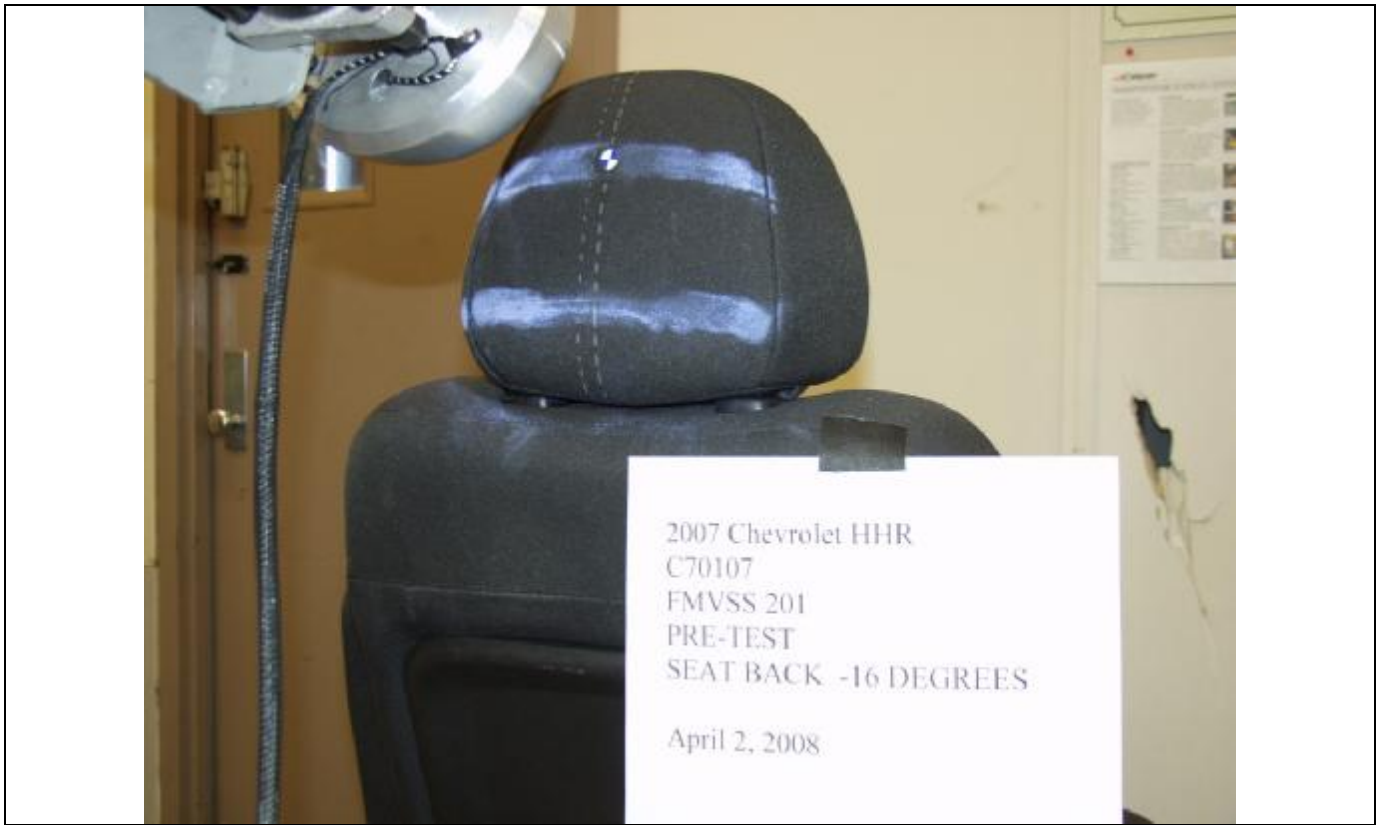
Figure A-21: HEAD RESTRAINT IMPACT AREA PRE-TEST
