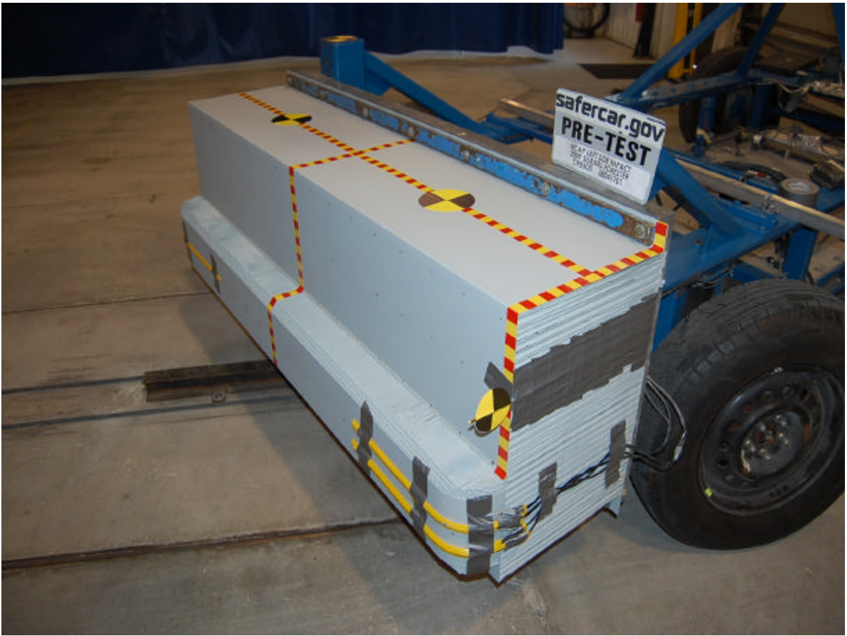
Pre-Test Left Side View of Deformable Barrier
