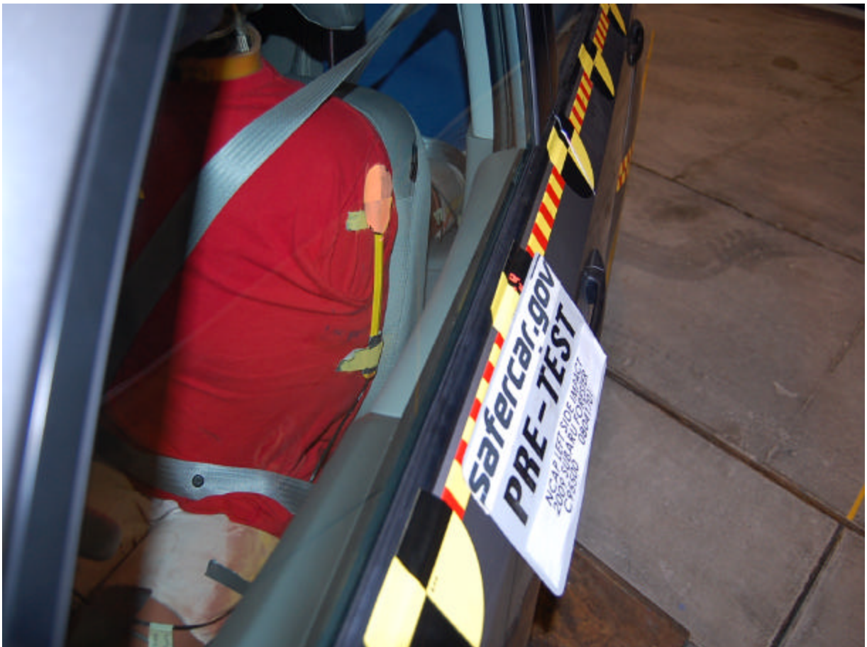
Pre-Test Driver Dummy Clearance From Door
