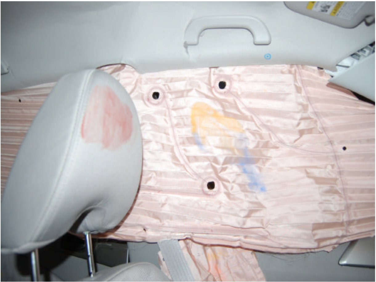
Post-Test Driver Dummy Head Contact
