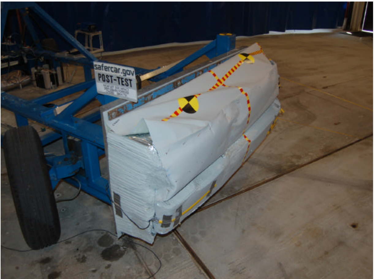
Post-Test Right Side View of Deformable Barrier
