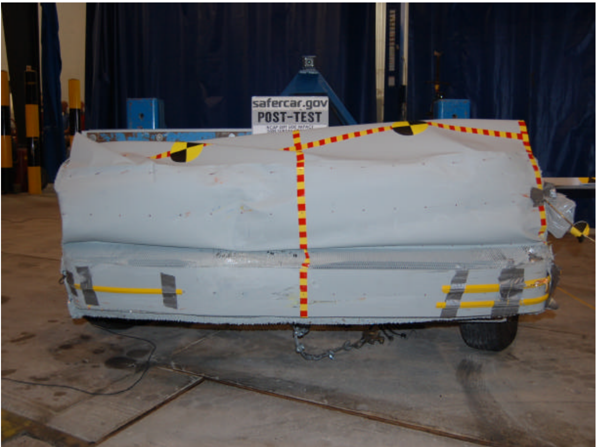
Post-Test Front View of Deformable Barrier
