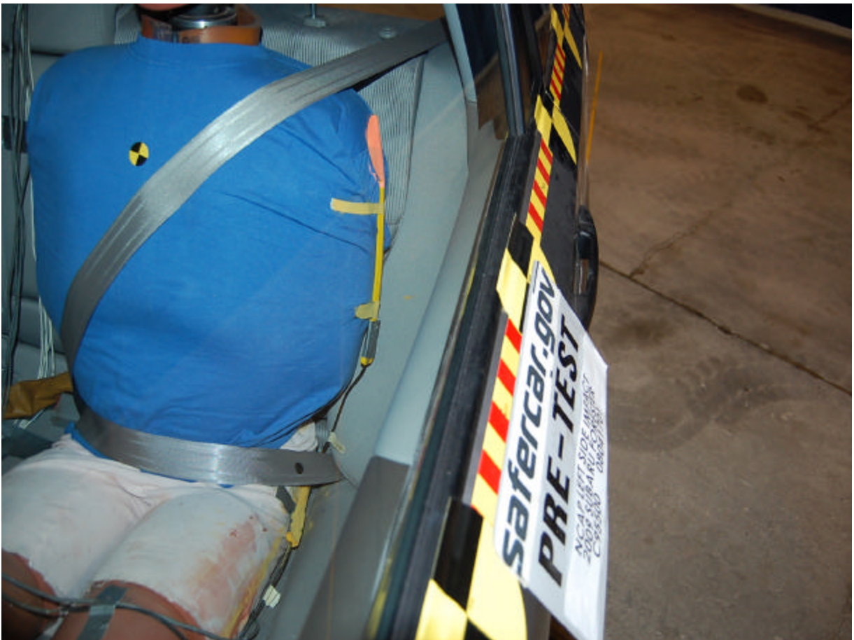
Pre-Test Passenger Dummy Clearance From Door
