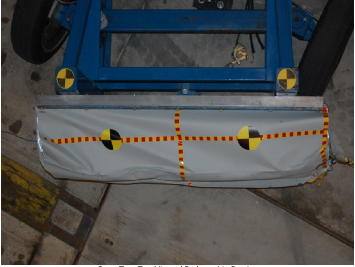
Post-Test Top View of Deformable Barrier
