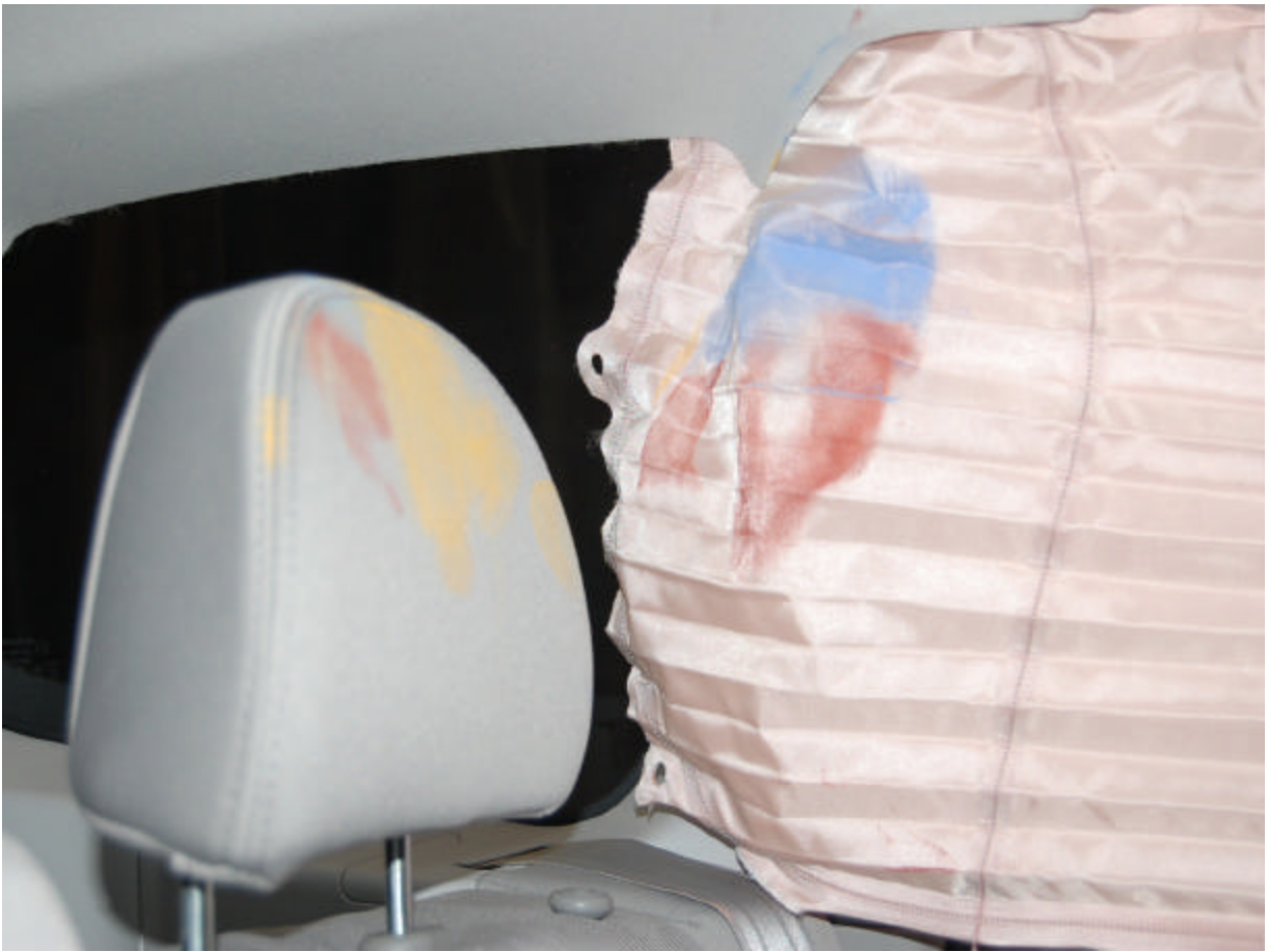
Post-Test Passenger Dummy Head Contact
