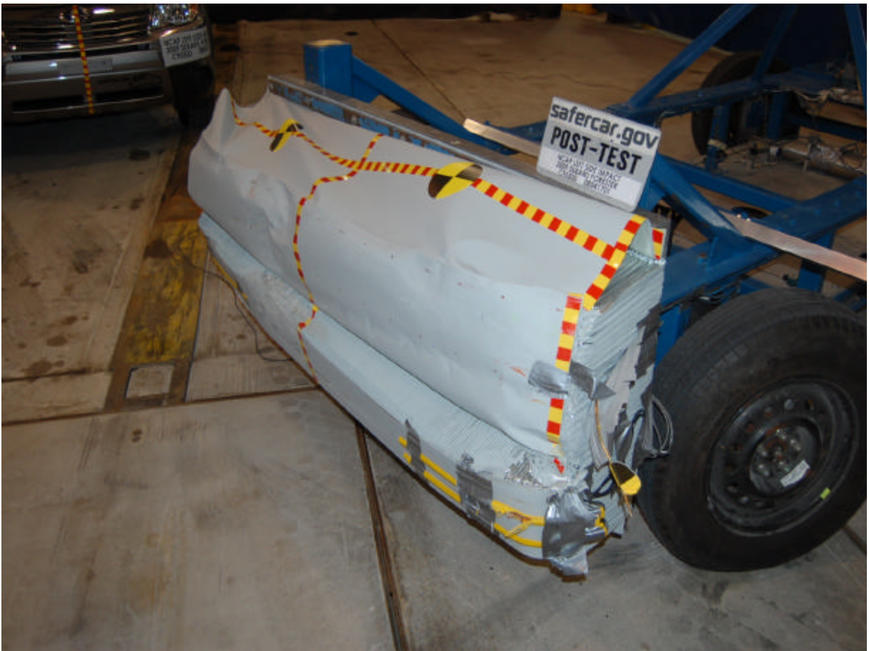
Post-Test Left Side View of Deformable Barrier
