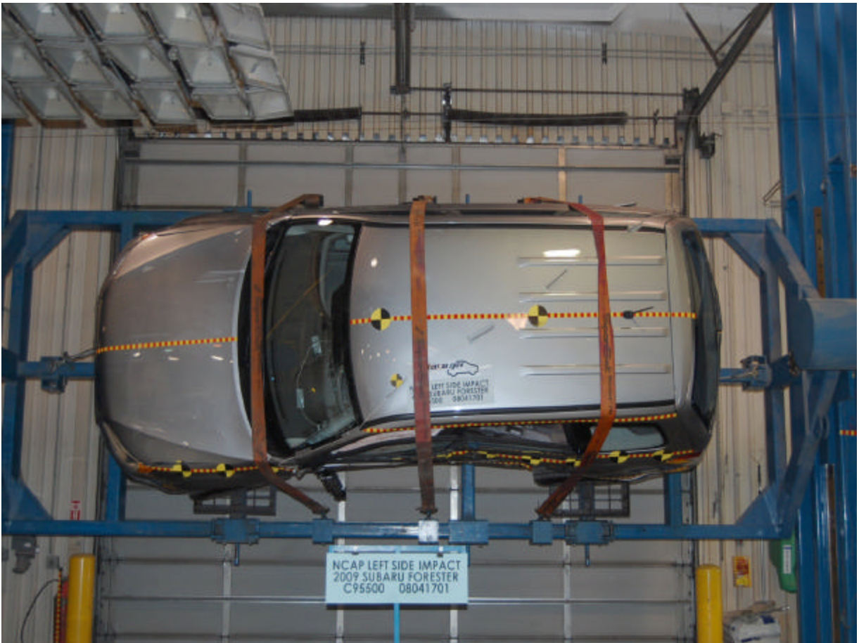
Vehicle on Rollover Device (270 Degrees)
