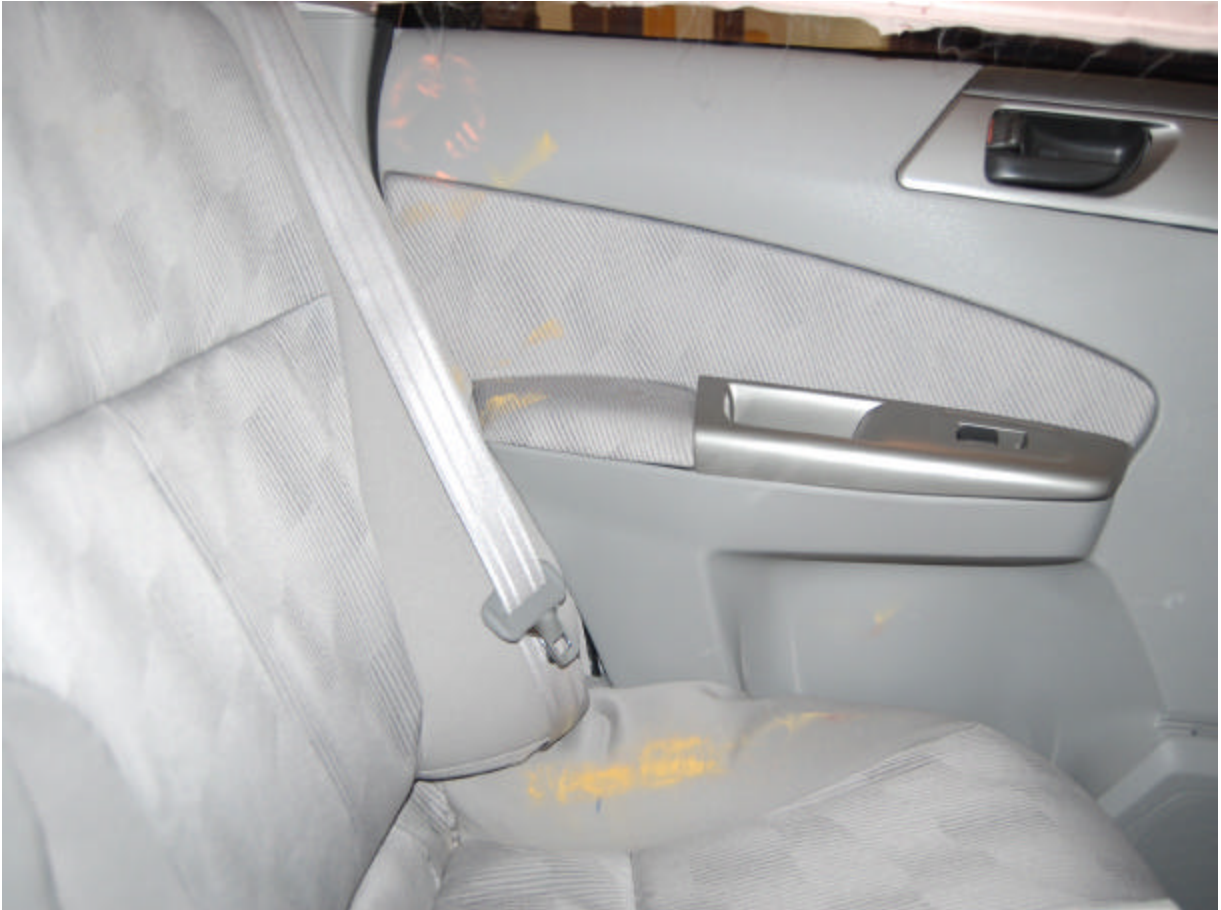
Post-Test Passenger Dummy Torso Contact
