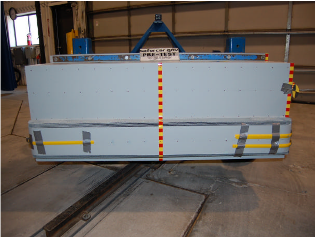
Pre-Test Front View of Deformable Barrier
