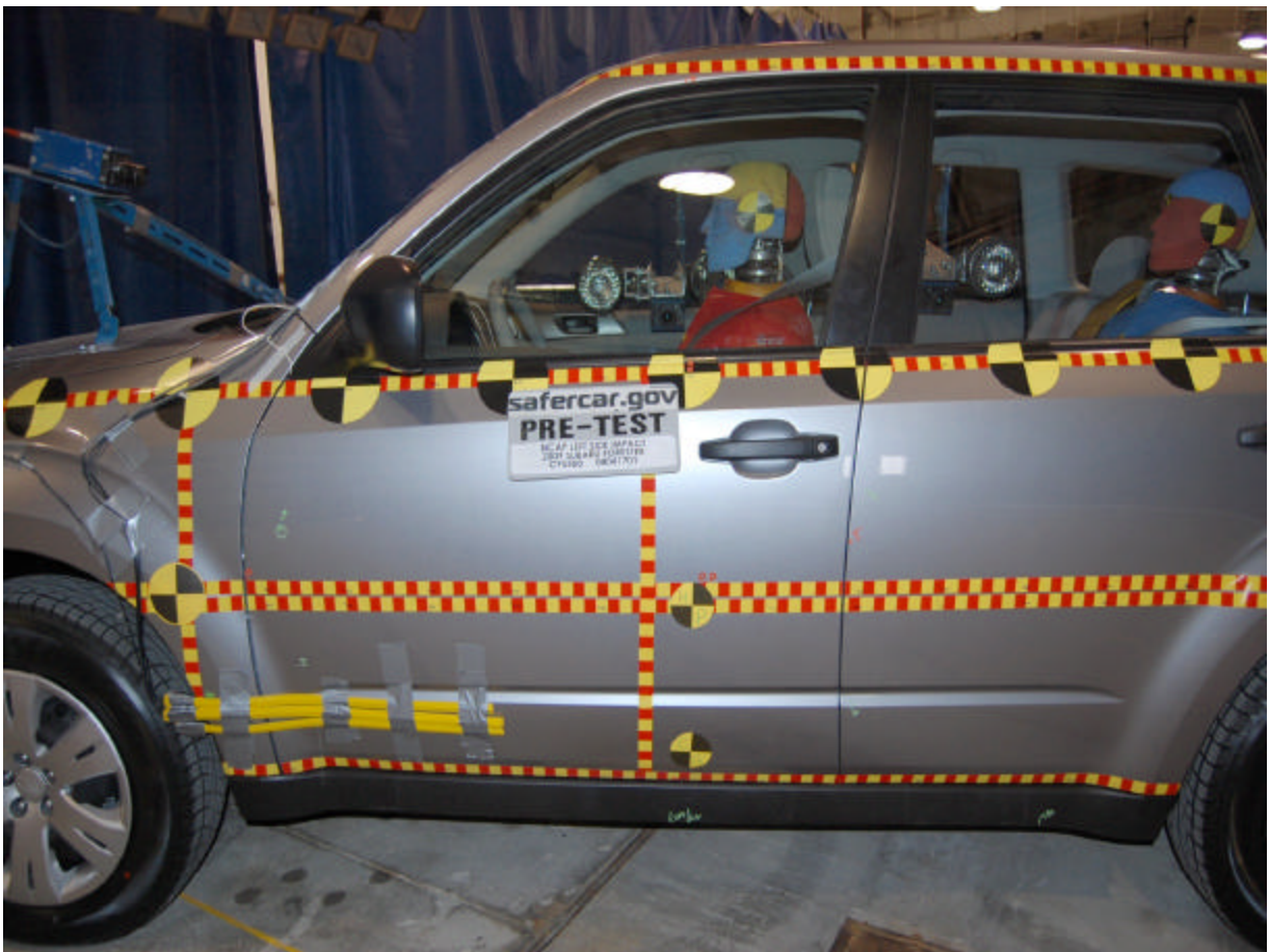
Pre-Test Left Side Impact Close-Up View
