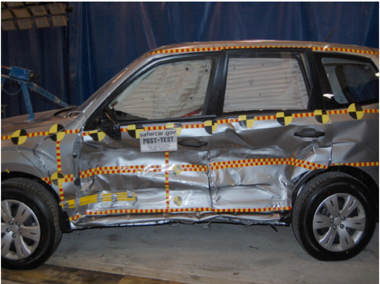
Post-Test Left Side Impact Close-Up View
