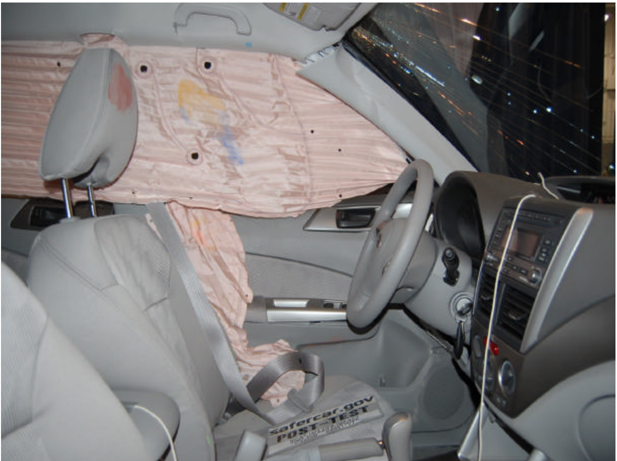
Post-Test Driver Dummy Contact
