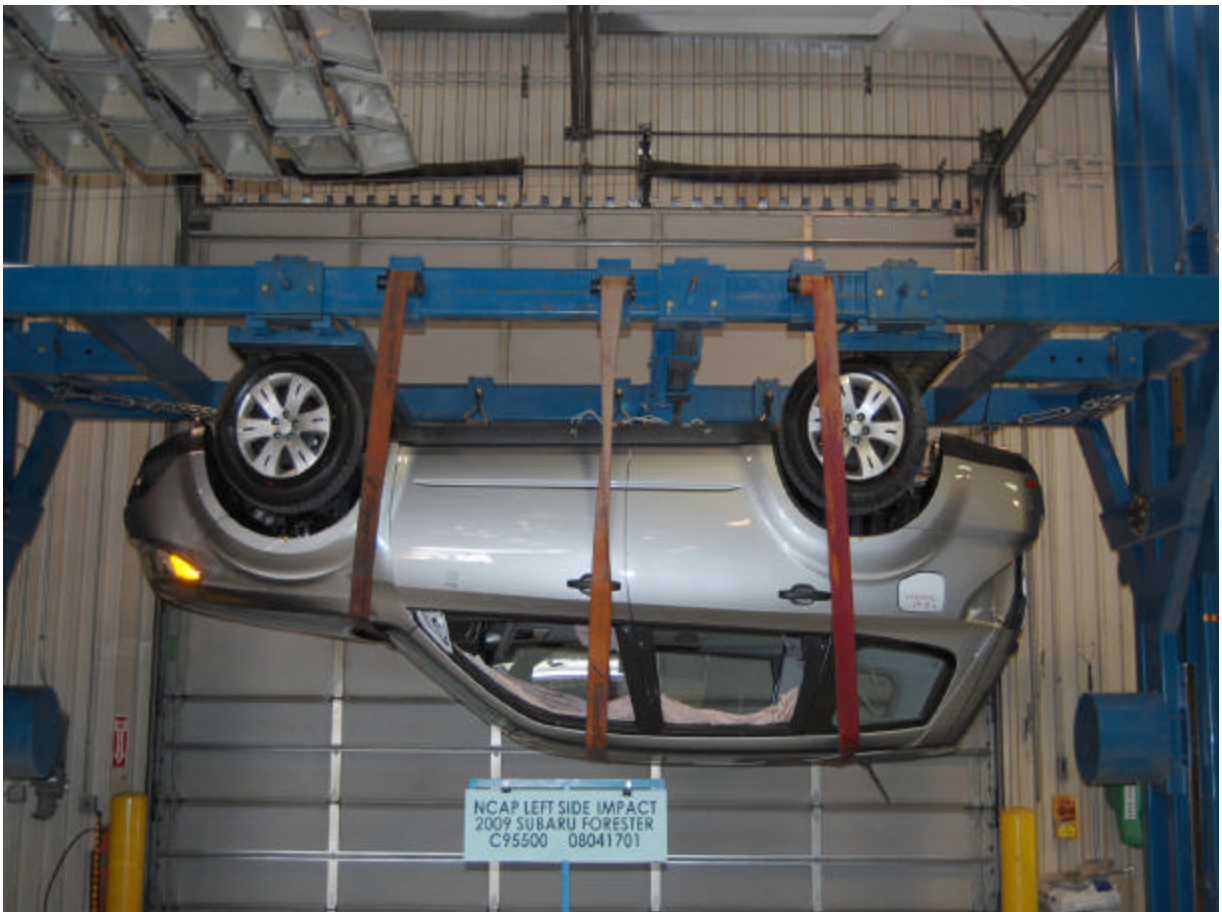
Vehicle on Rollover Device (180 Degrees)
