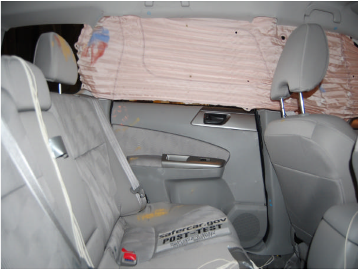
Post-Test Passenger Dummy Contact
