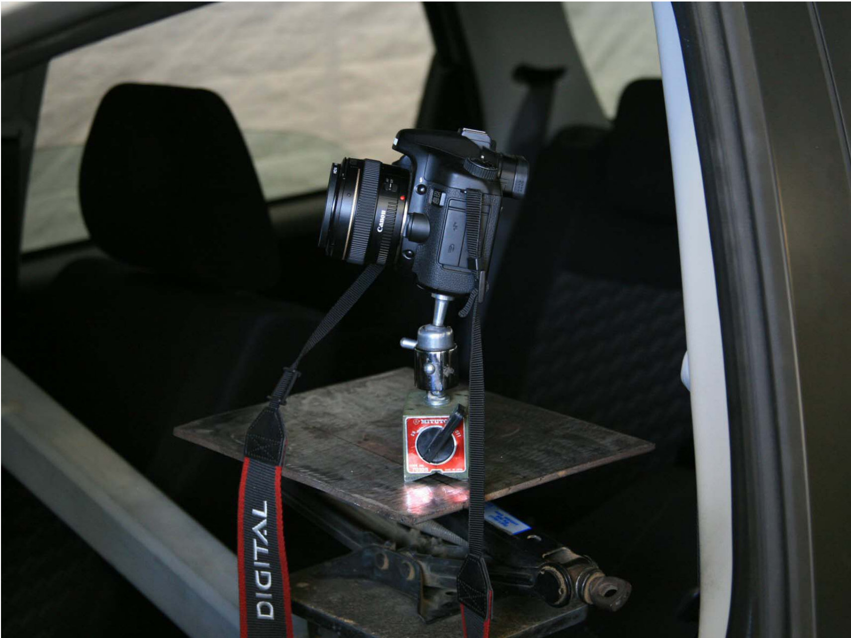
FIGURE 11:CAMERA SET-UP FOR PHOTOGRAPHING REFERENCE BOARD
