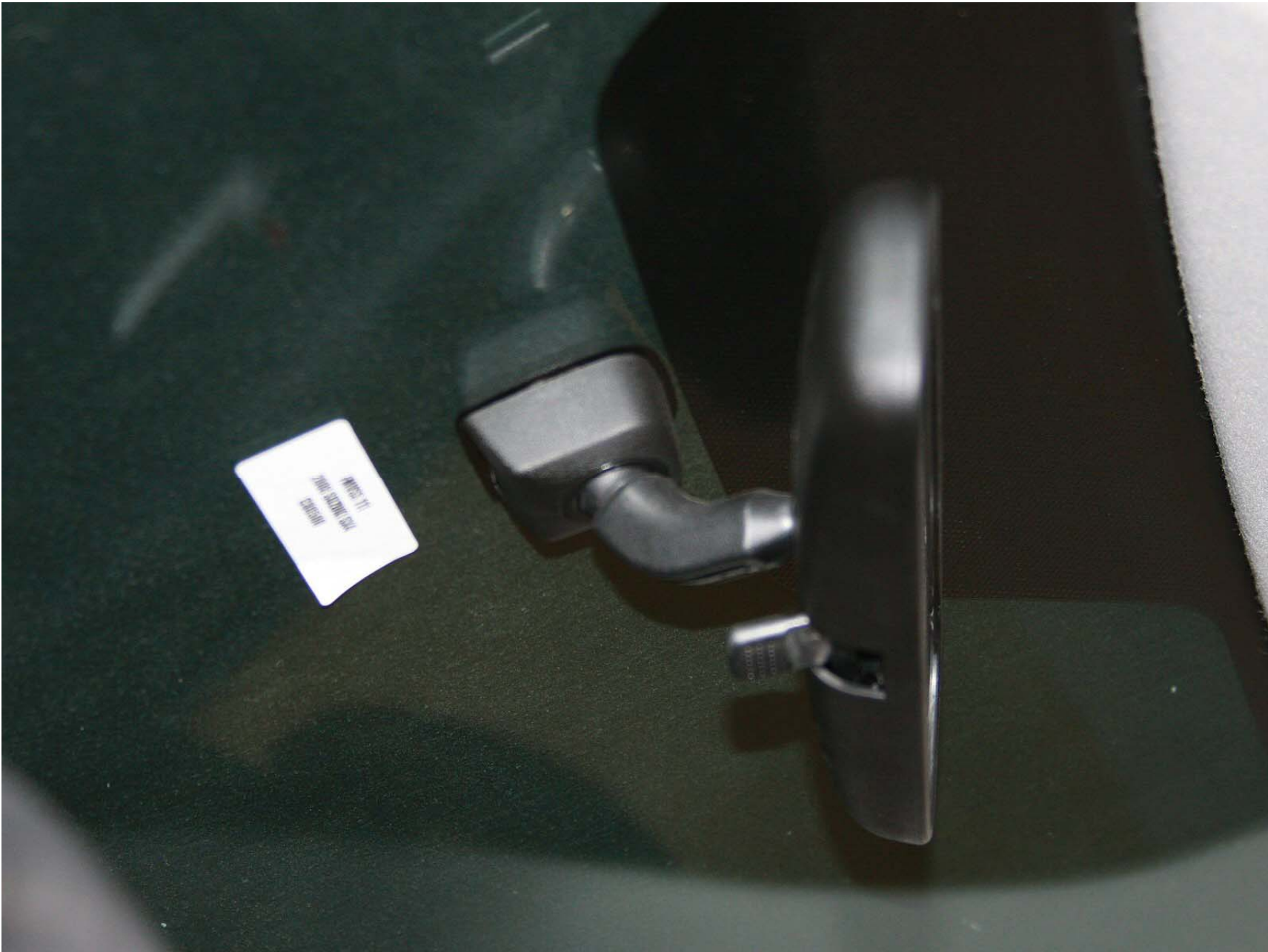
FIGURE 9: INSIDE REARVIEW MIRROR AND MOUNTING
