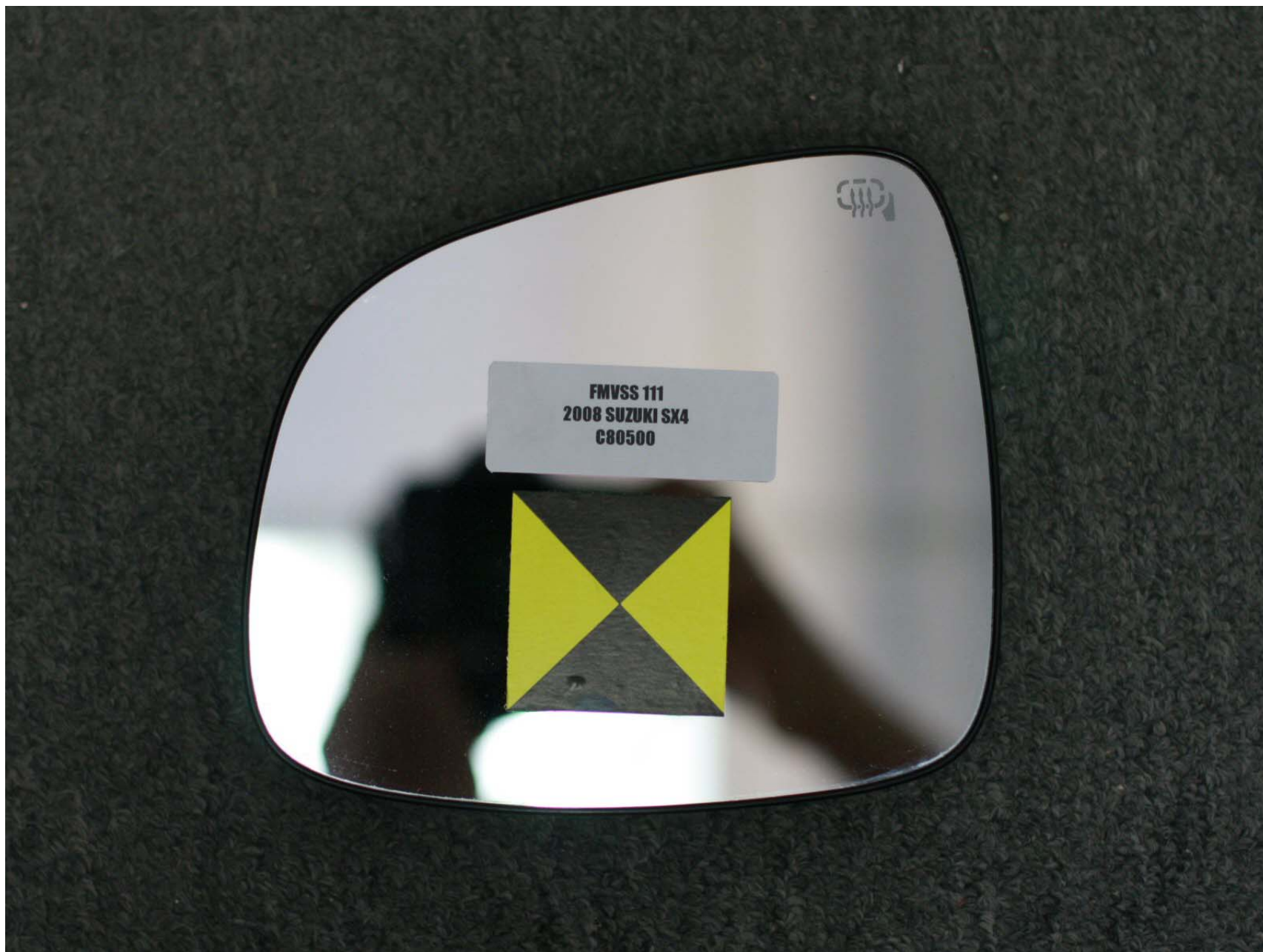
FIGURE 15: MIRROR SET-UP FOR AREA MEASUREMENT
