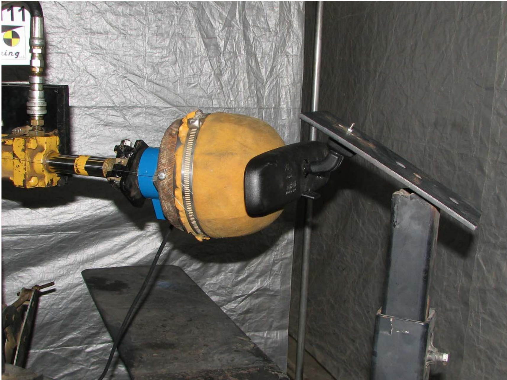
FIGURE 13:CLOSE-UP OF MIRROR BREAK- AWAY TEST
