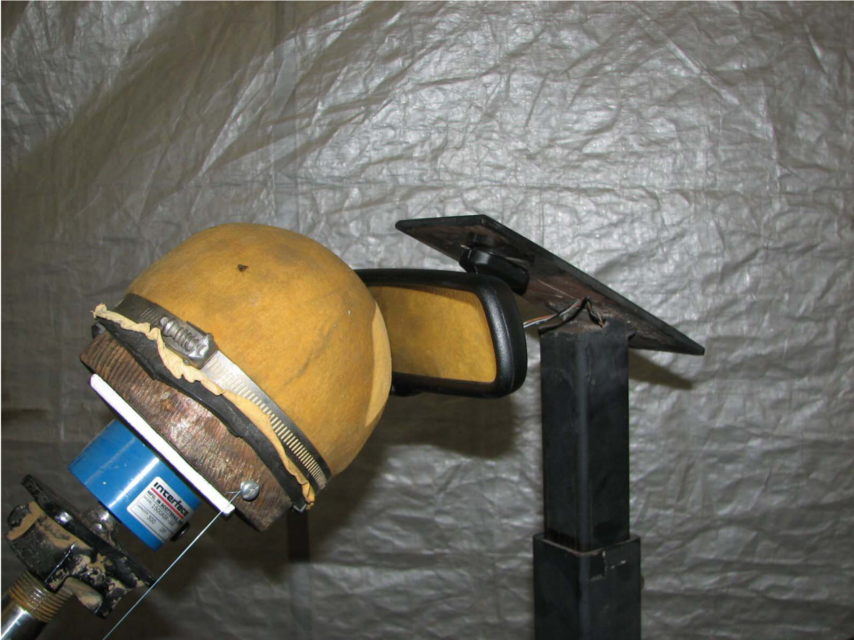
FIGURE 13:CLOSE-UP OF MIRROR BREAK- AWAY TEST
