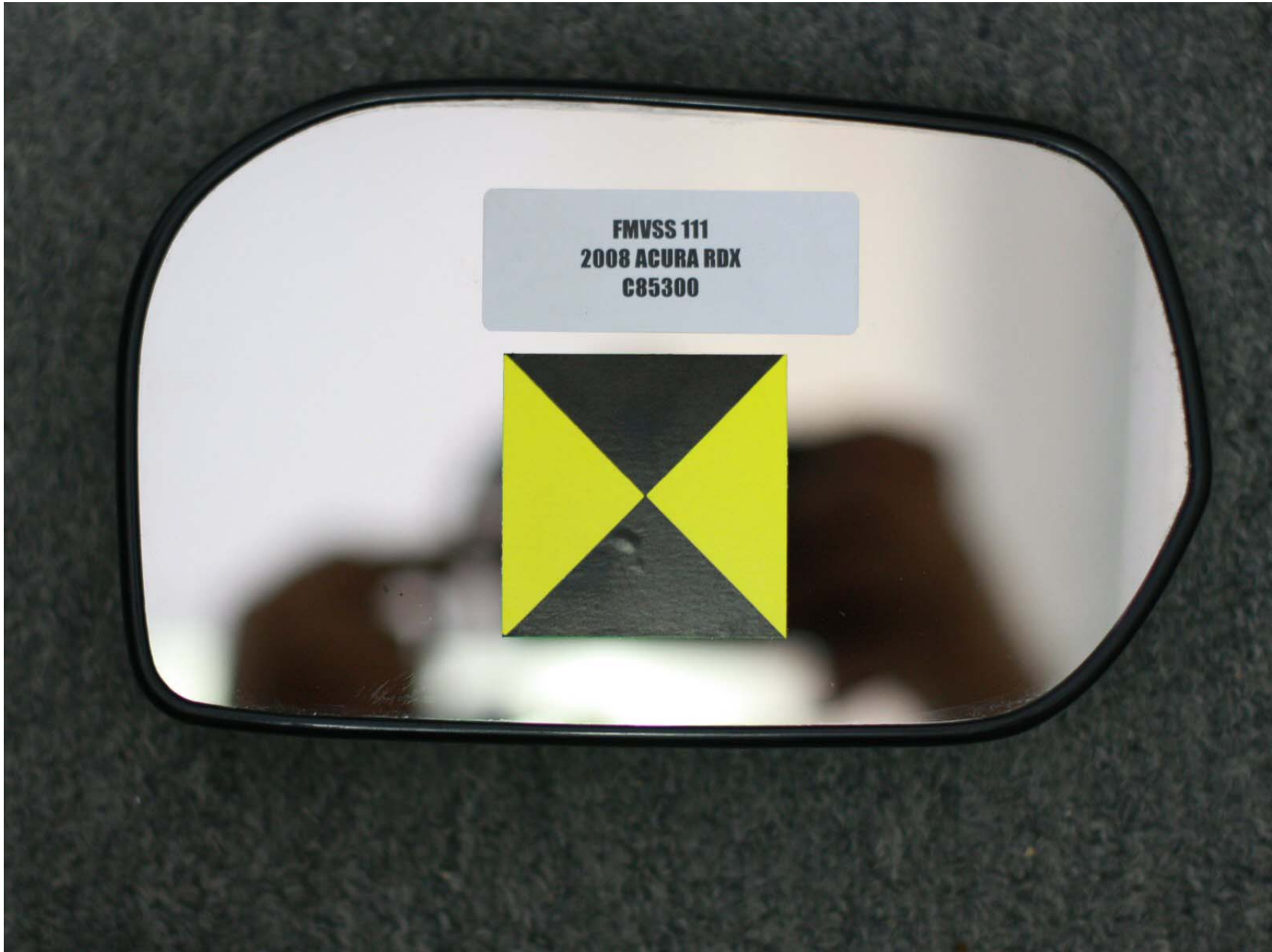
FIGURE 15: MIRROR SET-UP FOR AREA MEASUREMENT
