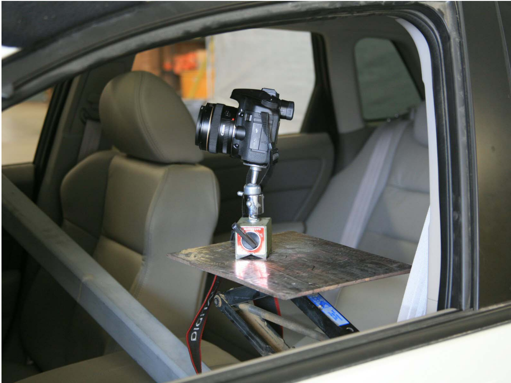
FIGURE 11:CAMERA SET-UP FOR PHOTOGRAPHING REFERENCE BOARD
