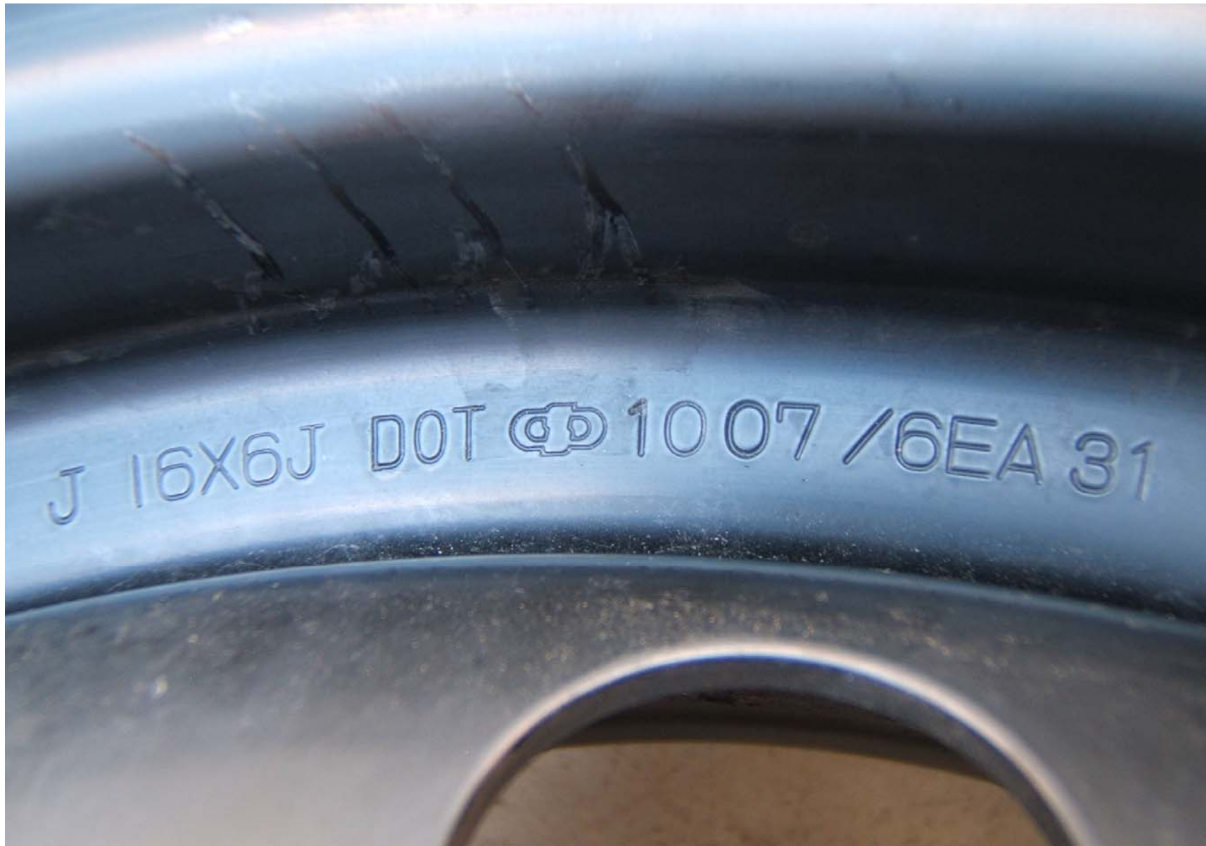
FIGURE 5.12 RIM SHOWING LETTER DESIGNATION FOR SOURCE OF PUBLISHED DIMENSIONS, SIZE, DOT SYMBOL, MANUFACTURER'S SYMBOL, AND DATE OF MANUFACTURE
