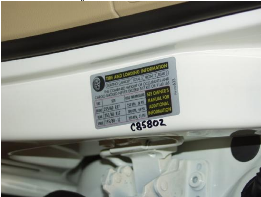
Figure A-2: Vehicle Tire Placard
