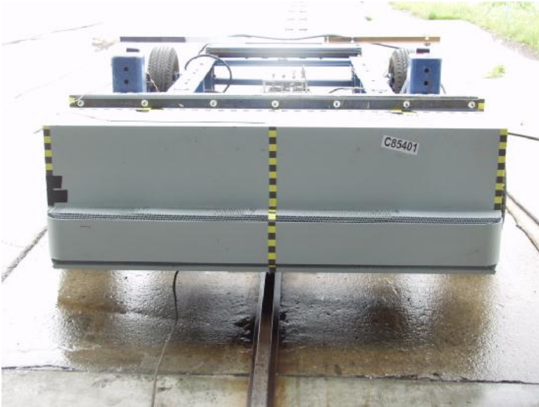
Figure A-19: Pre-Test MDB Front View
