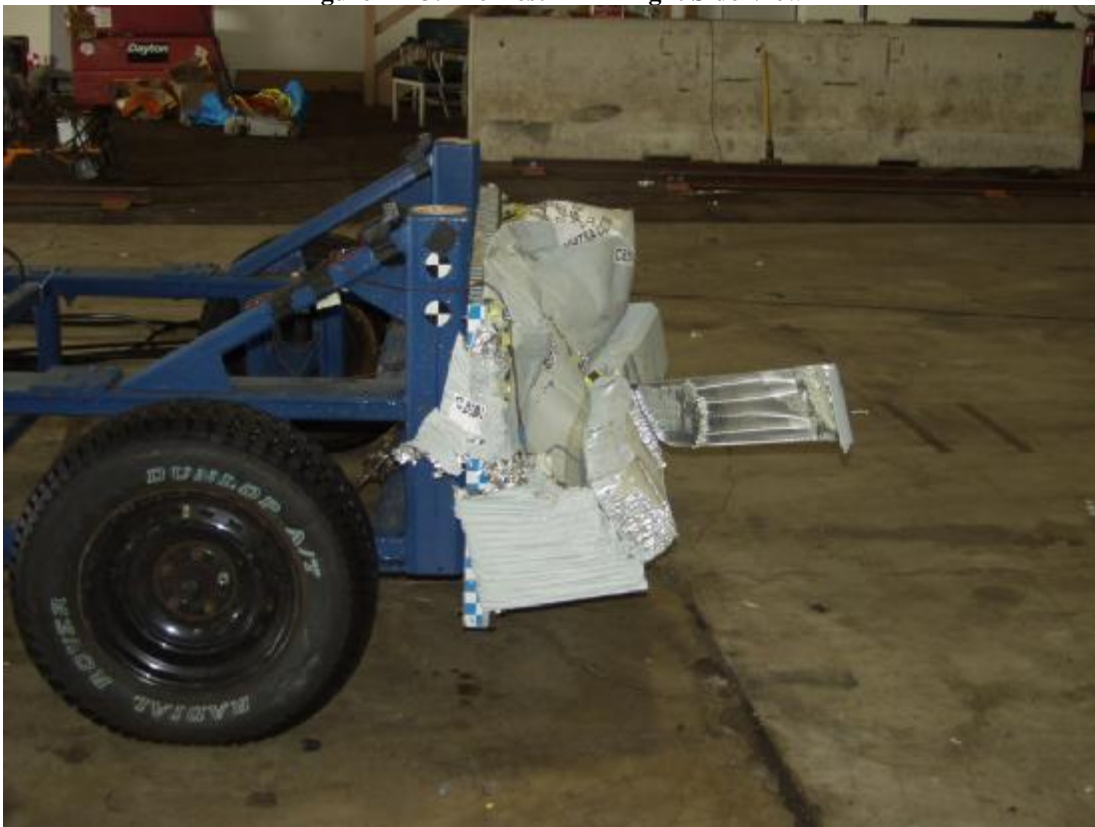
Figure A-24: Post-Test MDB Right Side View
