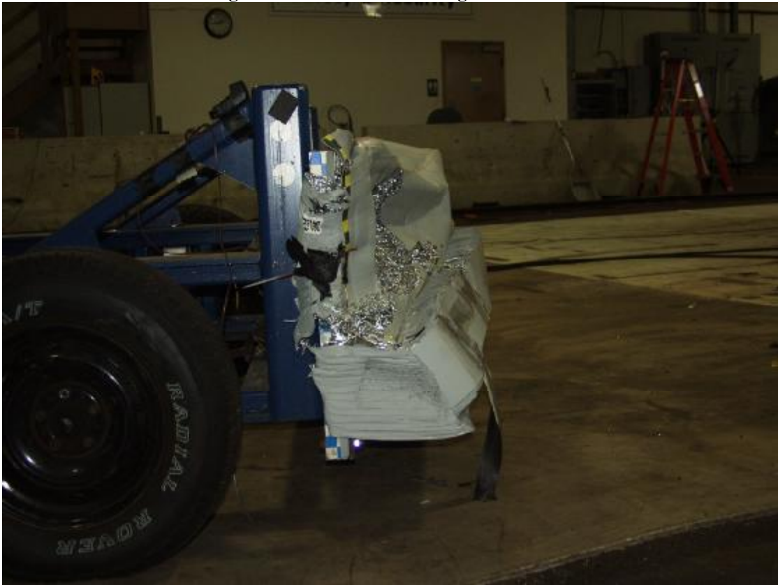
Figure A-28: Post-Test MDB Right Side View
