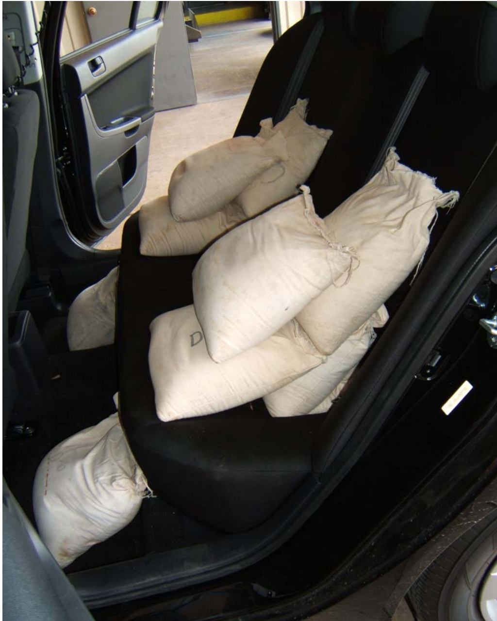
FIGURE 5.14 VEHICLE REAR SEAT BALLAST FOR UVW + VCW LOAD
