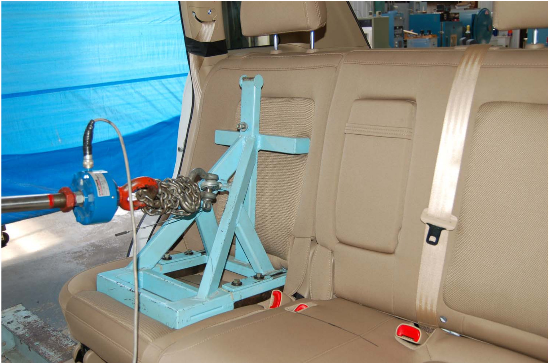
FIGURE 5.42 PRE-TEST ROW 2, RIGHT SIDE WITH SFAD 2
