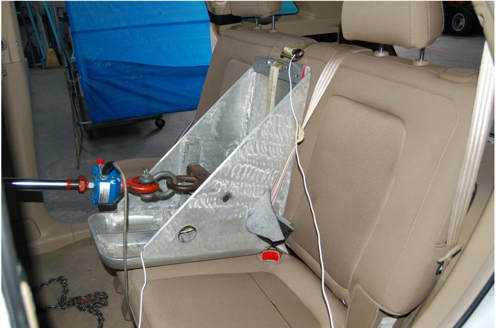
FIGURE 5.44 PRE-TEST ROW 2, CENTER WITH SFAD 1
