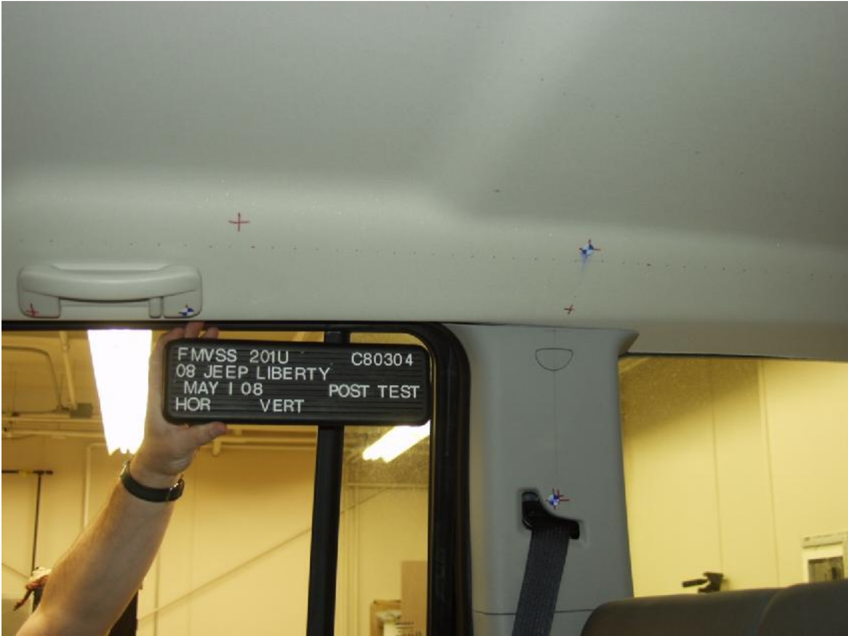
Figure A-29 : POST-TEST PASSENGER SIDE OTHER PILLAR
