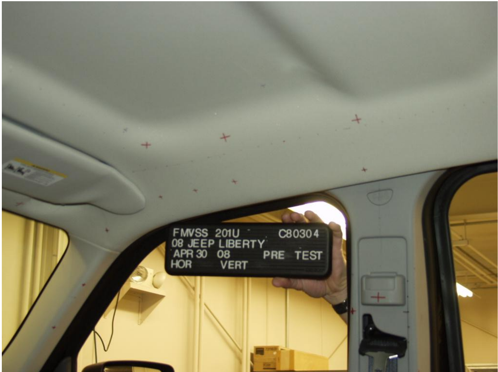
Figure A-15 : PRE-TEST PASSENGER SIDE SIDE RAIL
