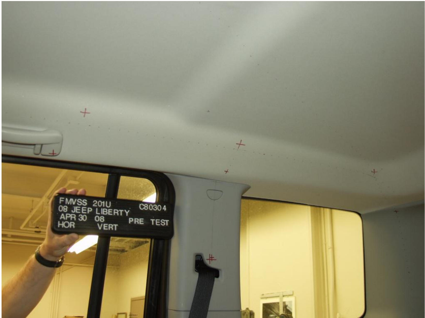
Figure A-17 : PRE-TEST PASSENGER SIDE OTHER PILLAR
