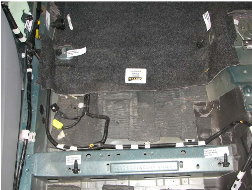
FIGURE 68. Floor Pan Anchors, P2 Overall, Post-Test
