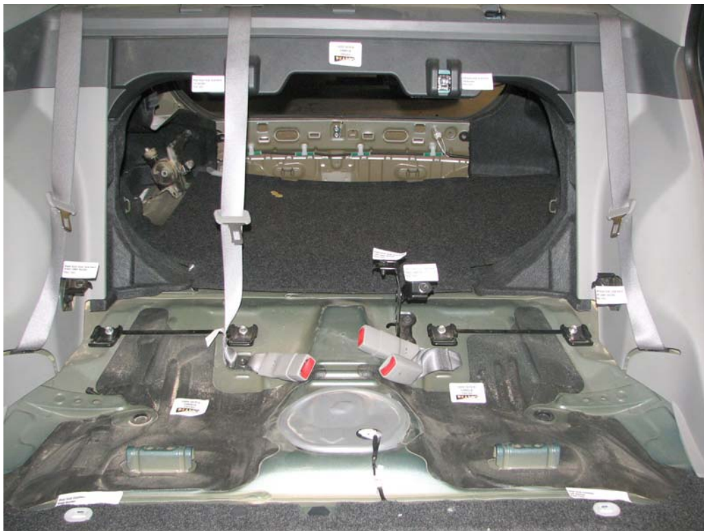
FIGURE 96. Floor Pan Anchors, P3 & P4 Overall, Post-Test
