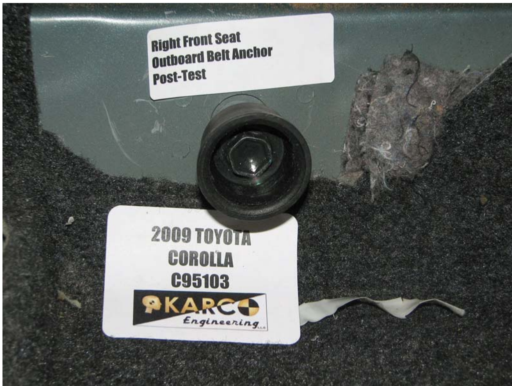
FIGURE 92. Shoulder Belt Anchor, P2, Post-Test
