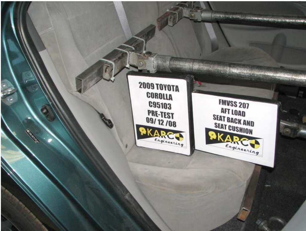
FIGURE 37. Aft Load on Seat Back and Seat Cushion, P3, Pre-Test
