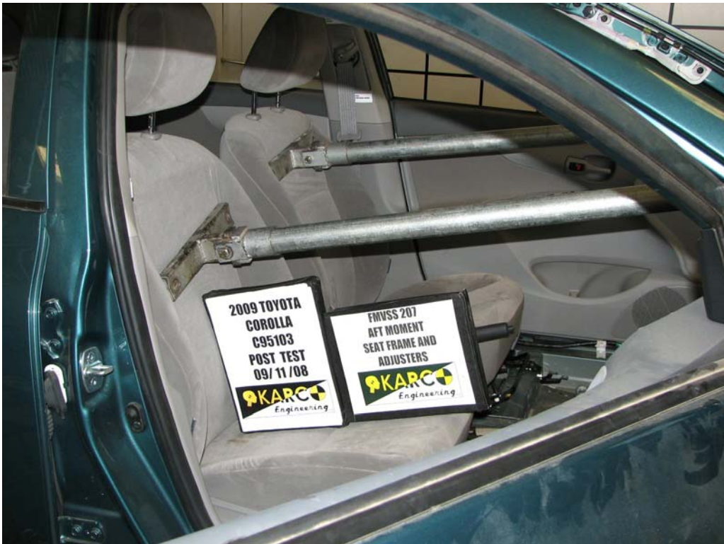
FIGURE 14. Aft Moment on Seat Back, P2, Post-Test
