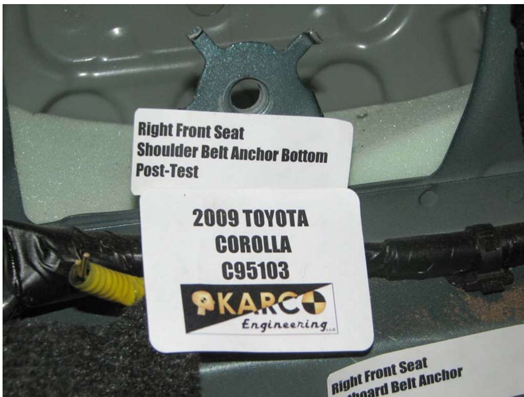
FIGURE 90. Shoulder Belt Anchor, P2, Post-Test
