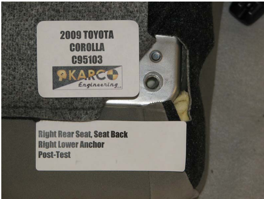
FIGURE 124. Seat Back Anchor, P4, Post-Test
