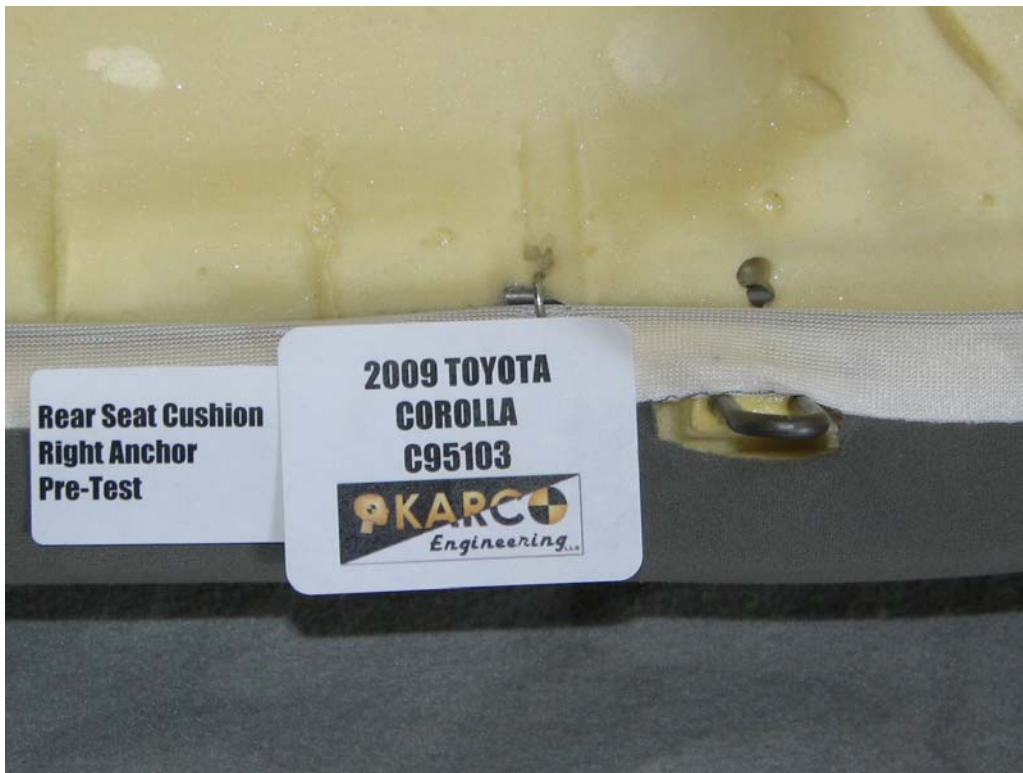
FIGURE 129. Seat Cushion Anchor, P3, Pre-Test
