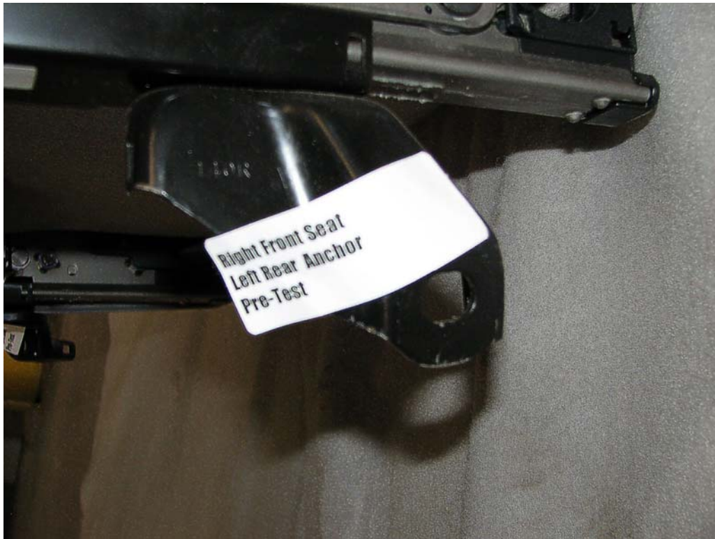
FIGURE 81. Seat Anchor, P2, Pre-Test
