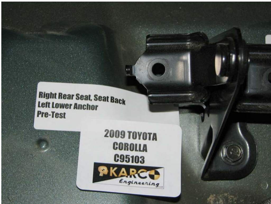
FIGURE 117. Seat Anchor, P4, Pre-Test
