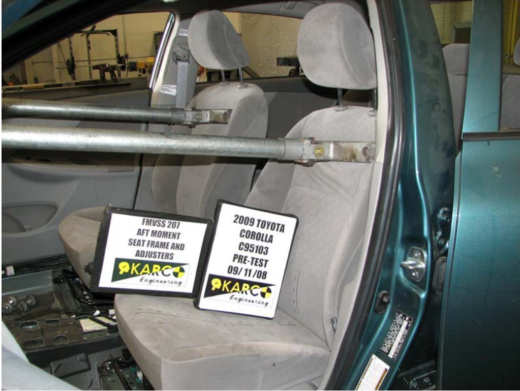
FIGURE 11. Aft Moment on Seat Back, P1, Pre-Test
