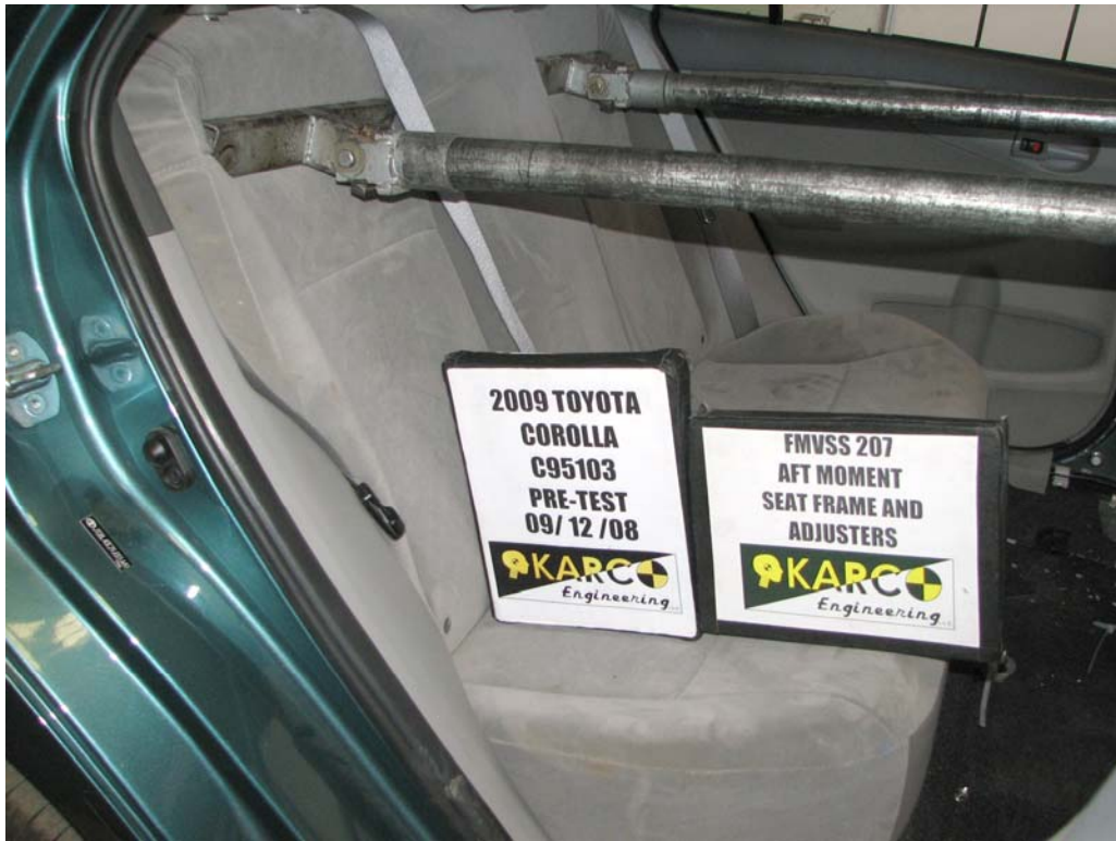
FIGURE 29. Aft Moment Seat Back (Incorrect Sign), P3, Pre-Test
