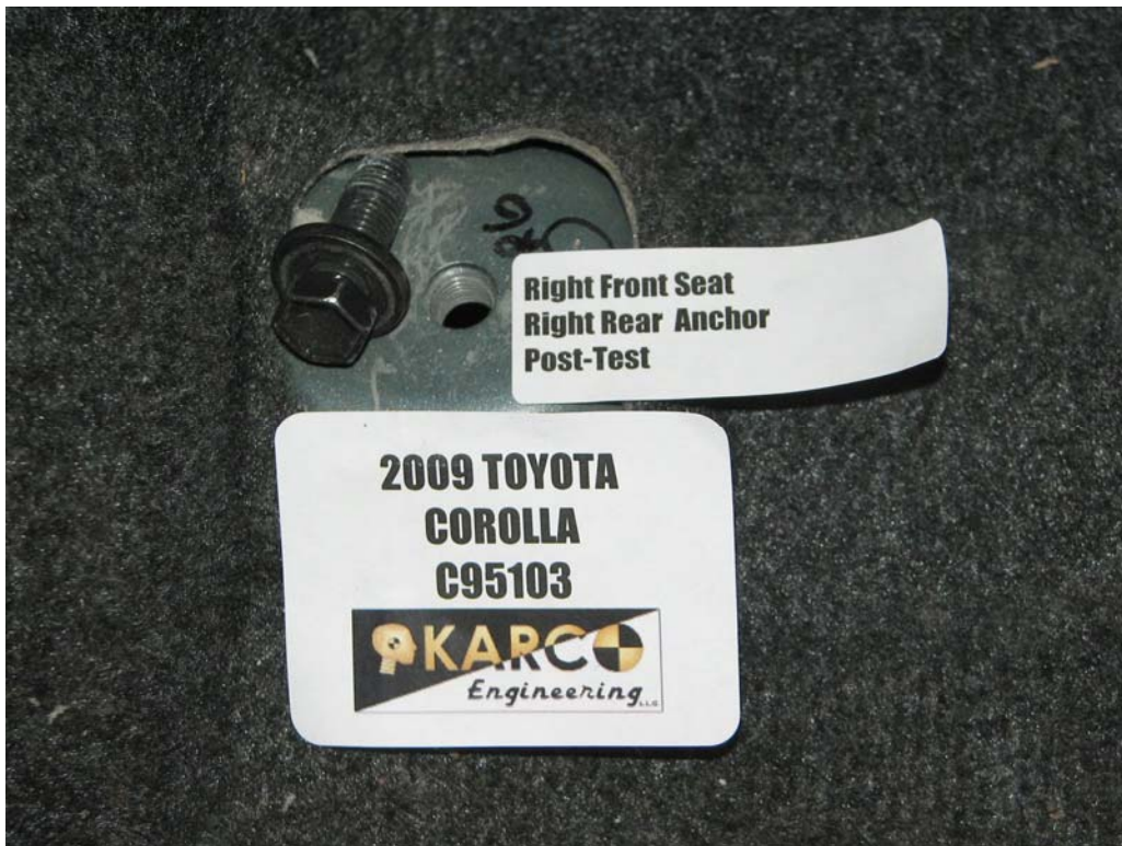
FIGURE 84. Floor Pan Anchor, P2, Post-Test
