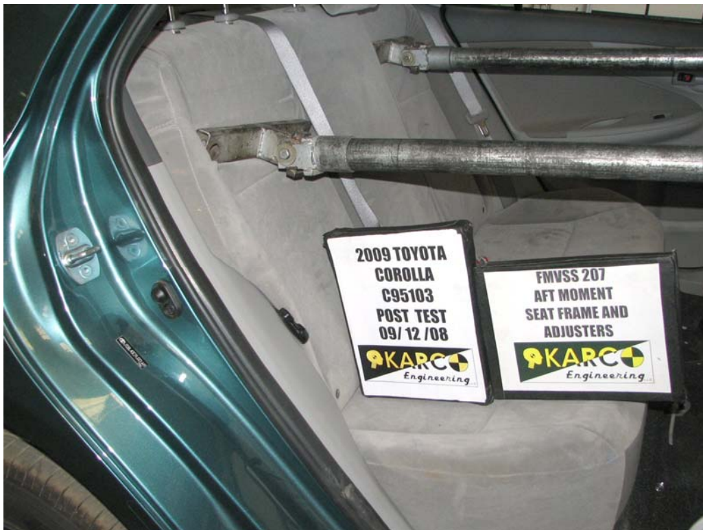
FIGURE 30. Aft Moment Seat Back (Incorrect Sign), P3, Post-Test
