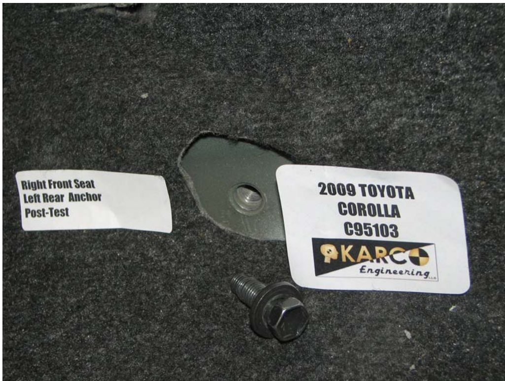
FIGURE 80. Floor Pan Anchor, P2, Post-Test
