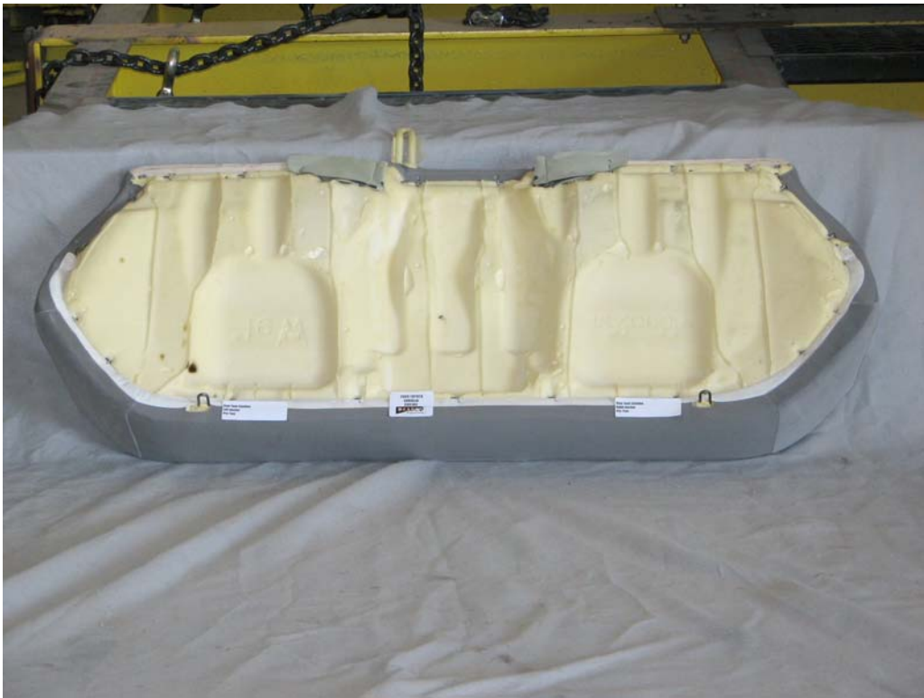
FIGURE 125. Seat Cushion Anchors, P3 & P4 Overall, Pre-Test
