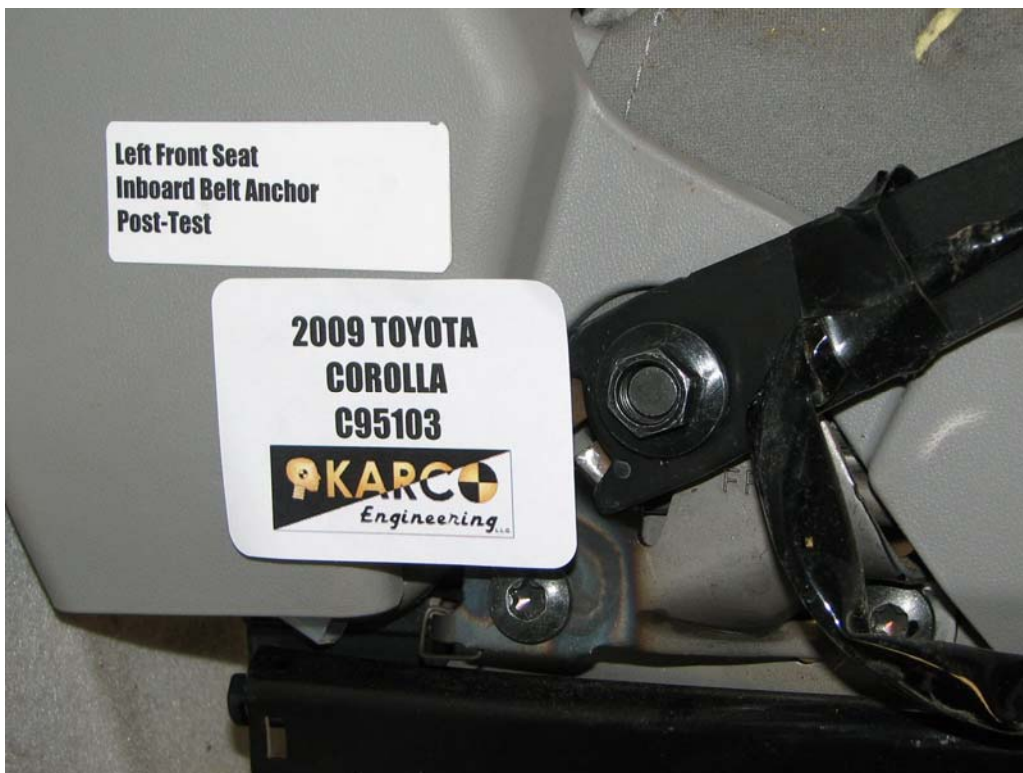
FIGURE 66. Belt Anchor, P1, Post-Test
