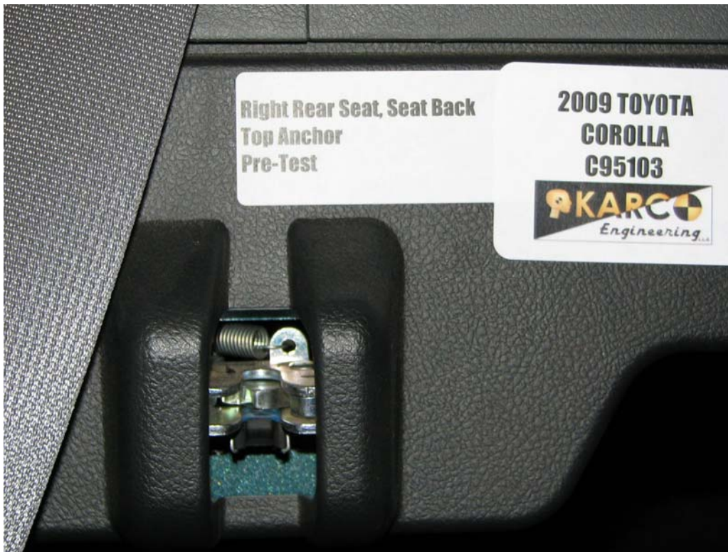
FIGURE 113. Seat Anchor, P4, Pre-Test
