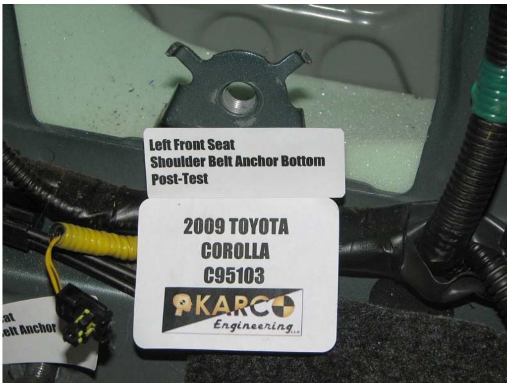
FIGURE 62. Shoulder Belt Anchor, P1, Post-Test
