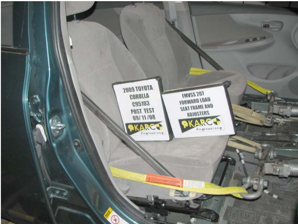
FIGURE 18. Forward Load on Seat Frame and Adjusters, P2, Post-Test
