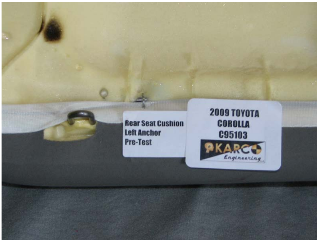
FIGURE 127. Seat Cushion Anchor, P4, Pre-Test
