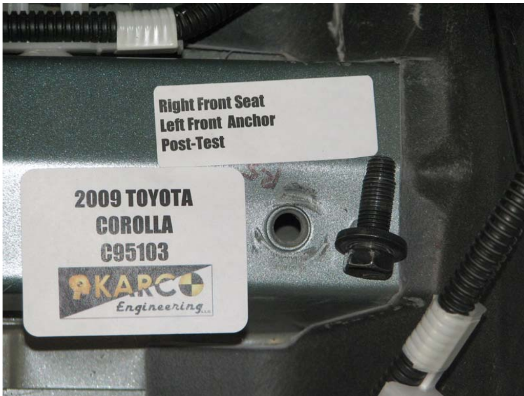
FIGURE 72. Floor Pan Anchor, P2, Post-Test
