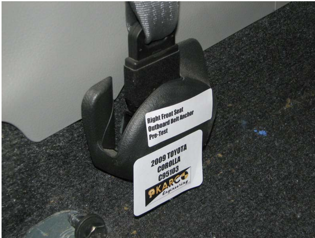
FIGURE 91. Shoulder Belt Anchor, P2, Pre-Test
