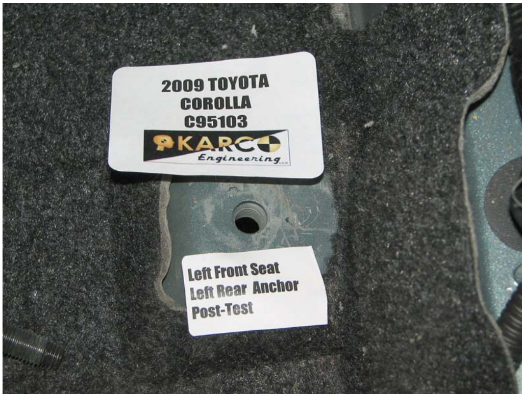
FIGURE 52. Floor Pan Anchor, P1, Post-Test
