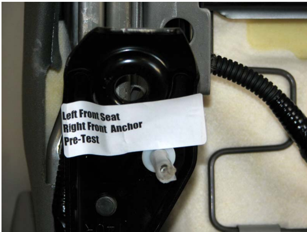
FIGURE 49. Seat Anchor, P1, Pre-Test
