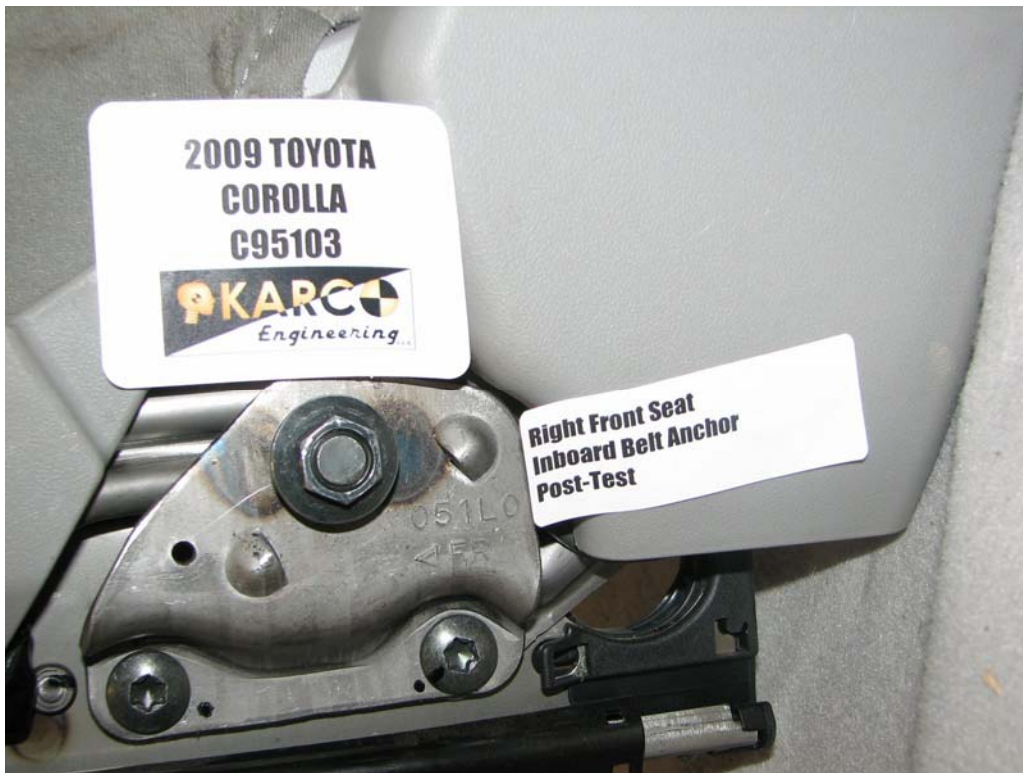
FIGURE 94. Belt Anchor, P2, Post-Test
