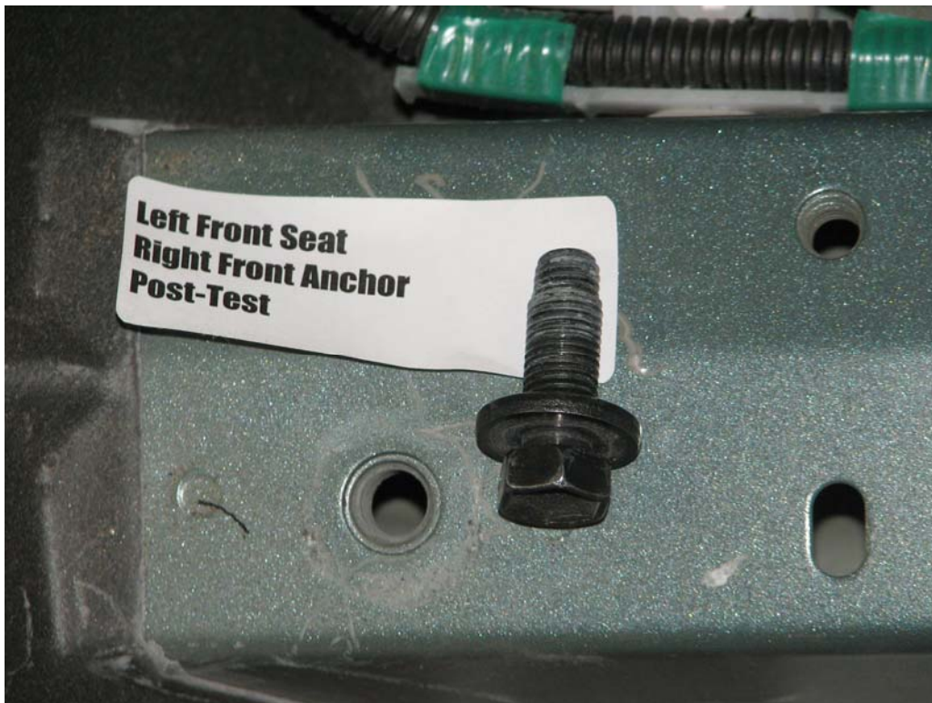
FIGURE 48. Floor Pan Anchor, P1, Post-Test
