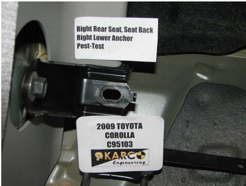
FIGURE 122. Seat Back Anchor, P4, Post-Test
