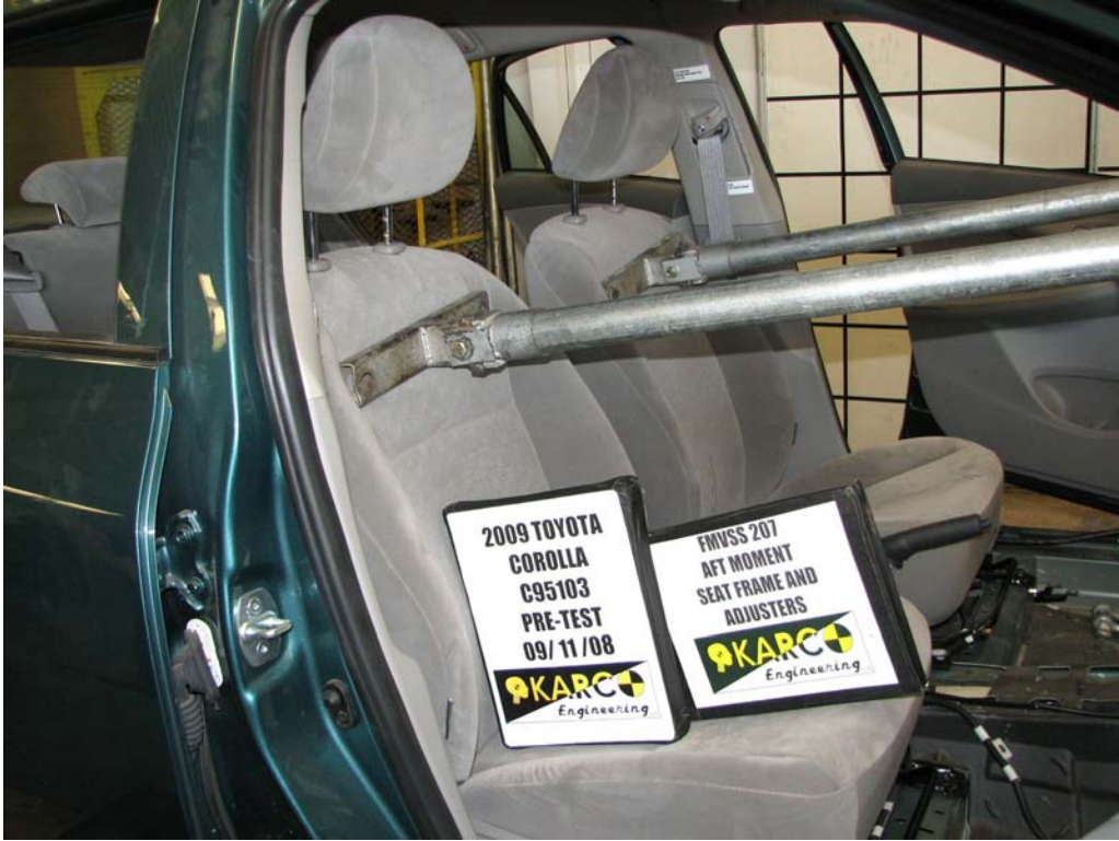
FIGURE 13. Aft Moment on Seat Back, P2, Pre-Test
