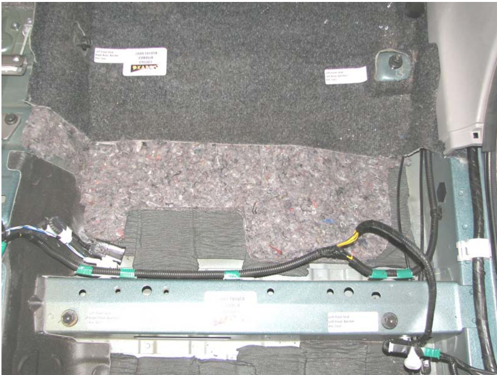
FIGURE 39. Floor Pan Anchors, P1 Overall, Pre-Test
