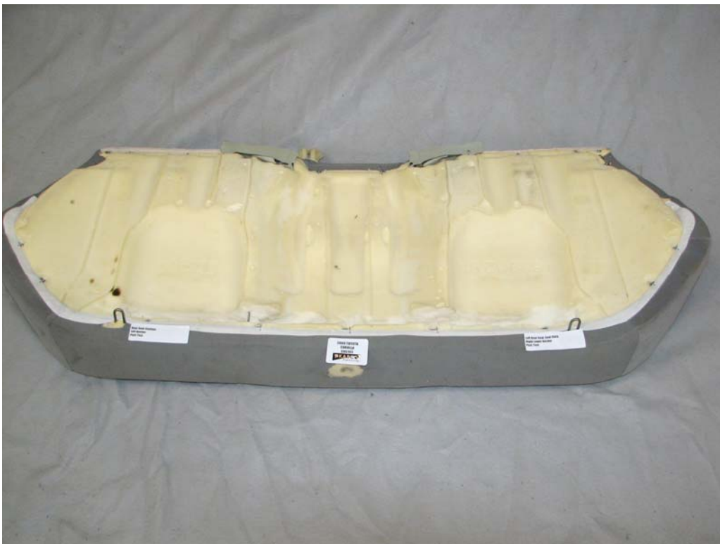
FIGURE 126. Seat Cushion Anchors, P3 & P4 Overall, Post-Test
