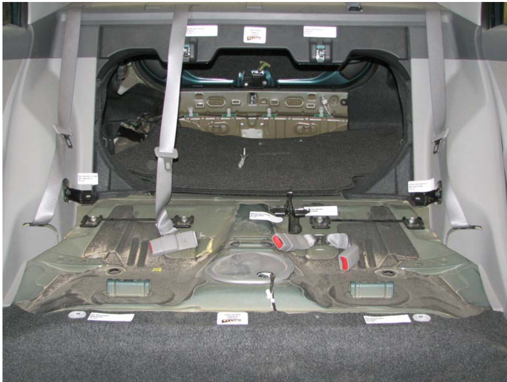
FIGURE 95. Floor Pan Anchors, P3 & P4 Overall, Pre-Test
