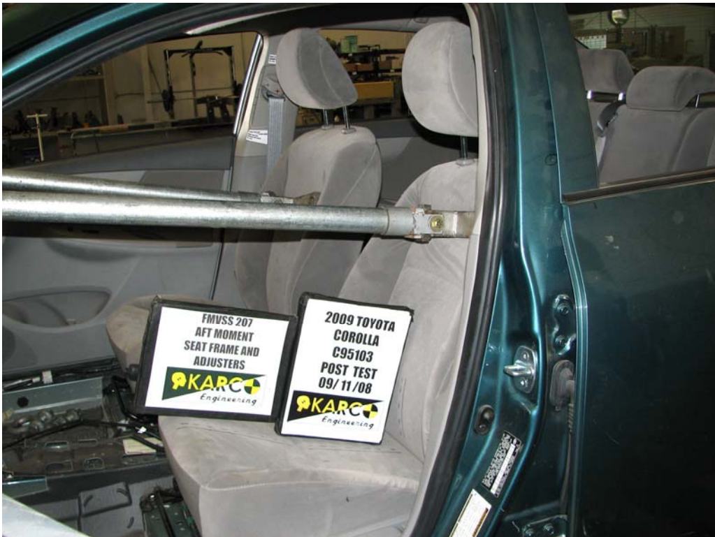
FIGURE 12. Aft Moment on Seat Back, P1, Post-Test
