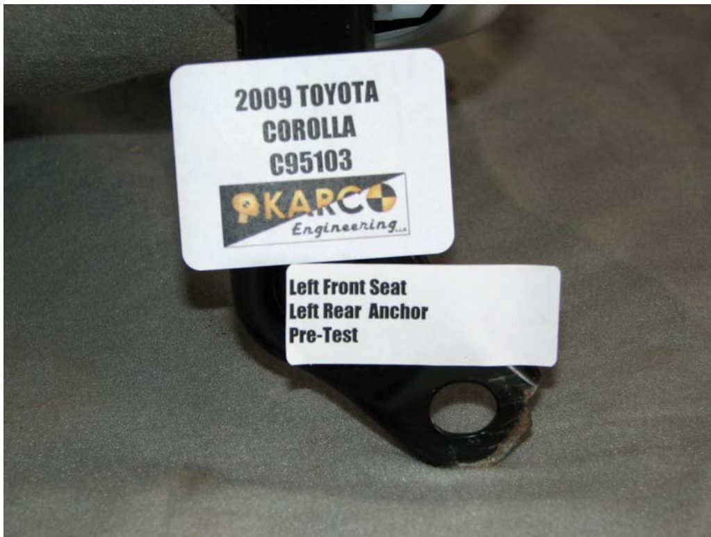
FIGURE 53. Seat Anchor, P1, Pre-Test
