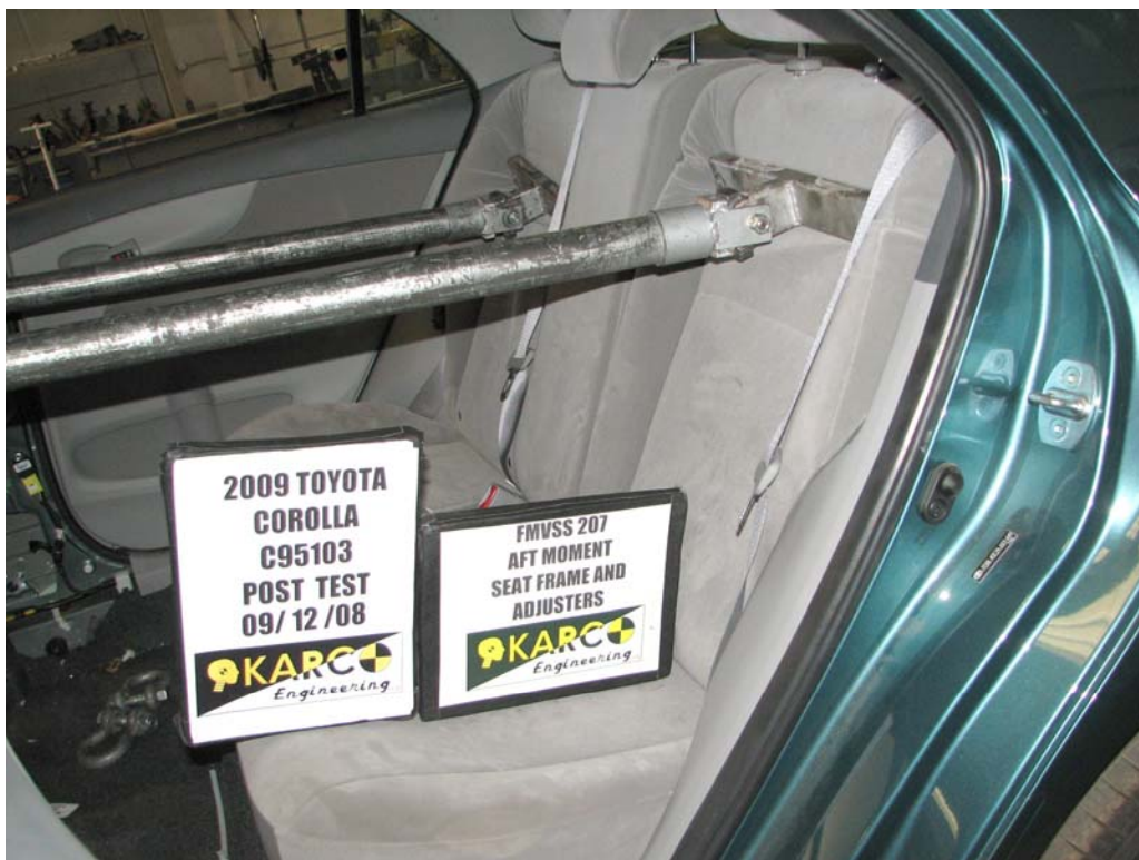
FIGURE 28. Aft Moment Seat Back (Incorrect Sign), P4, Post-Test
