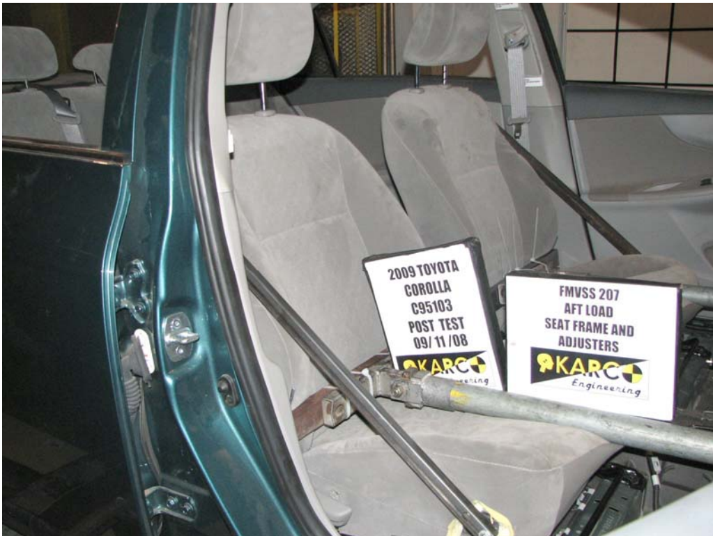
FIGURE 22. Aft Load on Seat Frame and Adjusters, P2, Post-Test
