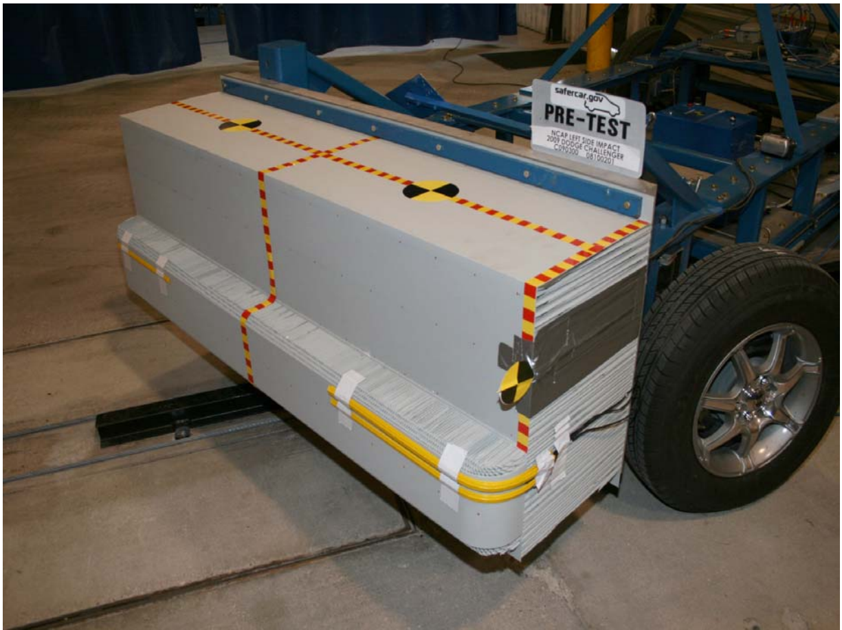
Pre-Test Left Side View of Deformable Barrier
