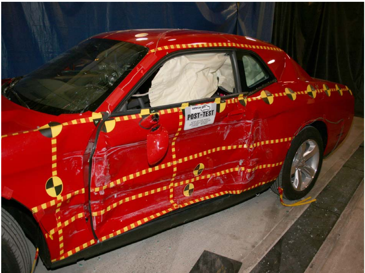
Post-Test Front \frac{3}{4} View of Left Side Doors
