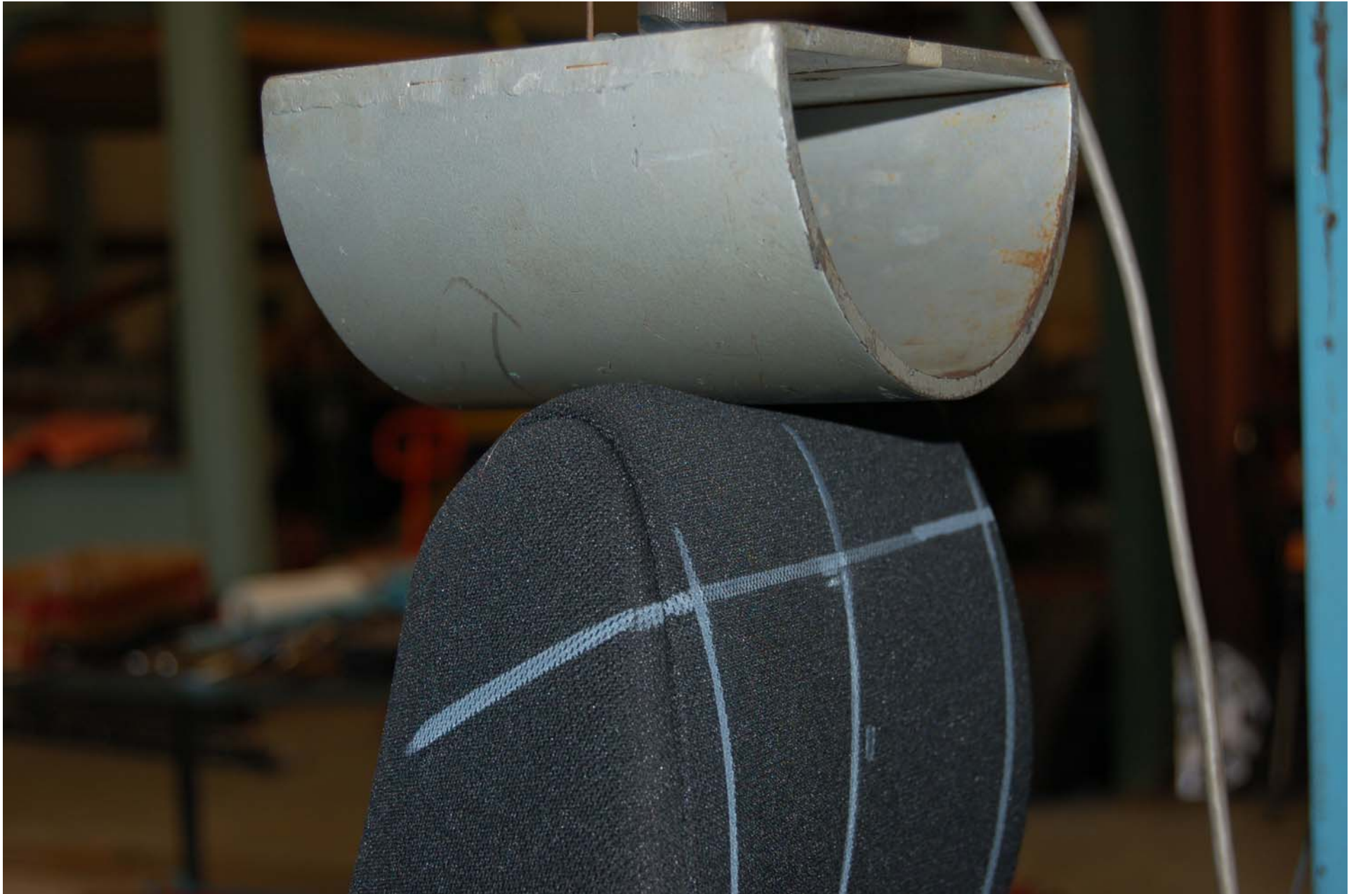
FIGURE 5.27 HEAD RESTRAINT WITH 50 N LOAD FOR HEIGHT RETENTION
