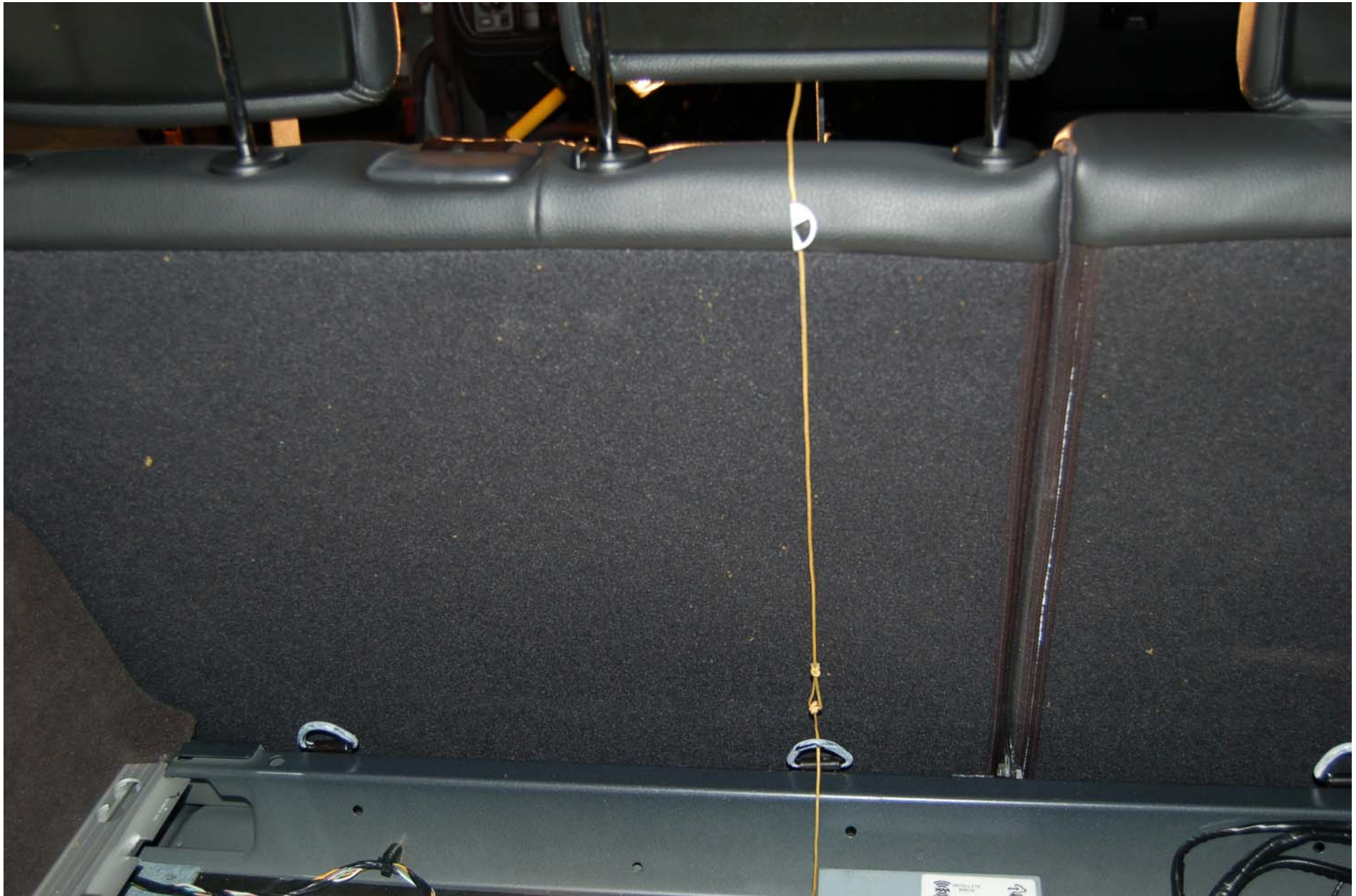
FIGURE 5.25 ROW 2, CENTER, TOP TETHER ROUTING
