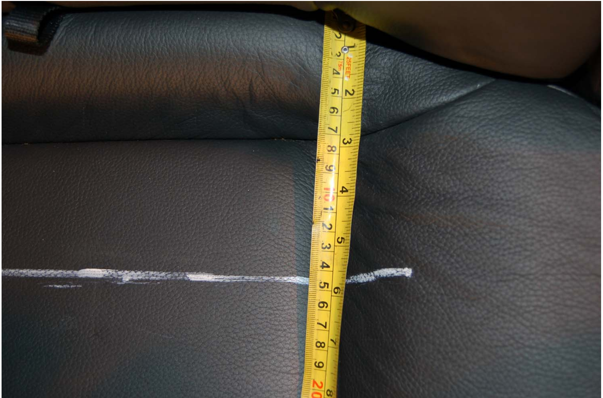
FIGURE 5.33 ROW 2, LEFT SIDE, OUTBOARD SRP MEASUREMENT
