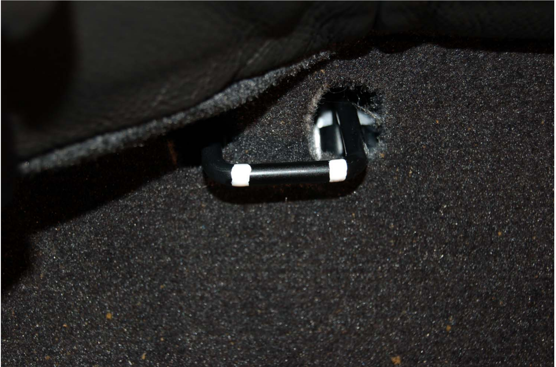
FIGURE 5.13 ROW 2, RIGHT SIDE, OUTBOARD LOWER ANCHOR, PRE-TEST
