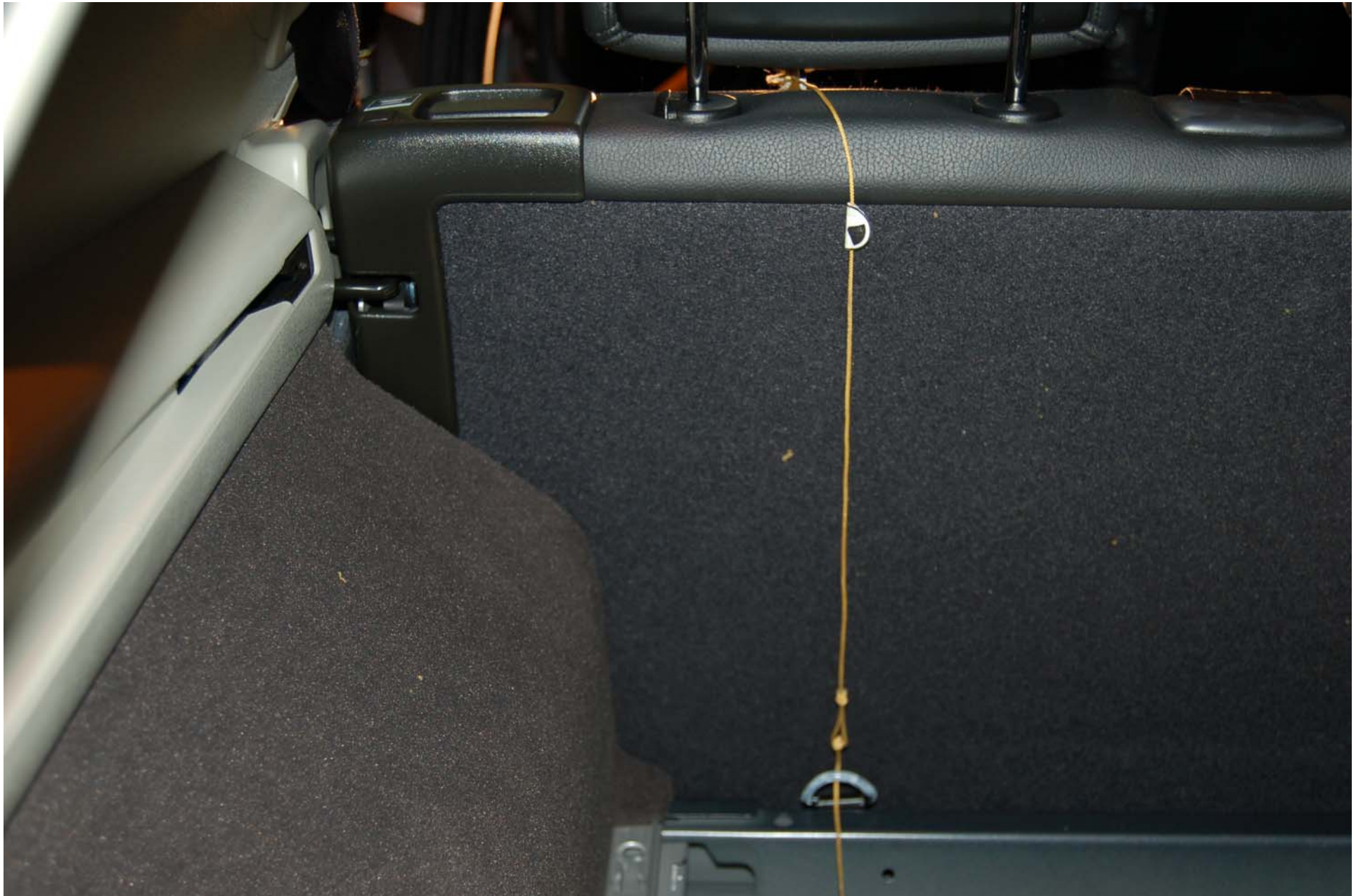
FIGURE 5.19 ROW 2, LEFT SIDE, TOP TETHER ROUTING
