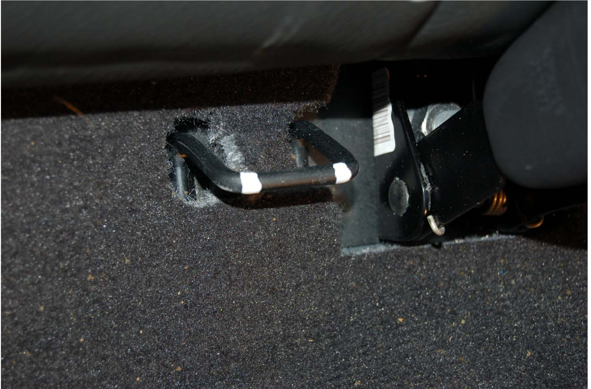
FIGURE 5.12 ROW 2, RIGHT SIDE, INBOARD LOWER ANCHOR, PRE-TEST
