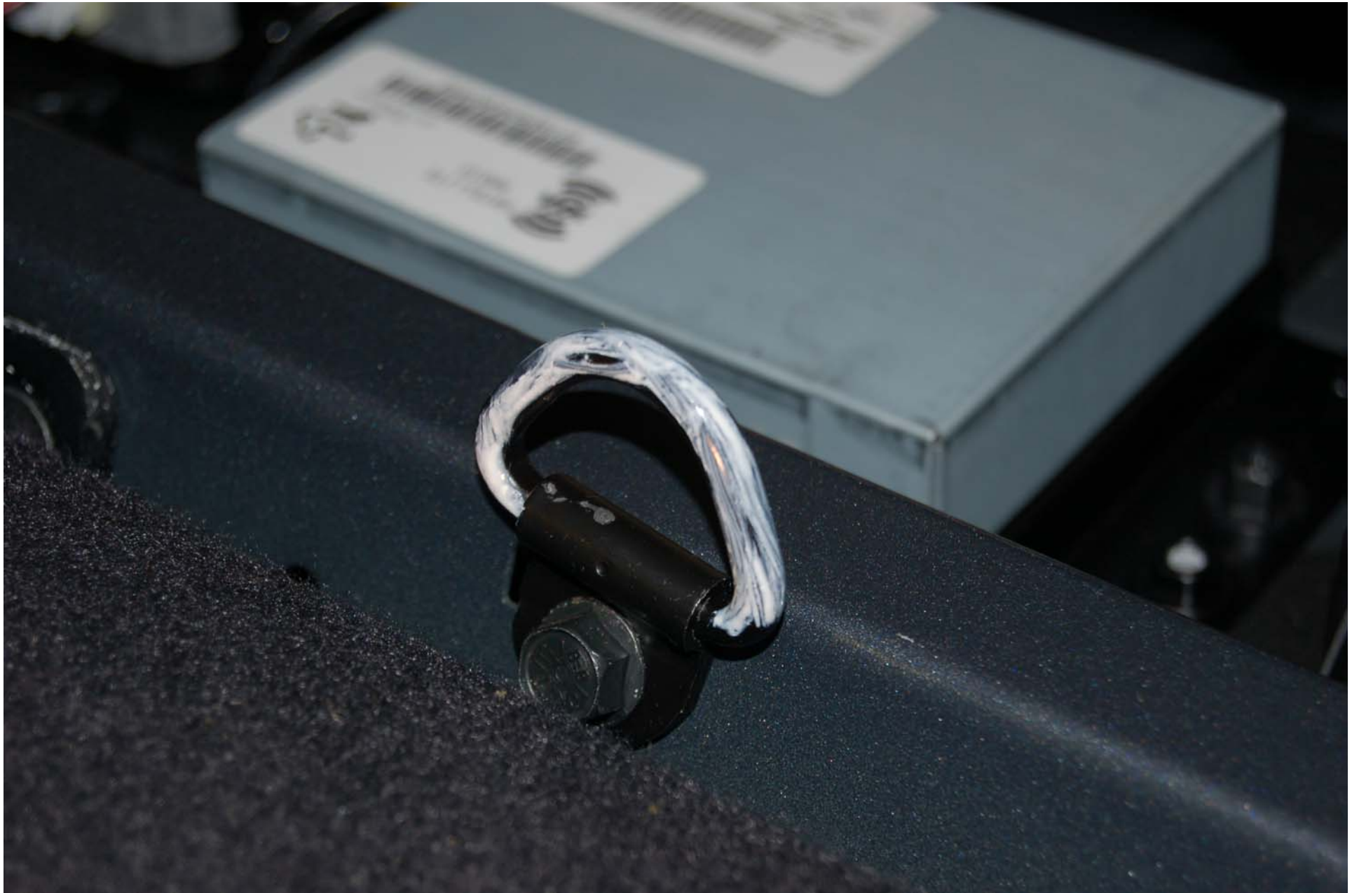
FIGURE 5.11 ROW 2, CENTER, TOP TETHER ANCHOR, PRE-TEST
