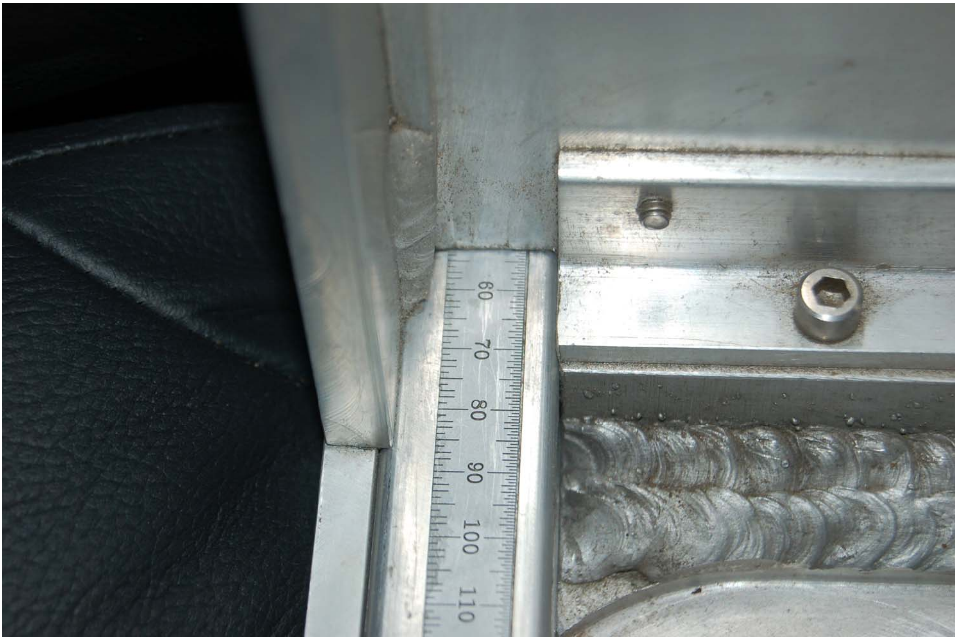
FIGURE 5.26 ROW 2, RIGHT SIDE, OUTBOARD CRF MEASUREMENT
