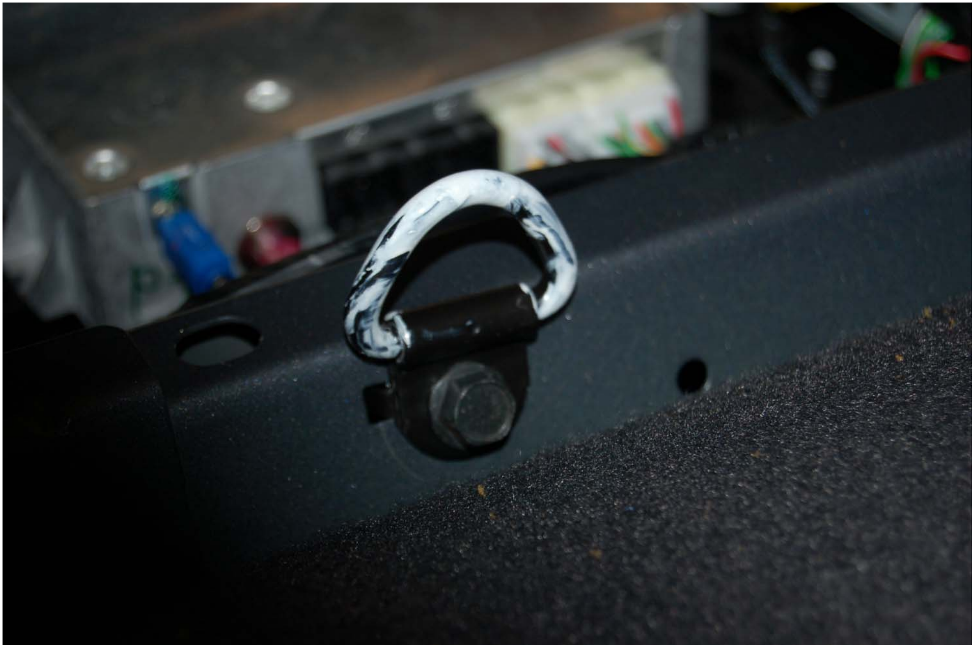
FIGURE 5.14 ROW 2, RIGHT SIDE, TOP TETHER ANCHOR, PRE-TEST
