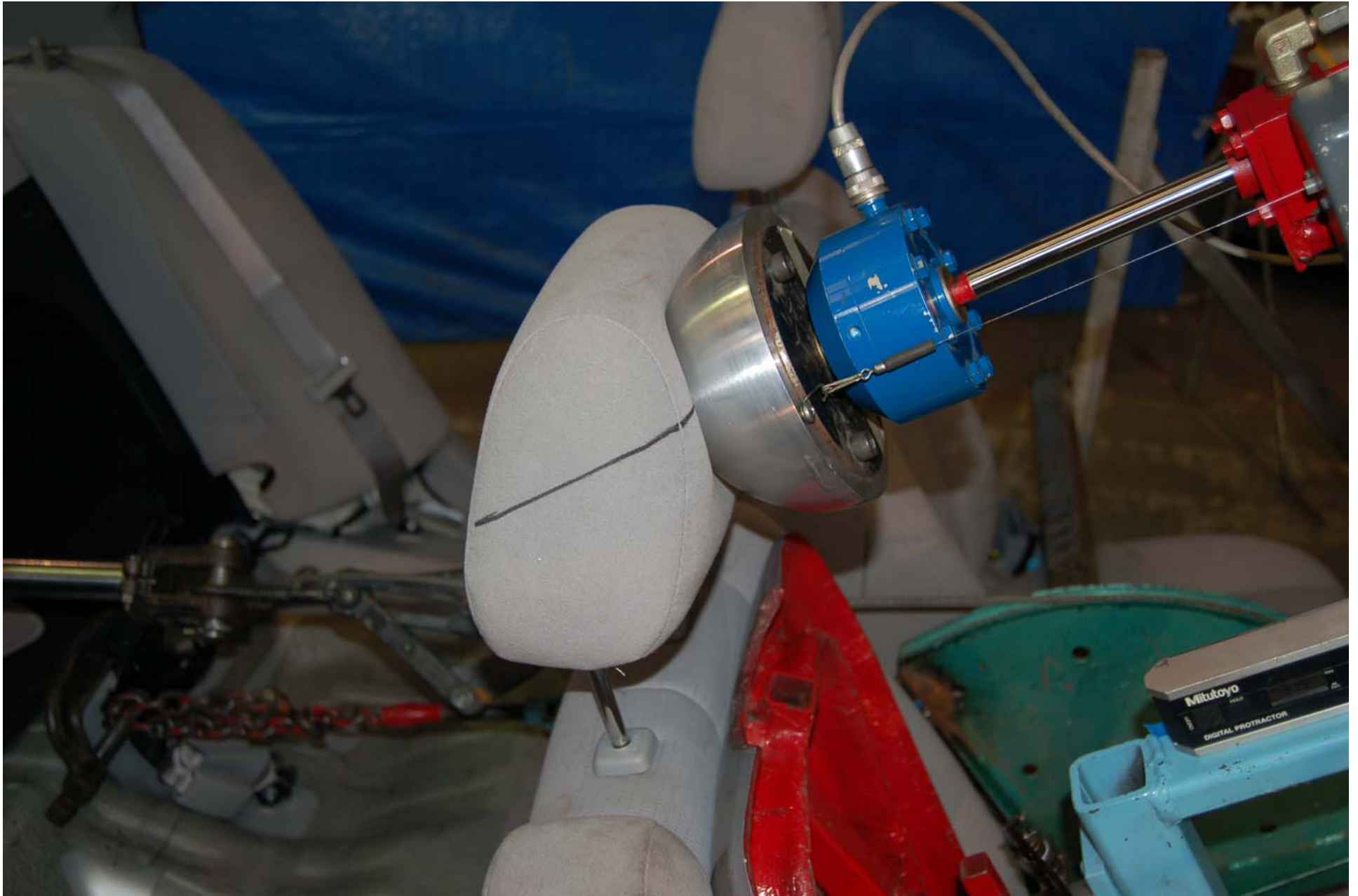
FIGURE 5.23 HEAD RESTRAINT WITH 373 Nm LOAD
