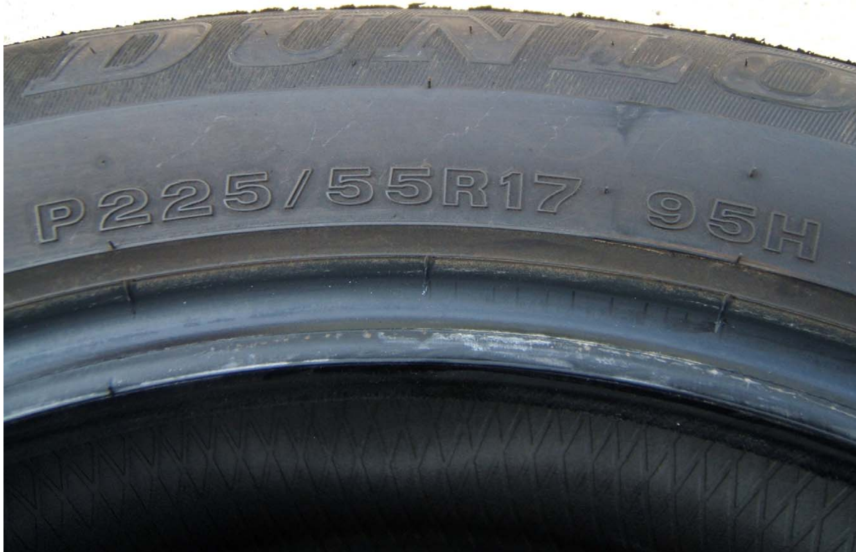
FIGURE 5.6 TIRE SHOWING SIZE AND LOAD INDEX / SPEED RATING
