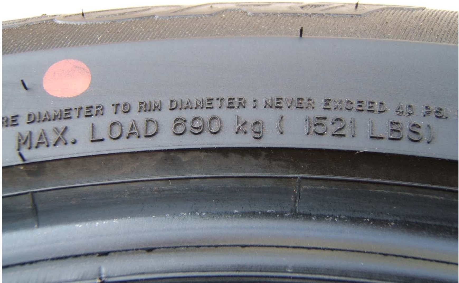
FIGURE 5.8 TIRE SHOWING MAX LOAD RATING
