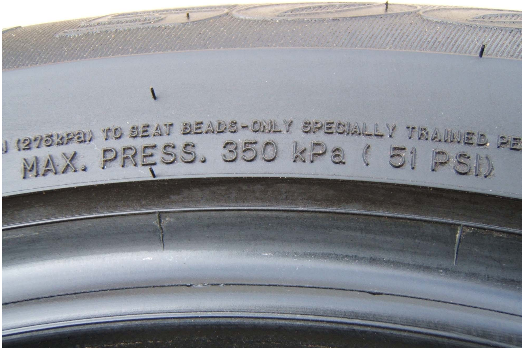
FIGURE 5.9 TIRE SHOWING MAX COLD INFLATION PRESSURE
