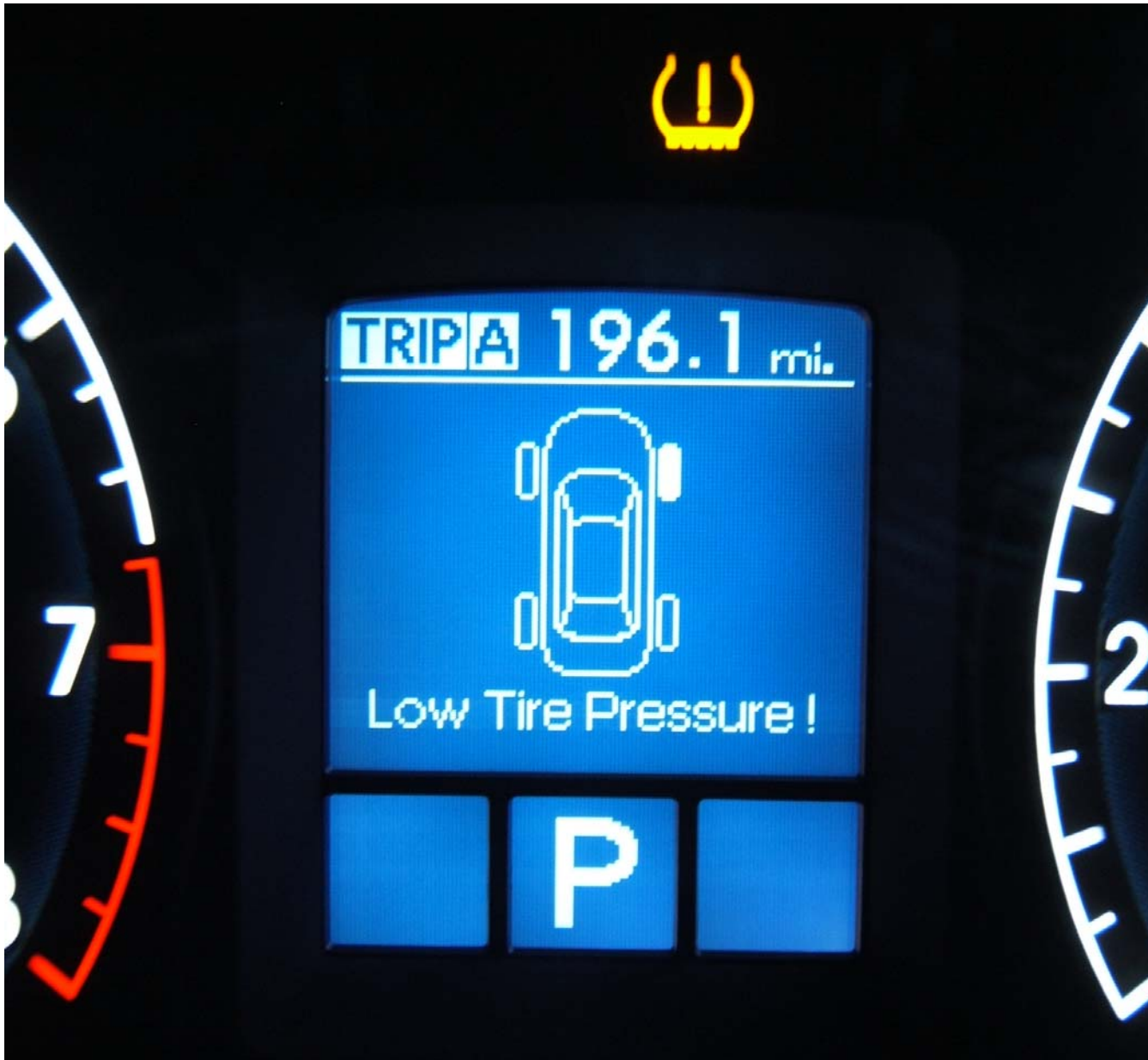
FIGURE 5.14 DISPLAY SHOWING LOW TIRE PRESSURE WARNING
