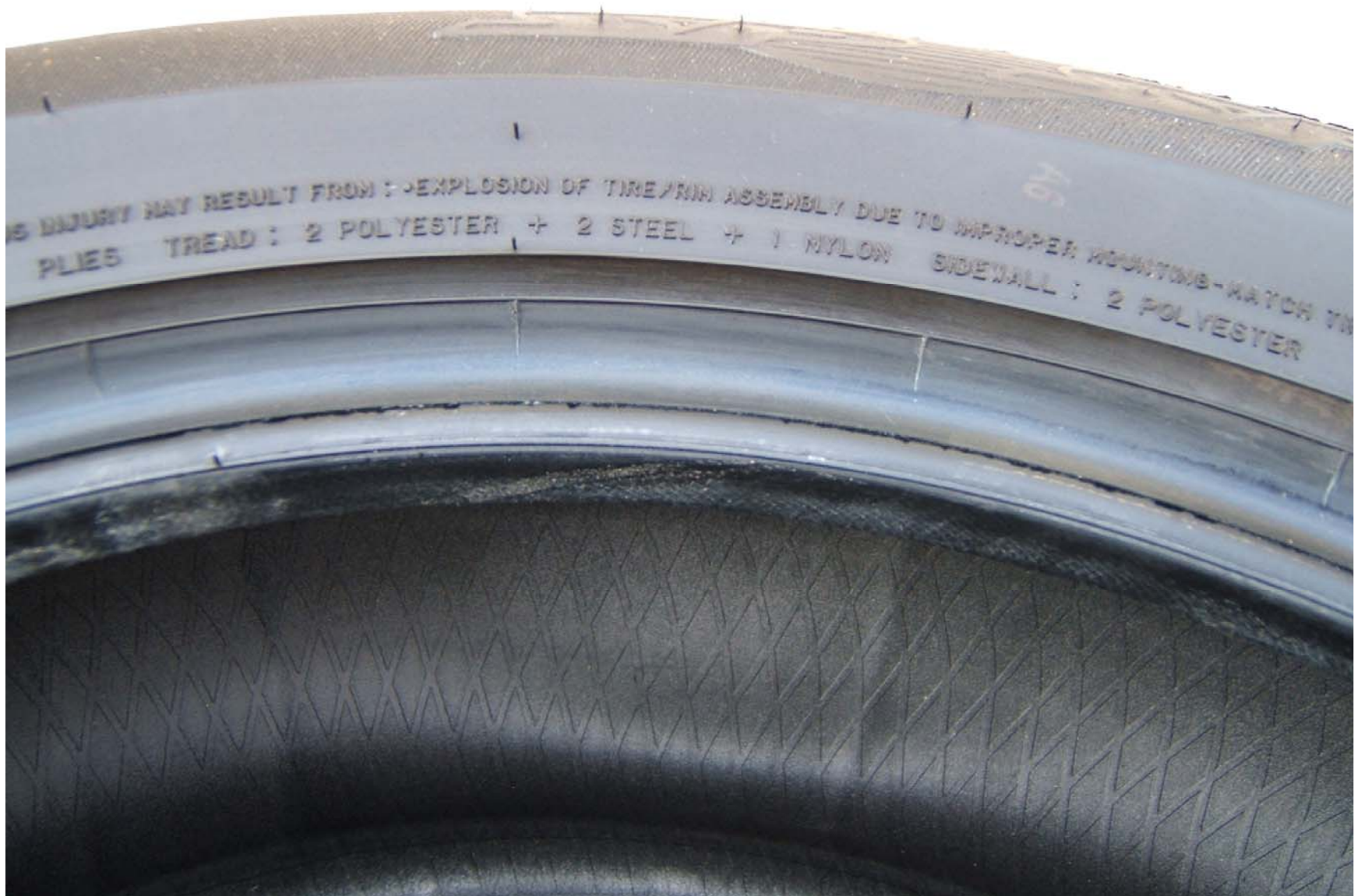
FIGURE 5.10 TIRE SHOWING SIDEWALL / TREAD CONSTRUCTION
