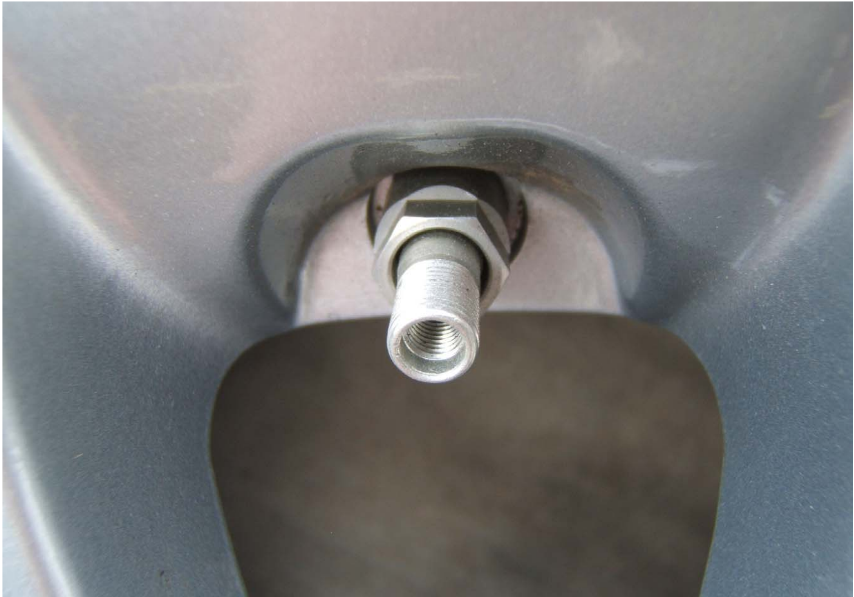
FIGURE 5.11 RIM SHOWING VALVE STEM
