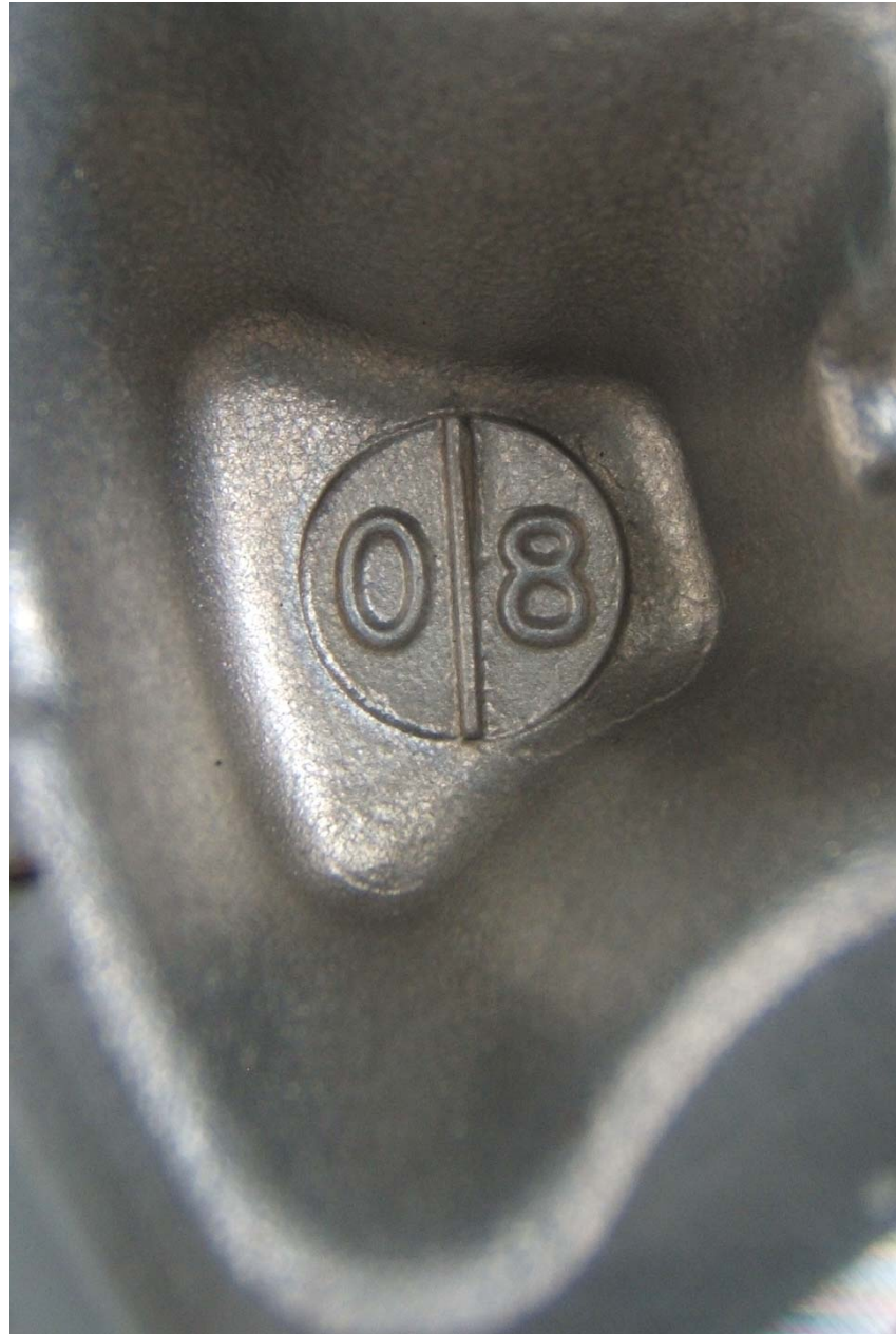
FIGURE 5.15 RIM SHOWING DATE OF MANUFACTURER
