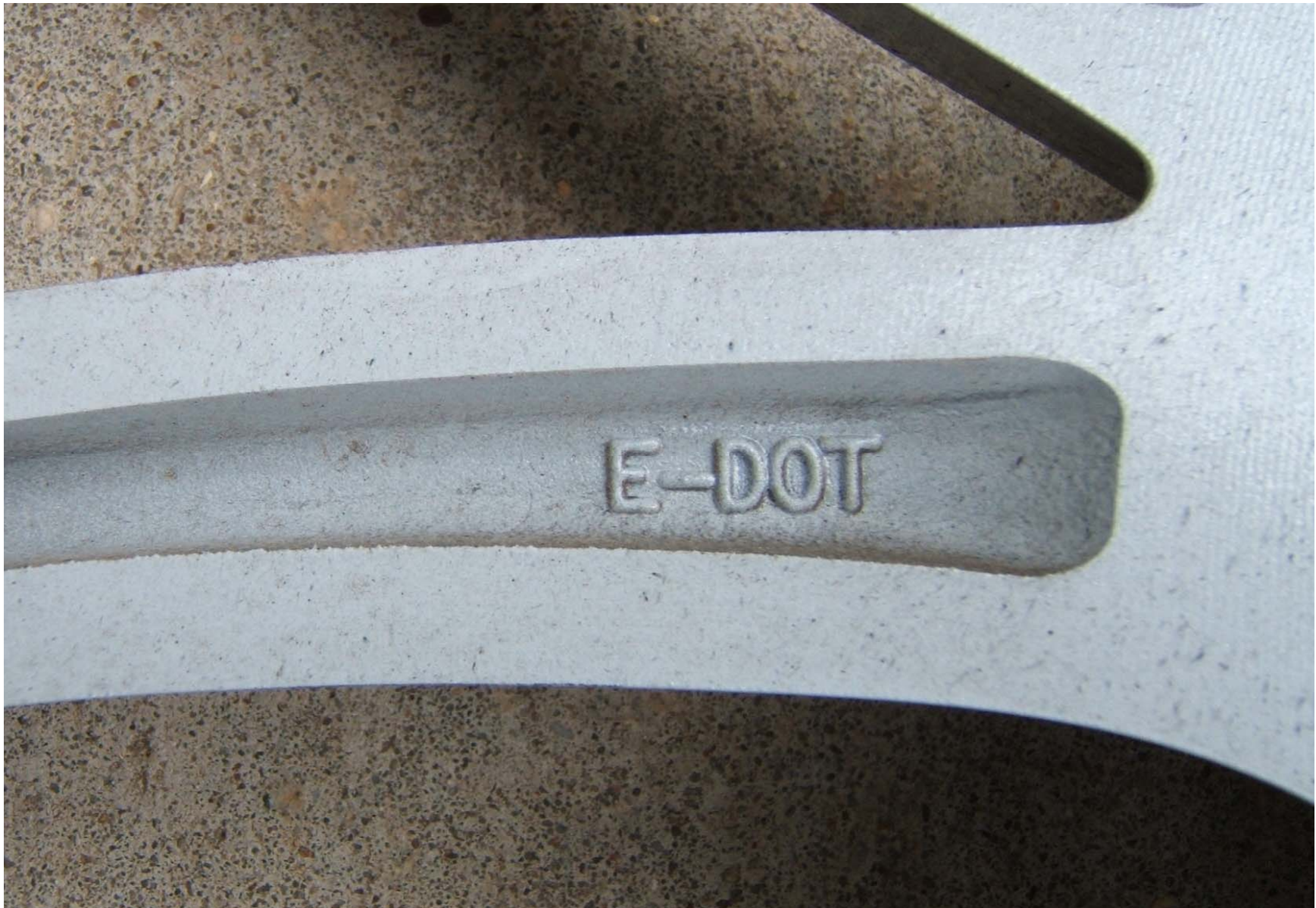
FIGURE 5.13 RIM SHOWING LETTER DESIGNATION FOR SOURCE OF PUBLISHED DIMENSIONS AND DOT SYMBOL
