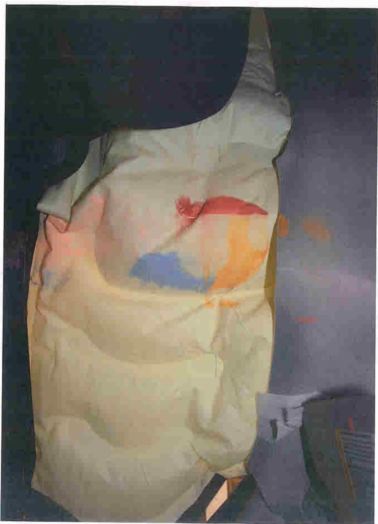
Post-Test Driver Dummy Head Contact (CAB)
