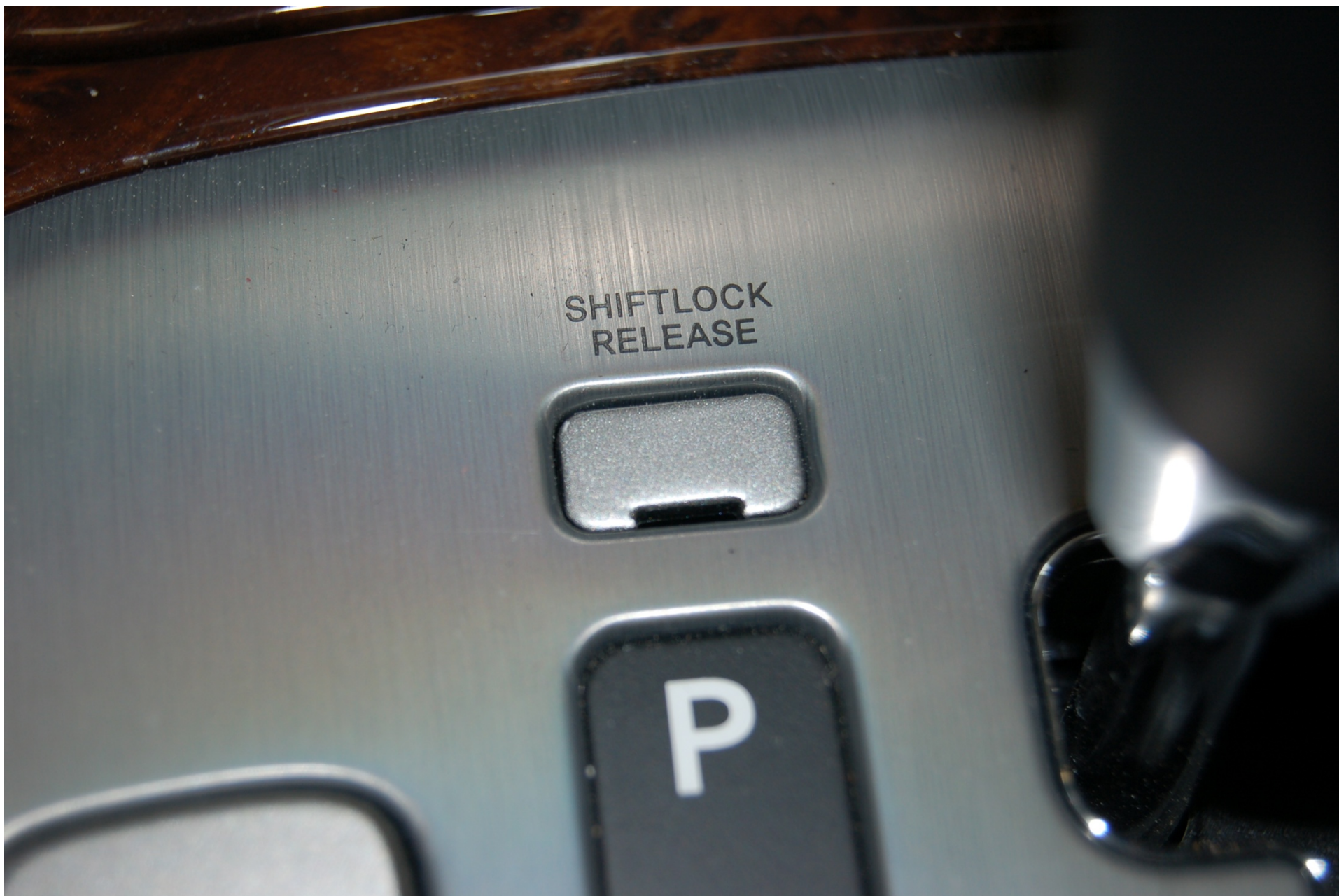
FIGURE 5.8 DEVICE WHICH ALLOWS MOVING GEAR SELECTOR OUT OF "PARK" POSITION
