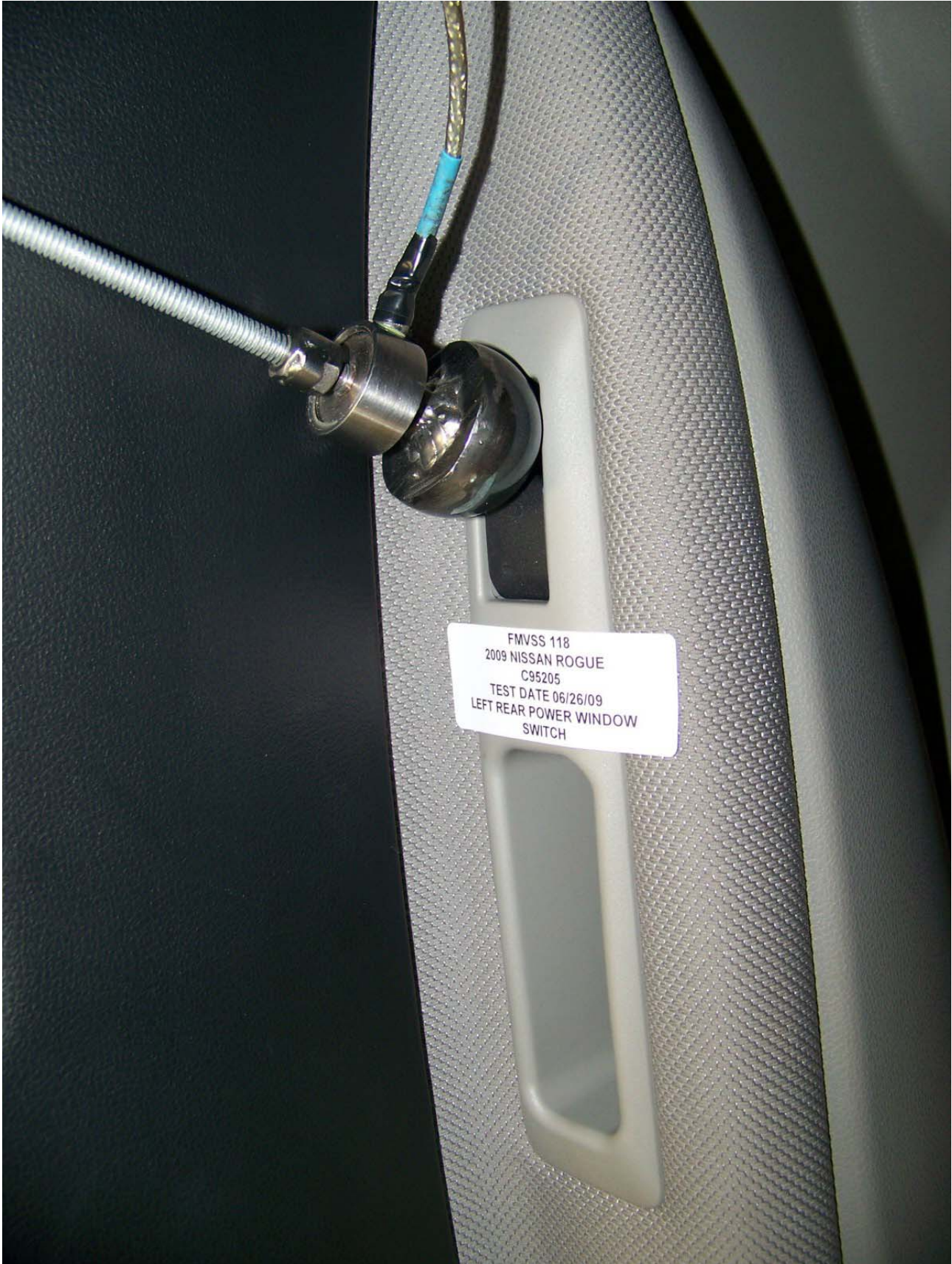
Figure 14: Sphere Test Left Rear Window
