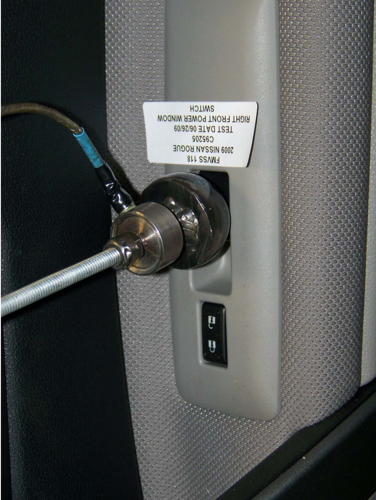
Figure 13: Sphere Test Right Front Window
