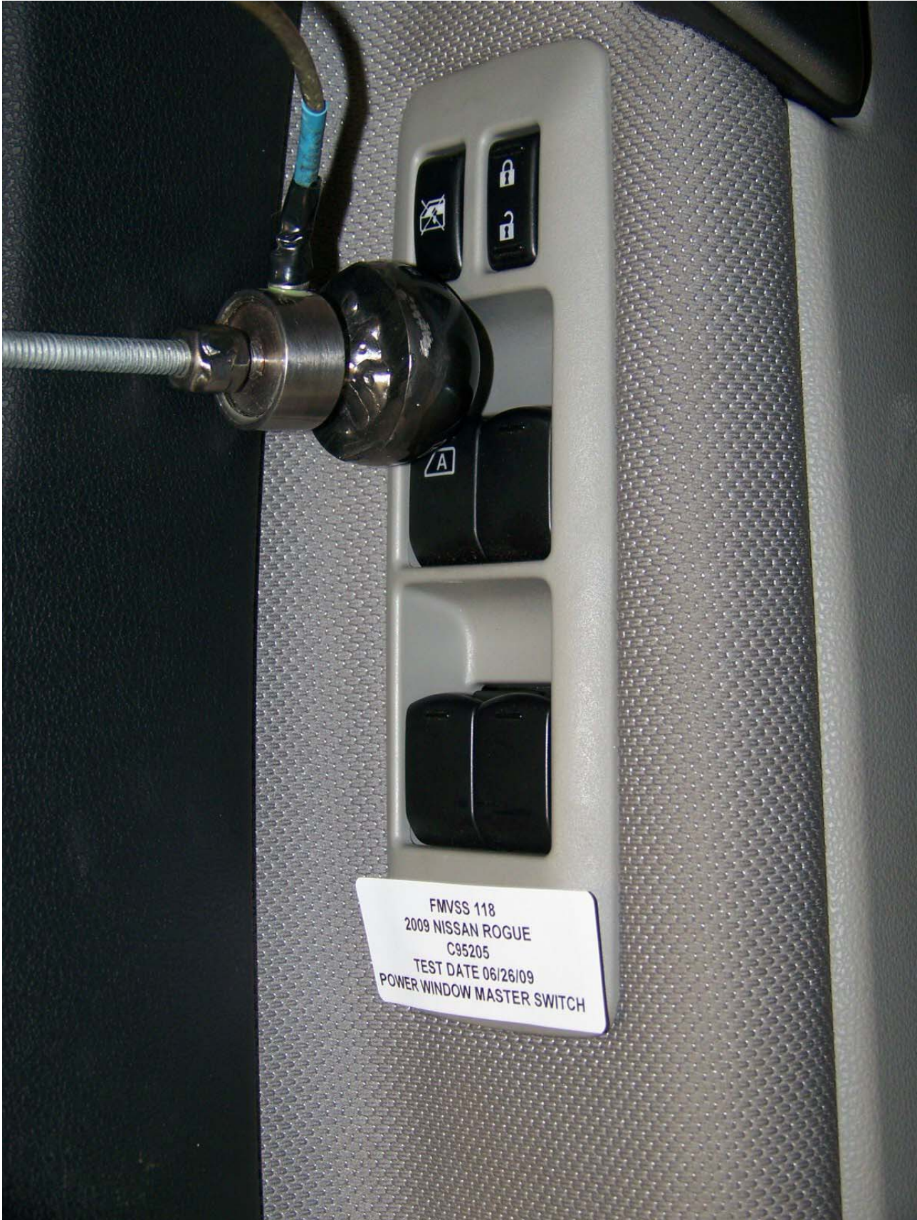
Figure 12: Sphere Test Master Control Panel
