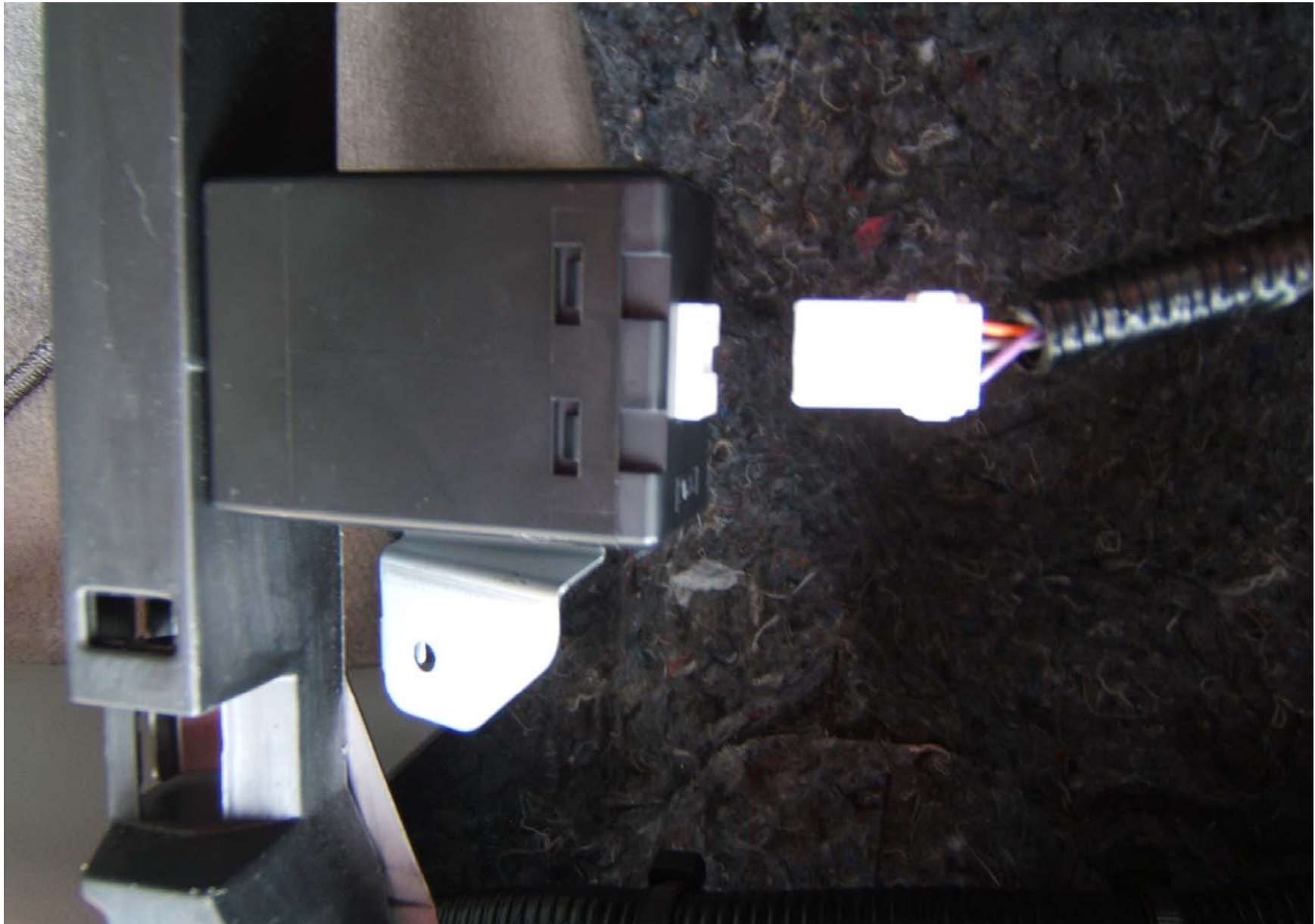
FIGURE 5.18 TPMS MODULE DISCONNECTED FOR MALFUNCTION DETECTION TEST
