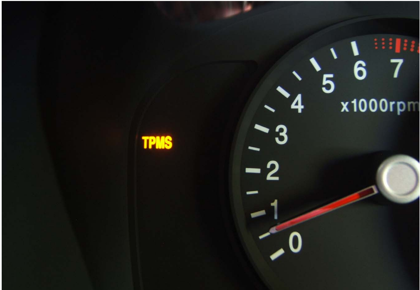
FIGURE 5.13 DISPLAY SHOWING DEDICATED TPMS MALFUNCTION WARNING TELLTALE
