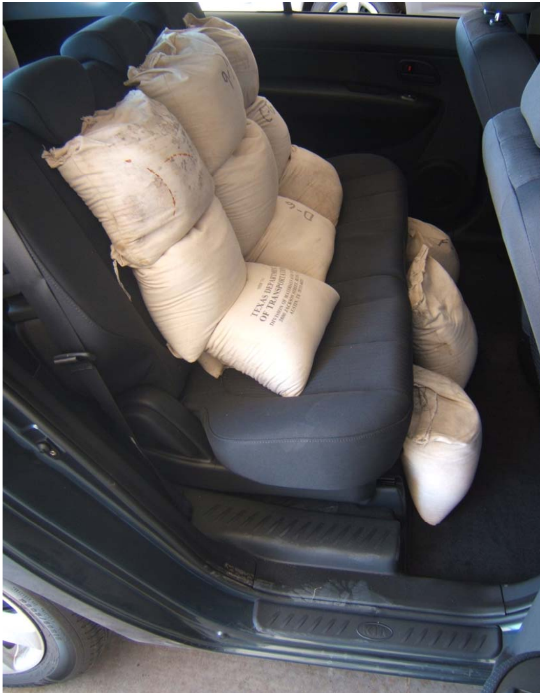
FIGURE 5.15 VEHICLE MID SEAT BALLAST FOR UVW + VCW LOAD
