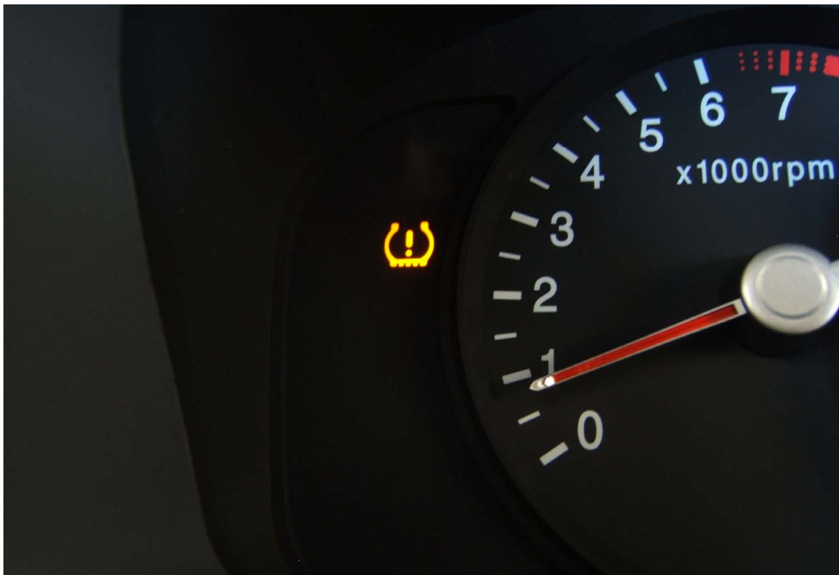
FIGURE 5.12 DISPLAY SHOWING LOW TIRE PRESSURE WARNING TELLTALE
