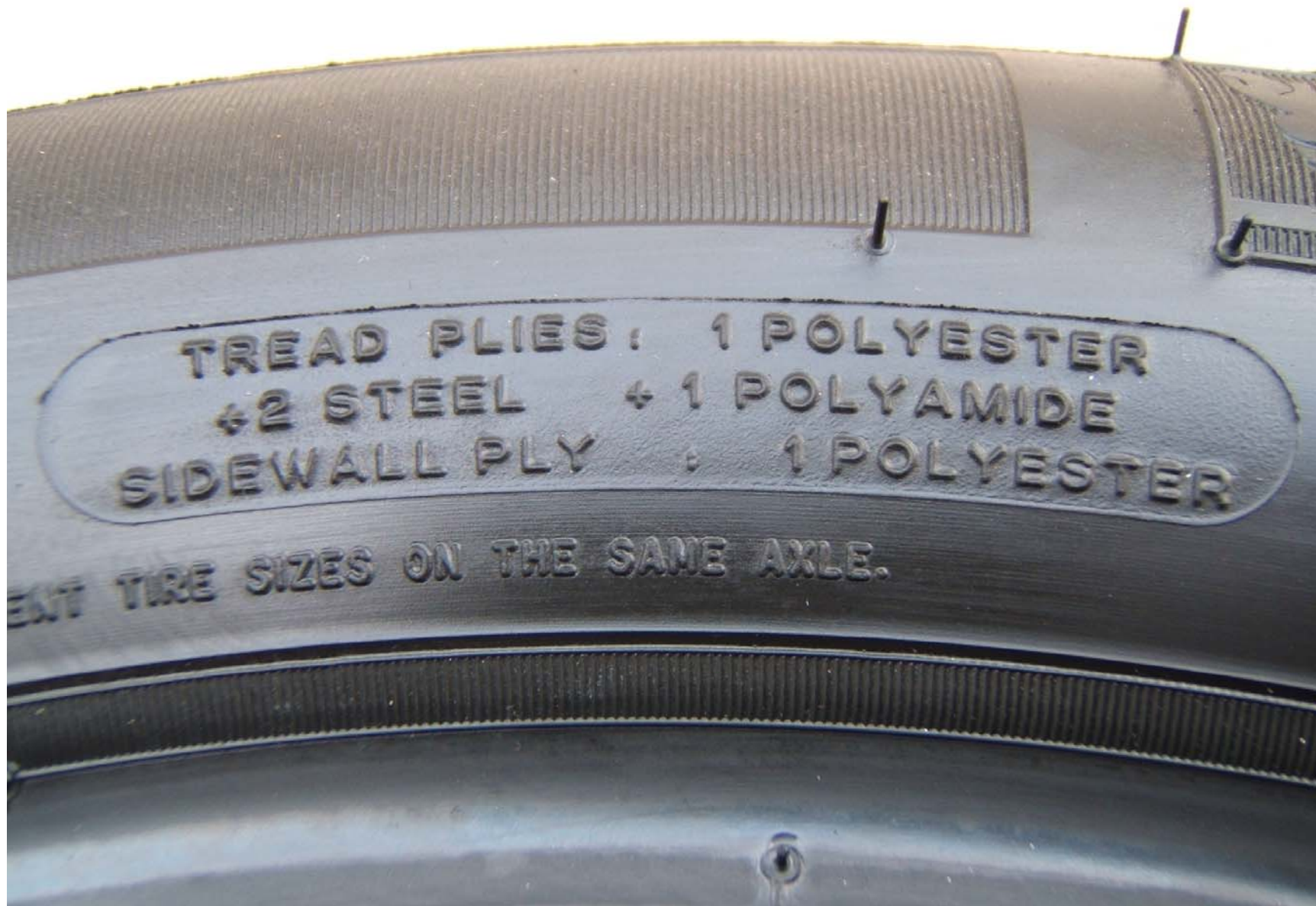
FIGURE 5.9 TIRE SHOWING SIDEWALL / TREAD CONSTRUCTION
