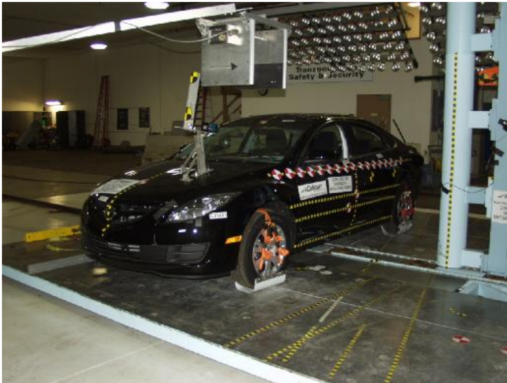
Figure A-21: Pre-Test Left Side View of Aligned Vehicle and Pole
