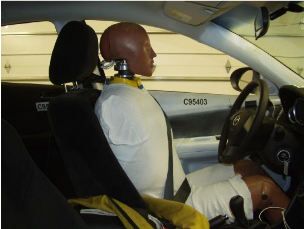
Figure A-27: Pre-Test Opposite Side View of SID HIII
