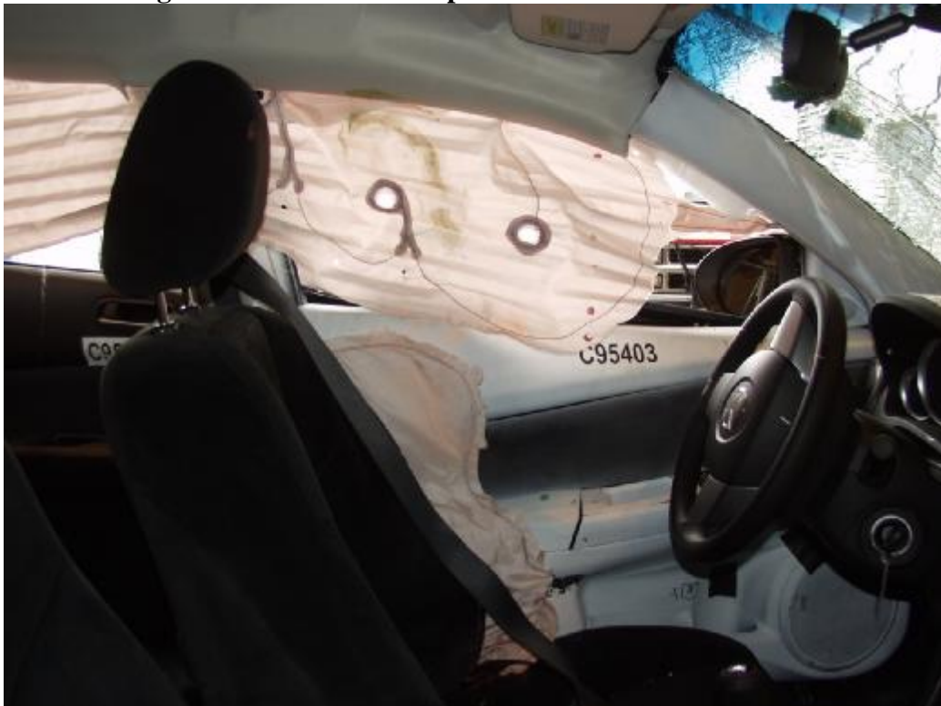
Figure A-35: Post-Test Impact Side Front Interior Trim
