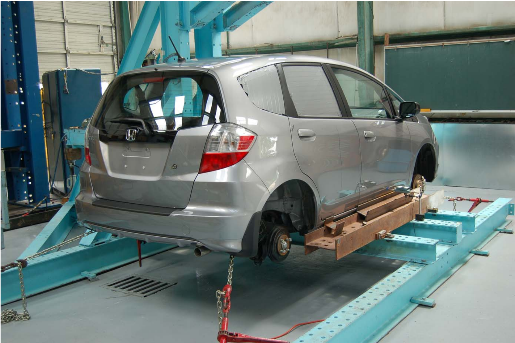
2009 HONDA FIT NHTSA NO. C95302 FMVSS NO. 214
