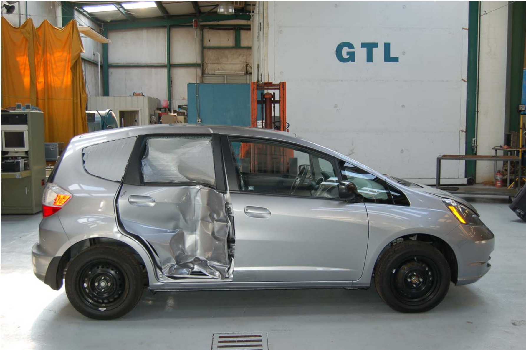
2009 HONDA FIT NHTSA NO. C95302 FMVSS NO. 214
