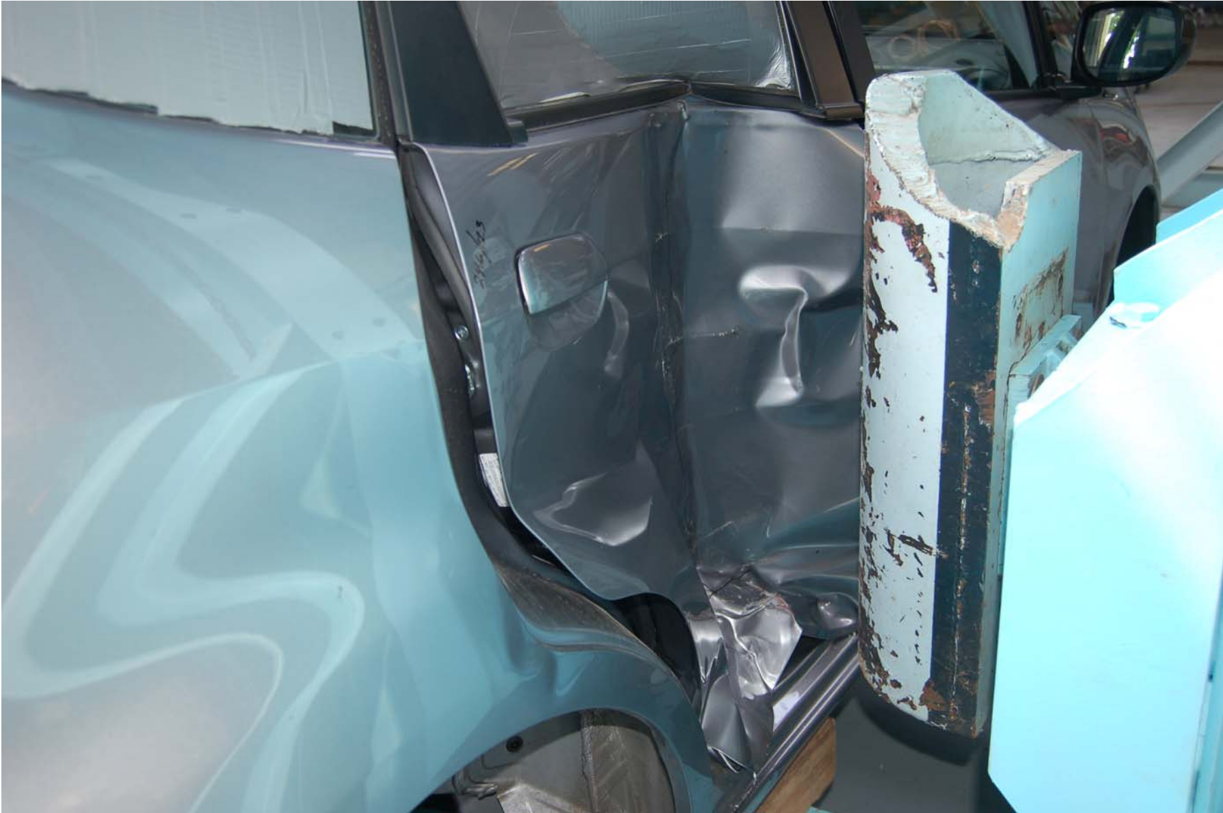
2009 HONDA FIT NHTSA NO. C95302 FMVSS NO. 214
