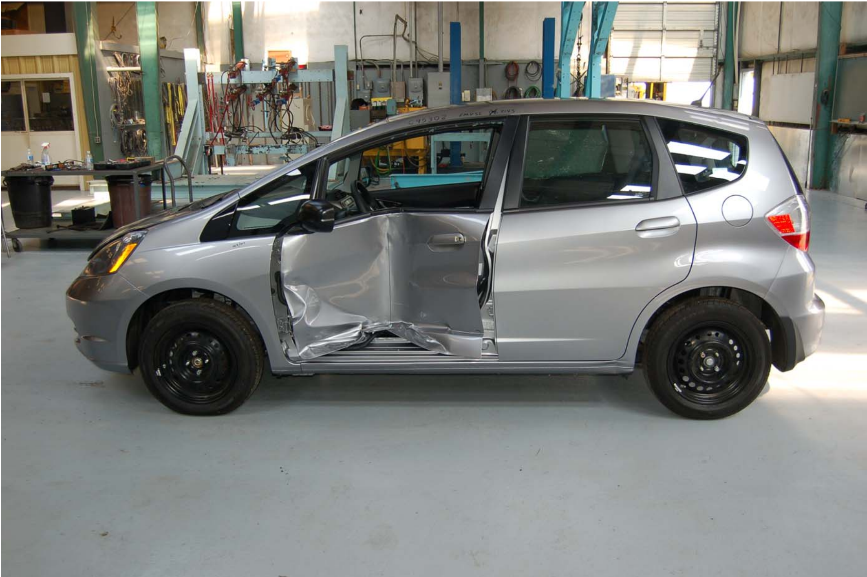
2009 HONDA FIT NHTSA NO. C95302 FMVSS NO. 214
