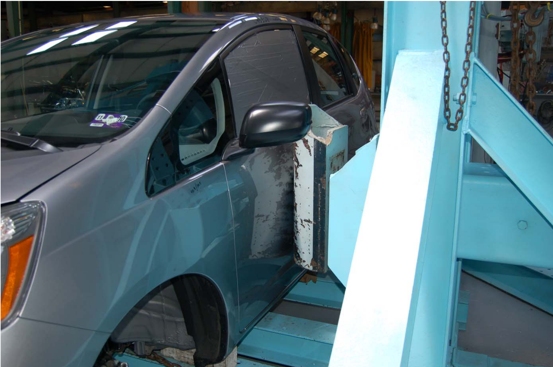
2009 HONDA FIT NHTSA NO. C95302 FMVSS NO. 214
