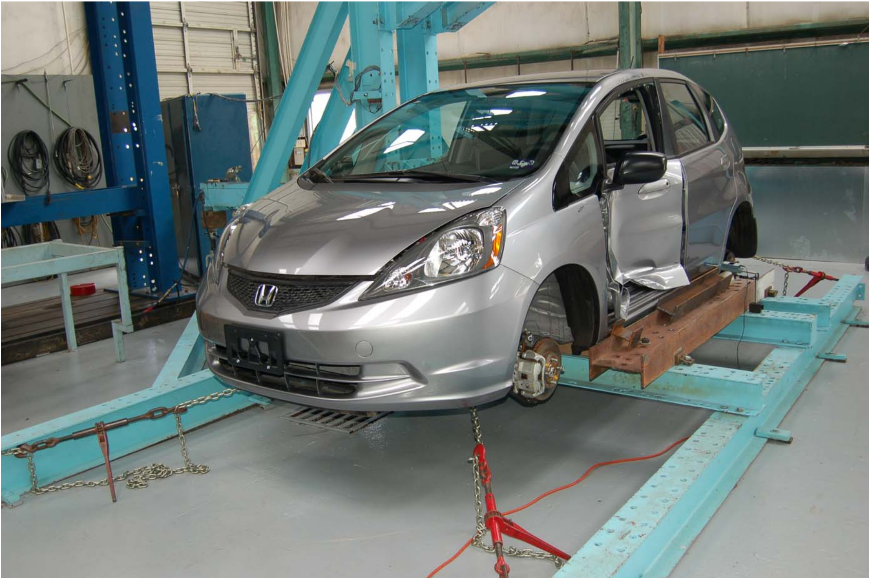
2009 HONDA FIT NHTSA NO. C95302 FMVSS NO. 214
