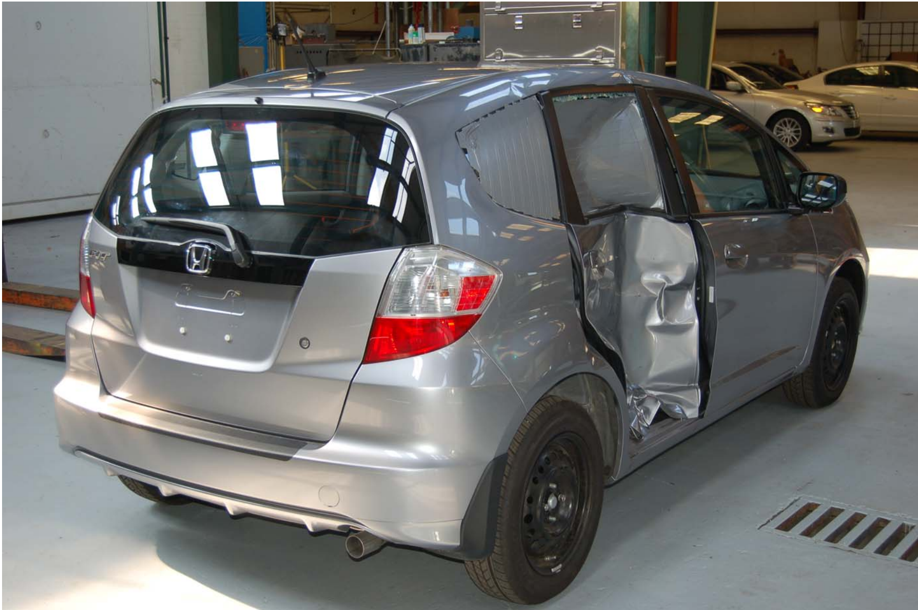
2009 HONDA FIT NHTSA NO. C95302 FMVSS NO. 214
