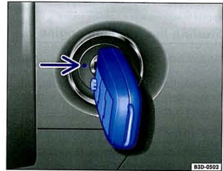
Fig. 3 Ignition lock: Emergency release button for the ignition key
